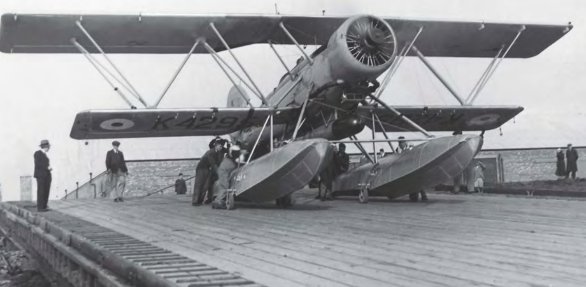
K4295 in floatplane configuration, running up its engine on the Brough slipway with dummy torpedo fitted. BAE SYSTEMS BROUGH HERITAGE
