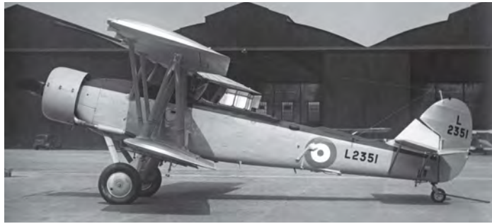
Factory-fresh Shark III L2351, from the final production batch. The main external difference on the MkIII was the enclosed canopy. This aircraft served at the School of Navy Co-operation from delivery in 1937, then going to the Fleet Air Arm pool, before being converted to a target tug in 1938 for service at No 2 AACU. BAE SYSTEMS BROUGH HERITAGE
