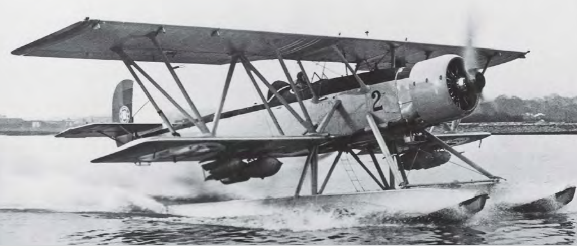
Portuguese Shark IIa serial 74, code 2, taxiing on the Humber. The load here is asymmetric, with three 250lb bombs under the port wing, and a 500lb and a smaller bomb to starboard. MATTHEW WILLIS COLLECTION
