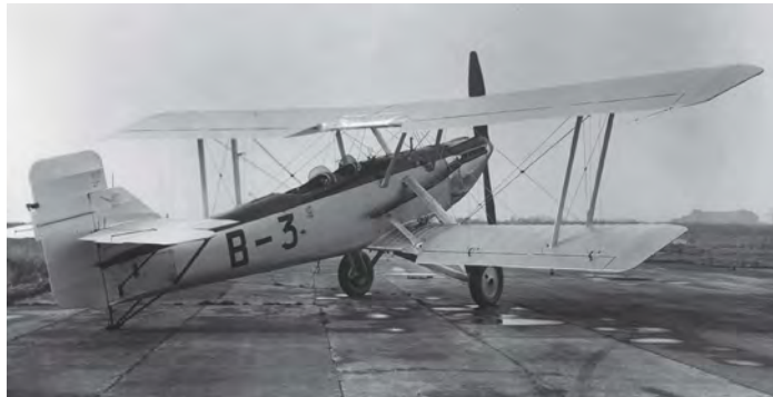
The second, revised Blackburn B-3, the true forerunner to the Shark. The aircraft was powered by a Rolls-Royce Buzzard and incorporated innovations such as a monocoque fuselage with a 'wet' section containing the fuel. BAE SYSTEMS BROUGH HERITAGE
