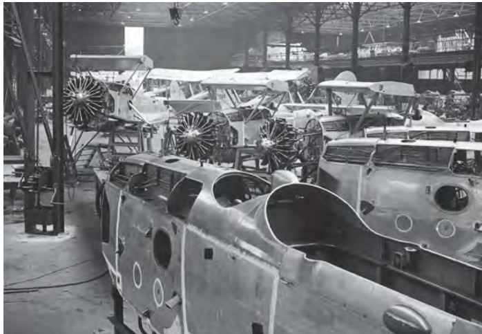
ABOVE: Shark fuselages from the initial batch of MkI airframes nearing completion at Brough in 1935 — K4354 was the sixth production Shark and K4356 the eighth. Note the sealant applied to the panel joins to help render the monocoque fuselage watertight. The aircraft to the right rear are Baffins, the Shark's predecessors, which were still being delivered. AEROPLANE
