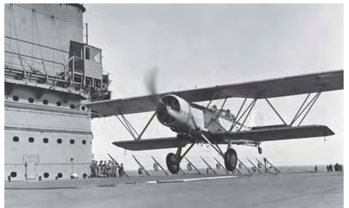
The B-6 taking off from HMS Courageous during the aircraft's carrier trials in 1934, still fitted with the short-chord cowling.
