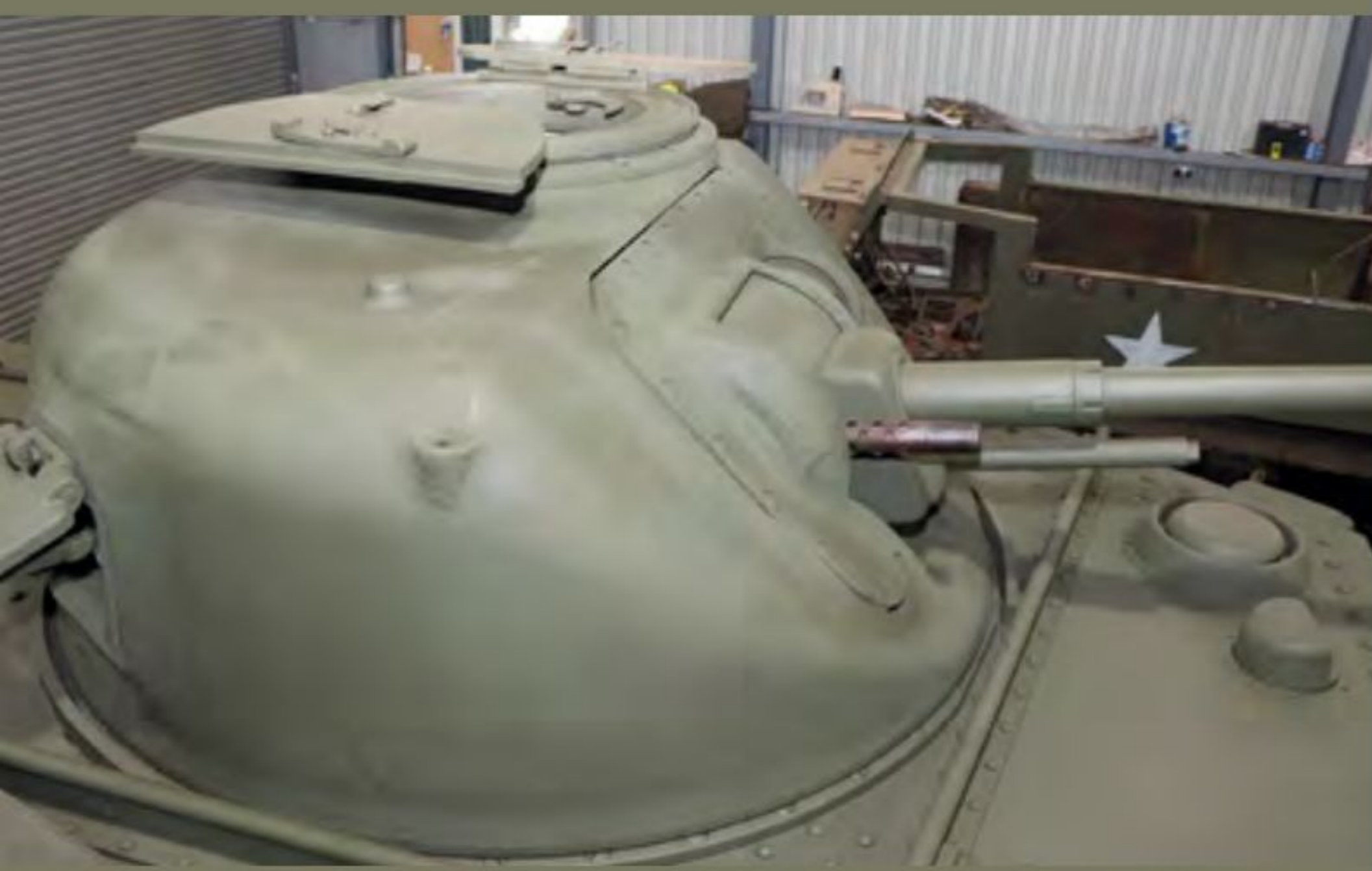
The turret with its 37mm and machine gun
