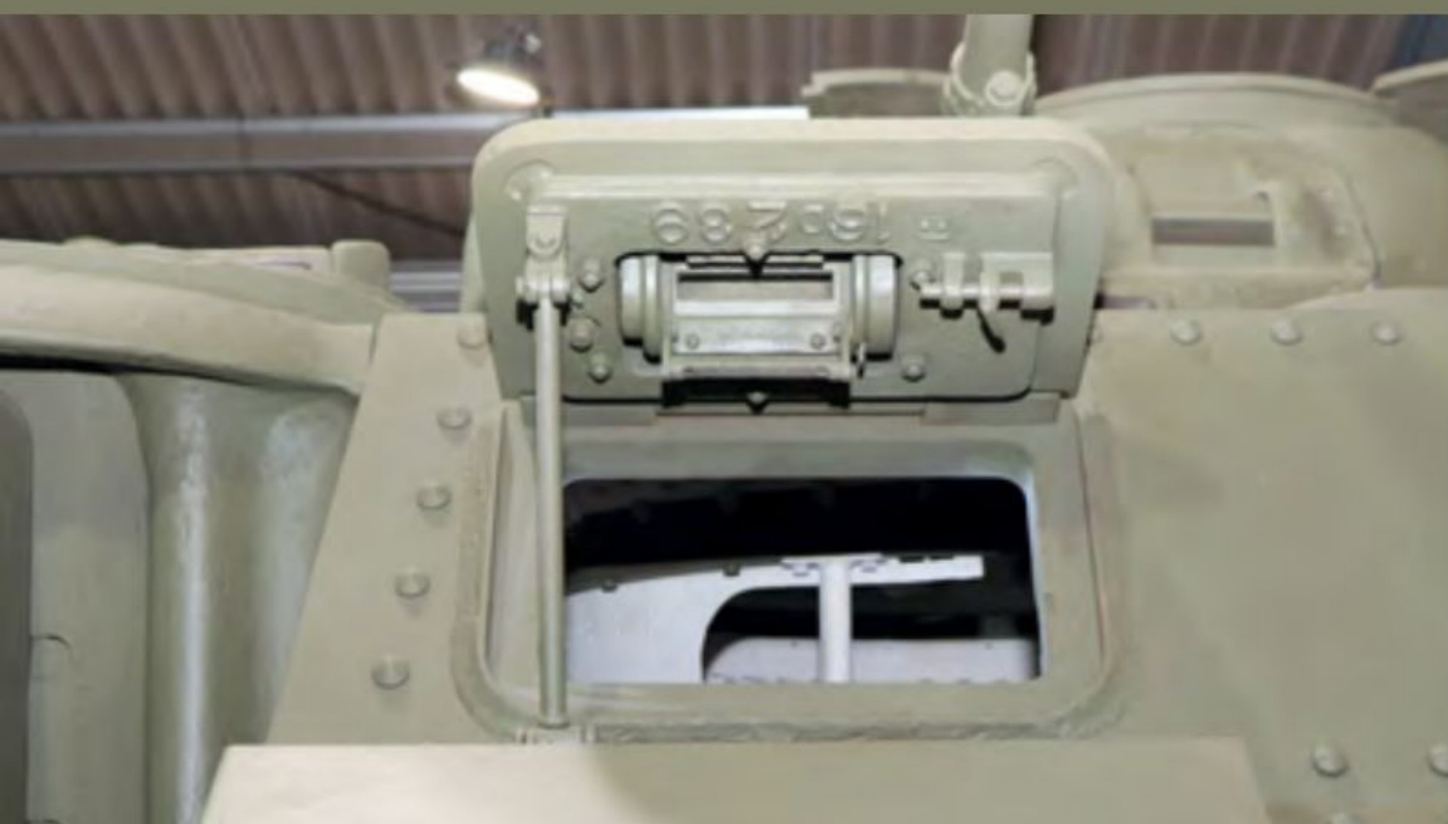
The driver's hatch located in the middle of the tank
