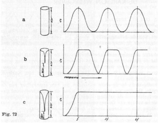
If an exponential slot is made at the open end of the pipe then the air column no longer has a specific length, resulting in the sharp peaks and dips being smoothed.
