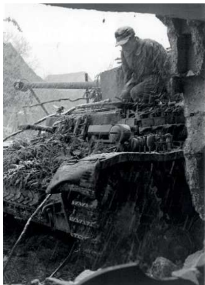
■ Right: GIs examine a destroyed Panzer IV Ausf. J. Against side hits, the 30mm armour could not withstand any Allied tank gun.
