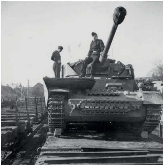
■ During rail transport the side skirts were usually removed. This Panzer IV (H or J) seems to be carrying a spare set.
