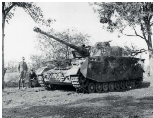
■ A Panzer IV Ausf. J. Mesh side skirts were introduced in September 1944. Just like those made of solid armour plate they were offering protection against heavy Russian AT-rifles.
