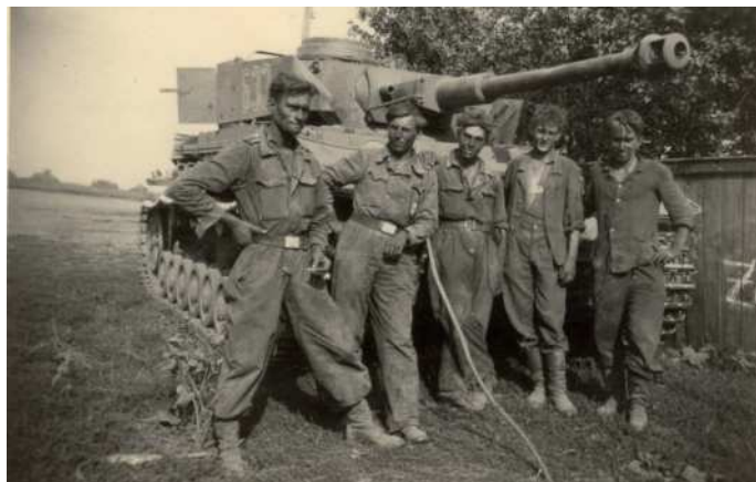
■ The strain of the fighting is visible in the faces of the crew of a Panzer IV Ausf.G. The fittings of the armoured skirts were not very sturdy and as such they were often lost. Yet in stark contrast to assault gun units, the Panzer-Abteilungen never introduced any sturdier, self-built solutions. The reasons for that are unknown.
