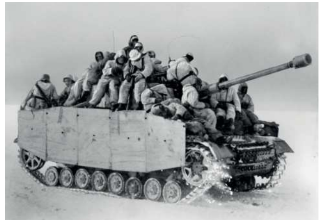
■ It is not commonly known that in 1943 the Nibelungenwerke developed a way to increase the ground clearance of the Panzer IV by fitting spacers between the hull and bogie assembly. The spacer set could easily be installed to lift the 'stilted chassis' by about 15 centimeters but was never used in large numbers.
