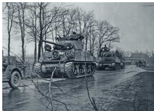
■ The 76 mm armed Sherman M4 was introduced by autumn 1944. This crew have added extra 'armour' - track links and road wheels.
