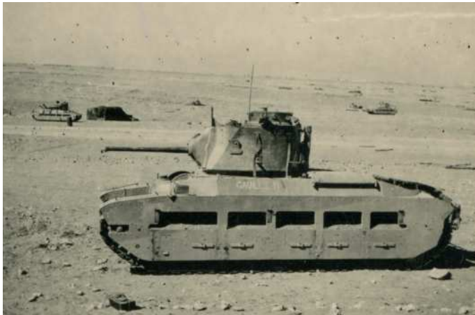
■ The British Mk.II Matilda II was a serious opponent for any German tank and it often took the support of 8.8 cm Flak to cope with the heavily armoured threat.
