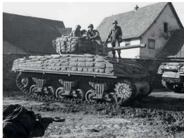
■ A US Sherman tank at the Steinbourg in France close to the German border. The layer of 'extra armour' consisting of sacks of sand was to some extent effective against Panzerfaust and Panzerschreck projectiles but offered no protection against the PzGr 39 or 40 fired by the Panzer IV.
