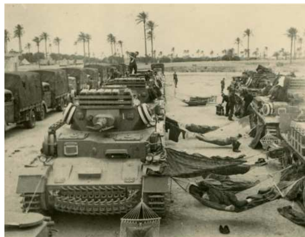
■ Panzer IV Ausf.E of Pz.Reg.8 after landing at Tripoli. Openings still sealed against seawater and rubber coverings protected against heat with white paint.
