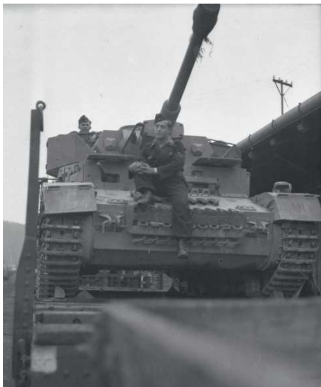
■ A limited number of older tanks were modernised during general maintenance. This Ausf.E had already received additional armour when a 7.5 cm KwK 40 L/43 and armour skirts around the turret were fitted during a repair.
