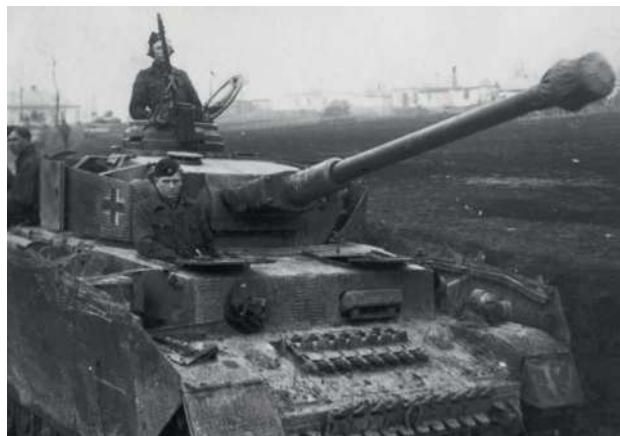
■ A mysterious photo showing a Panzer IV, probably an Ausf.H, which has been coated with an atypical coat of Zimmerit, probably as a trial. It mounts a Fliegerbeschussgerät 43. The name ‘York’ has been written on the barrel jacket.
