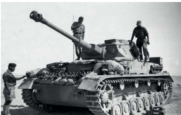
■ In Africa the Panzer IV G with its long KwK40 could engage and destroy any Allied tank on ranges between 1,500 and 2,000 metres, outside the effective range of their opponents guns.
