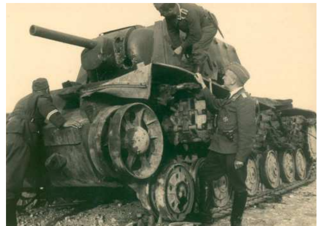
■ During the early part of Operation Barbarossa in 1941, German tankers found the heavy KV-1 a near invincible opponent. This example was stopped by a hit on the idler wheel which ruptured the track.
