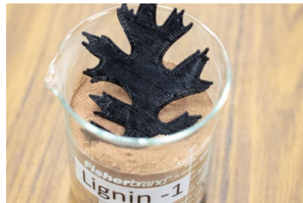
Figure 38: Lignin sample and 3D-printed part composed of lignin-nylon-carbon fiber composite filament in beaker
