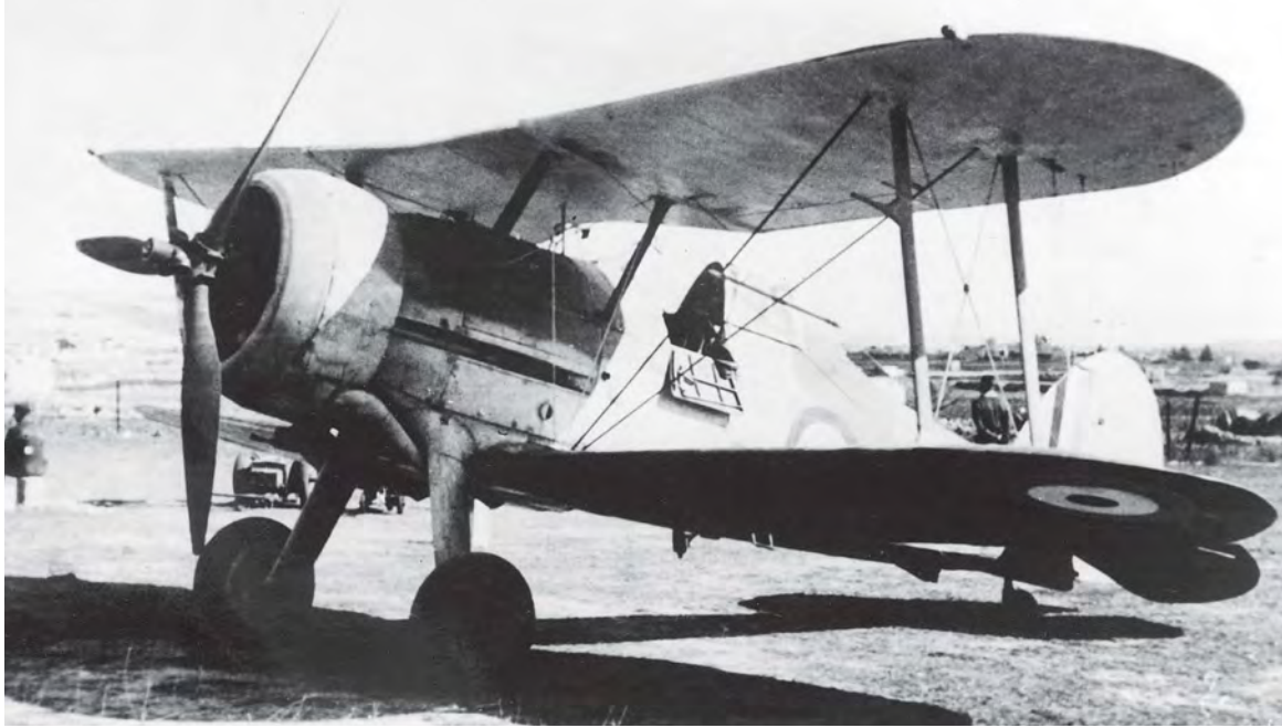
LEFT: The last RAF Sea Gladiator claims over Malta were made on 2 November 1940 by Flt Lt Burges. He was in N5520, which had earlier been fitted with a Mercury VIII engine and Hamilton propeller from a crashed Blenheim. NWMAVIA B. CULL
