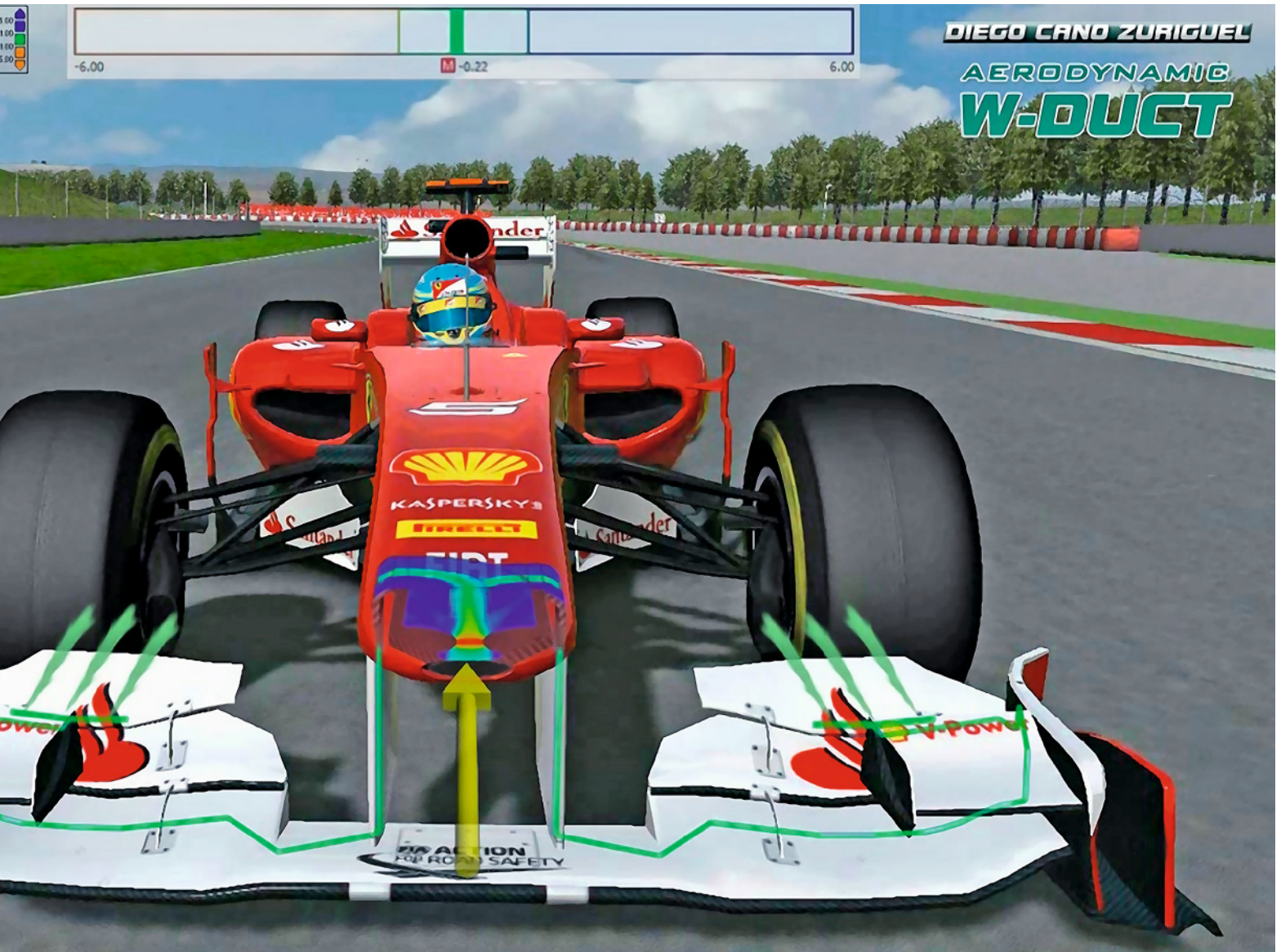
Gap between elements keeps flow attached
