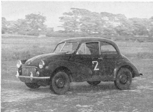
★ SOUPED UP, NOT SAT UPON: (Left) Andy Hutchinson's Morris Minor has an odd-looking bonnet, but it hides a lusty 1,250 c.c. M.G. engine which helped him to win the saloon car handicap at Cranfield. ★
