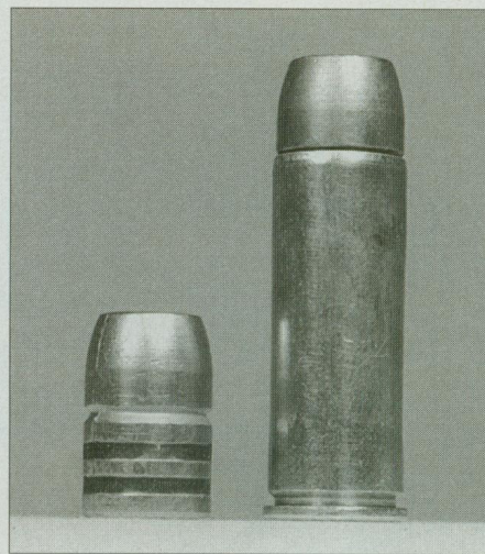
The author's load for his new revolver uses a 300-grain LBT wide flatnose bullet and 23 grains of H-110 powder. It is exceptionally accurate and hits very hard.
