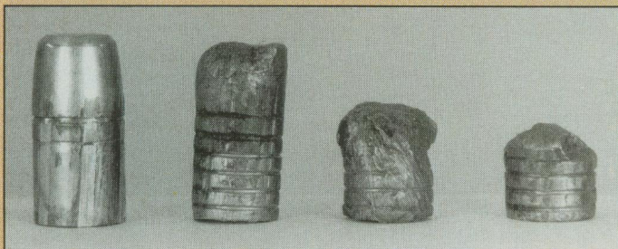
The above bullets were recovered from game on the hunt: 385-gr. Sledge Hammer from bull, 430-grain solid from buffalo, and bases of two soft noses after expanding.
