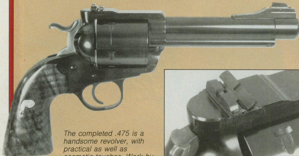
Three photos show the versatile custom sights on Seyfried's .475. Top: Front sight adjusts for elevation. Above: A barrel band is also a shoulder for the extractor rod. Left: Two rear blades.
