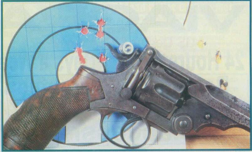
The "group" on the right shows the keyholes, while the one on the left demonstrates fine accuracy after drilling the hollow bases in the bullets allowing them to fit the ill dimensions of the .476 revolver.
