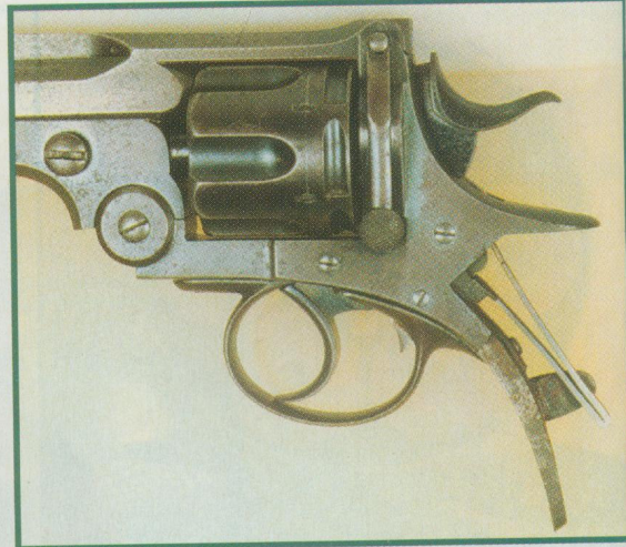
The Webley revolver features a typical British V mainspring and a magnificent double-action pull.
