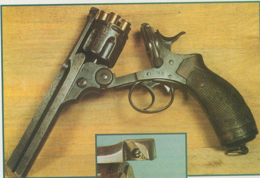
The Webley revolver features a typical British V mainspring and a magnificent double-action pull.
