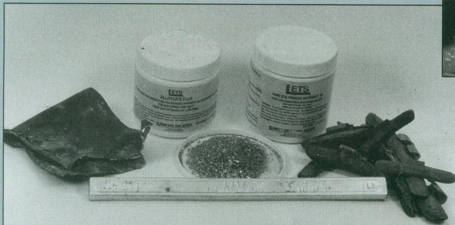
Flux helps remove impurities. Powdered antimony and special flux for mixing it with your lead are available (below).
