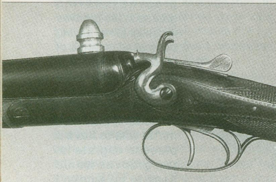
This is an original Holland & Holland Paradox gun shown along with an original bullet in the unusual configuration to allow it to successfully pass through the rifled choke.
