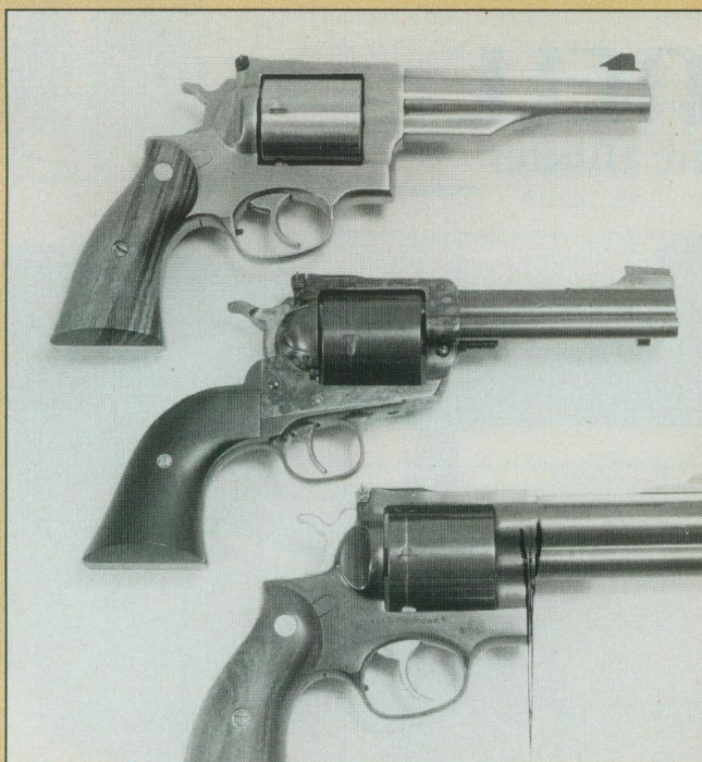
Bowen conversions to 5-shot big-bores at left. Top: Redhawk rebored w/new cylinder. Center: Blackhawk with ovate barrel. Bottom: Redhawk "L" barrel. Below: 300-gr. Freedom Arms JFP (left) shown with 325-gr. NEI long flat-nose bullet.
