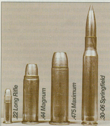
Rounds used in the fire-lapping tests included this lineup of centerfire handgun and rifle cartridges, along with the .22 rimfire. Any firearms barrel will respond well to the lapping process, regardless of type.
