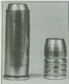
This is the .44 Magnum lapping round and its bullet. Note that the bullet is seated very deeply in the case to control the lapping compound and to decrease case capacity for reliable powder ignition.
