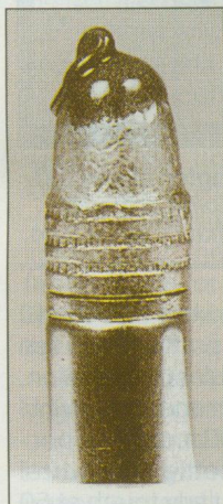
To fire-lap the bore of a .22 rimfire arm, the LBT lapping compound is applied directly to the tip of the bullet, like whipped cream on a sundae!
