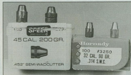
Soft swaged-lead handgun bullets can be used to slug barrels to determine interior measurements. Use the next larger caliber size (i.e., .45 in .44, .32 in .30) for correct results.
