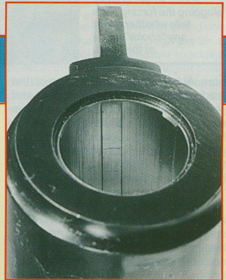
This is the muzzle view of the author's .475 Maximum revolver after fire-lapping, showing the smooth, even finish achieved.
