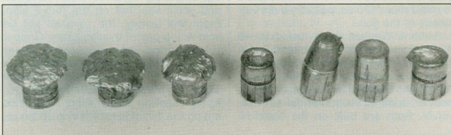
The 3 cast soft nose slugs at left gave better expansion than jacketed soft nose bullets in wet newspaper.
