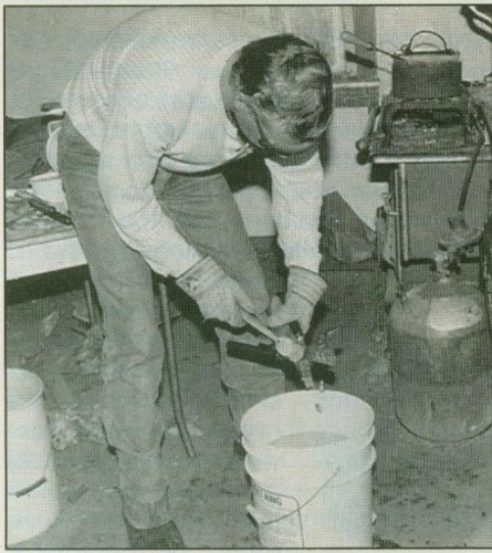
Dropping the hot bullets directly from the mould into a bucket of water will heat-treat the bases for extra hardness.
