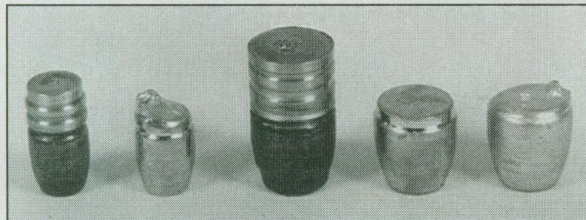
Nose sections cast using standard moulds are not as perfect as noses from the LBT mould (second from left), but accuracy is good.
