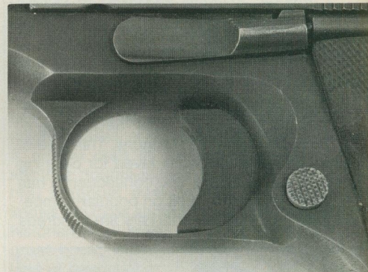
A standard G.I. trigger is hard for many shooters to use. An extended trigger like this one is more comfortable.
