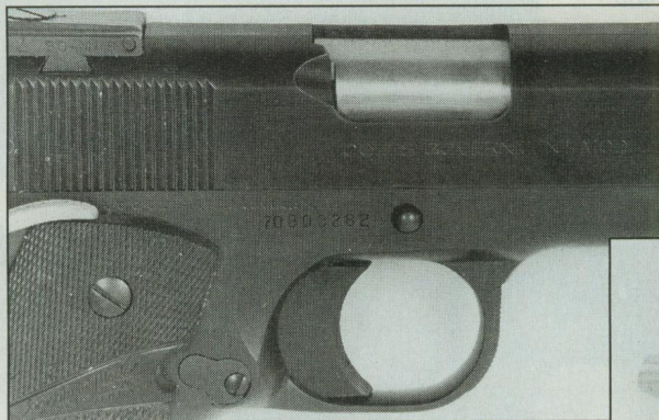
A lowered ejection port is a big aid to reliability. It also helps keep the fired cases in better shape for reloading—there are no dents in the case mouth.
