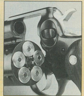
Because of the size of these .577 rounds, Bowen's creation, like the 19th-century revolvers, employed five-shot cylinders.
