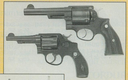
Gunmaker Hamilton Bowen created his own .577 DA revolver by starting with a Ruger Redhawk revolver, then using a Labounty barrel and Bowen's own five-shot cylinder. Dubbed the .577 No. 2, this modern-day equivalent of Seyfried's 19th-century .577 Bland is shown here with an S&W M&P in .38 Special. Inset shows difference in bore sizes.
