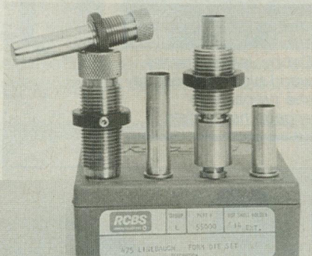
Above: RCBS case forming die set for the .475 Linebaugh. From left is expander die, file trim die, extended shellholder. Left: Steps in making cases shows sequence of forming.
