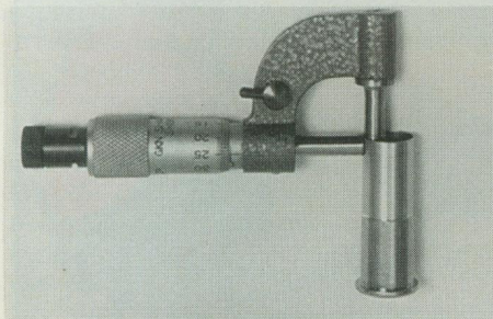
After lathe turning, a tubing micrometer is used to check case wall thickness. Here, .25mm or .010" is ideal for .475.
