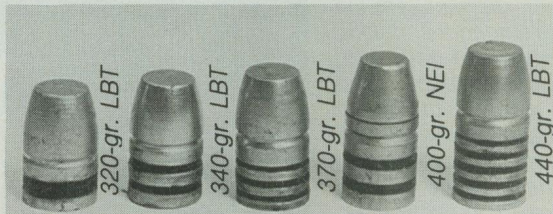
Above: Steps taken by author to form .475 ammo from .45-70 cases. Larger chambers and RCBS form die set make this easier. Left: .475 bullets: 320-gr. LBT, 340-gr. LBT, 370-gr. LBT, 400-gr. NEI and 440-gr. LBT.
