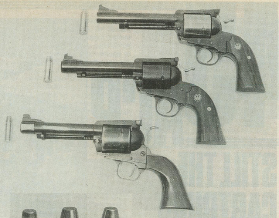
Above: Author's trio of "super magnums." Top to bottom: the .500, .475, and .45 Colt Linebaugh revolvers. .475 and .500 use Ruger Bisley frames. .45 Colt is made on Seville frame. All exhibit superior finish. Left: .45 Colt, .475 Linebaugh, .500 Linebaugh.
