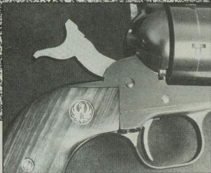
The engine-turned machinework on this .45 Colt caliber Ruger's hammer and trigger is evidence of quality work, even on a basic action job.
