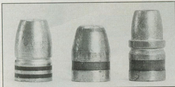
Pressure tests were made using the three bullets seen above, which include from left to right a truncated radius, truncated cone and SWC.
