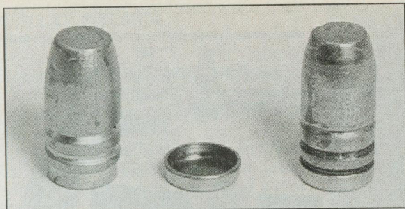
Gas checks, fitted to the base of cast bullets, are not the harmful appendages we were once told, and in many cases make a good bullet better.
