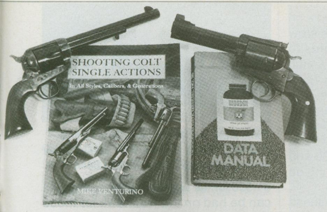
Two sources of loading data and their respective guns: Venturino's Shooting Colt Single Actions and EMF Hartford function at the blackpowder level, while Hodgdon's manual offers data compatible with the Ruger Bisley.
