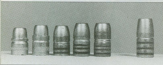
Selection of .45 cast bullets: 260-grain Keith, 310-grain Keith, 325-grain LFN/LBT, 350-grain LFN/LBT, 360-grain WFN/LBT. Bullet far right is a 412-grain WLN/LBT. This bullet is generally too heavy for best results.
