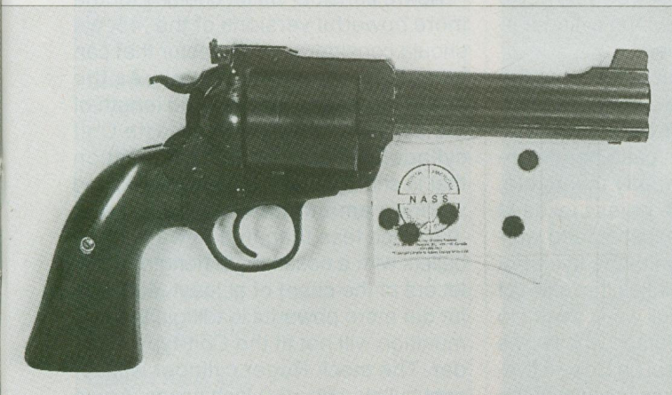
This Clements five-shot Ruger Bisley conversion is shown with a target shot at 50 yards using full-power 360-grain WFN bullets.
