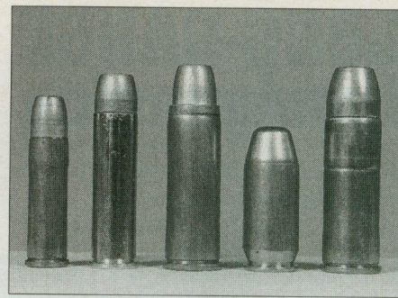
Long-range shooting can be done with just about any cartridge. From left: The .32 Mag. and .357 Mag. are a bit light, while the .44 Mag. is optimum. The .45 ACP's low velocity keeps it from being a top performer, though the .45 Colt is right up there with the .44 Mag.
