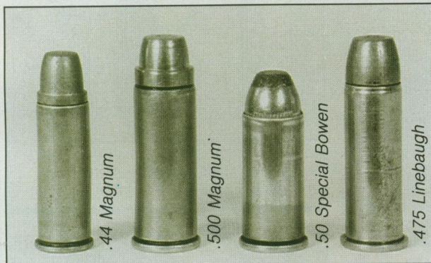
Here are some special Wildcats, tailored for use with custom handguns. The cartridge on the left is the familiar .44 Magnum, shown for contrast. Others are: .500 Magnum, .50 Special Bowen, .475 Linebaugh.
