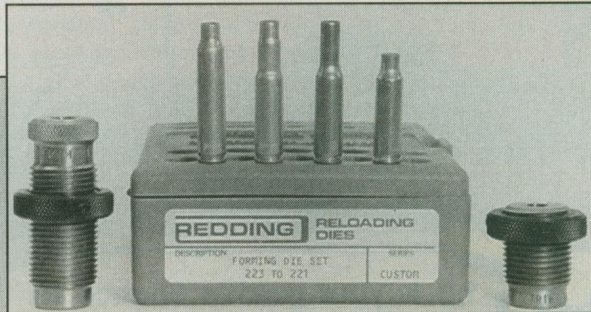
Economy-minded reloaders can use this form die set from Redding, making .221 Fireball from .223—for a penny each.
