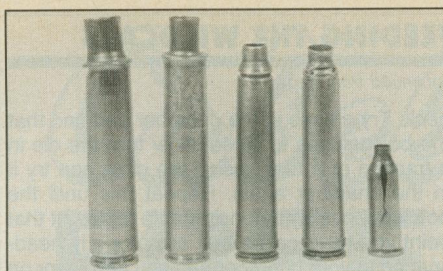
Case forming gone wrong. Wrinkled necks, collapsed shoulders and split cases are part of the game.
