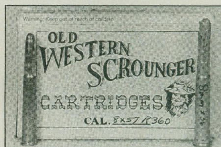
The chamber cast on the right was the only way to identify an unknown wildcat, for which ammo was made.
