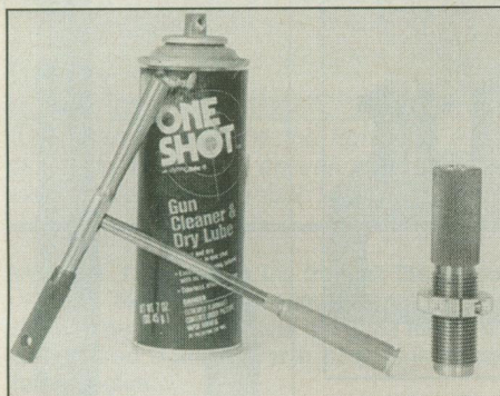
RCBS neck ream die will reduce neck thickness with great precision. Use a good lube like Hornady's One-Shot.
