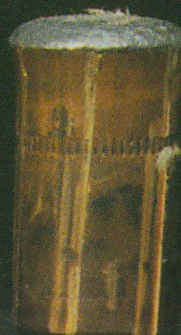
.475 430-gr. DWR softnose (recovered from wet paper)
