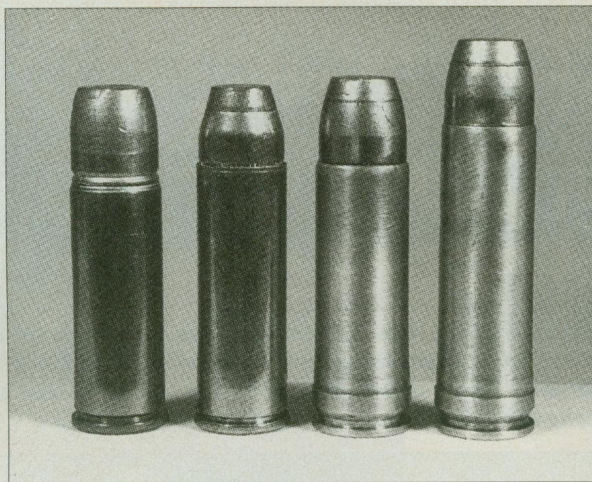
From left: .45 Colt, .454 Casull, .458 1.4-inch, .458 1.6-inch. While the .45 Colt remains the most practical cartridge, the belted magnum rounds demonstrate the ultimate in ballistic performance from the .45 bore, easily outdistancing even the .454.
