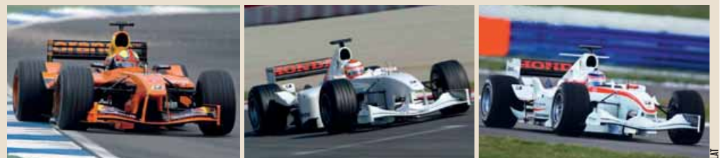
Super Aguri's re-worked Arrows chassis made its competition debut at the Bahrain Grand Prix. Initially the test car appeared with 2002-spec aerodynamics (centre) then with an update kit for the Bahrain Grand Prix (right). The car has evolved from the Sergio Rinland-designed A23 of 2002 (left). The arrival of the all new Aguri has been delayed.
