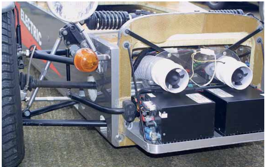
Above: twin controllers at the front look after the pair of fan-cooled front motors. Driveshaft to the driver's side front wheel is also visible
