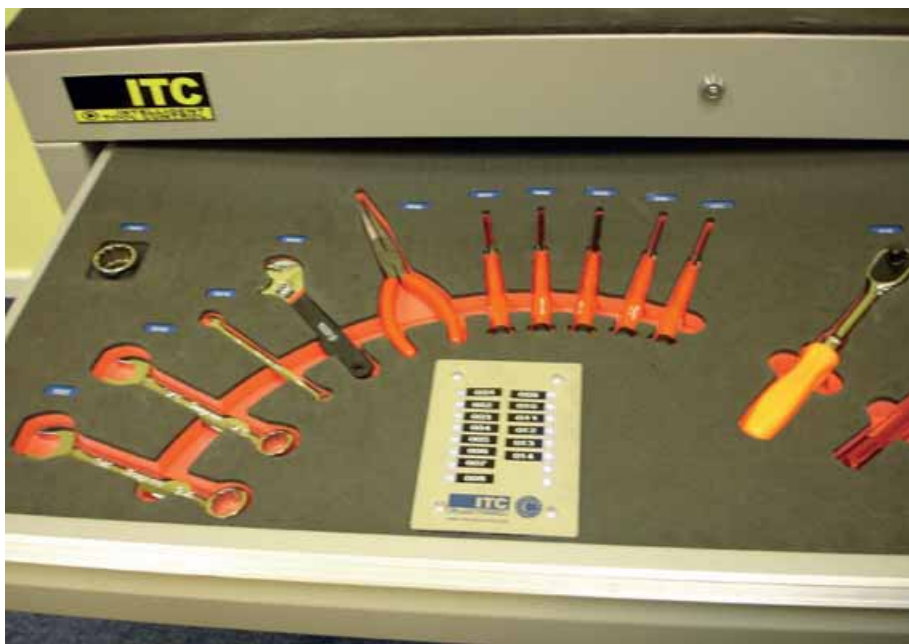
Optican sensors were chosen for the tracking devices while PIN codes and swipe cards control access
