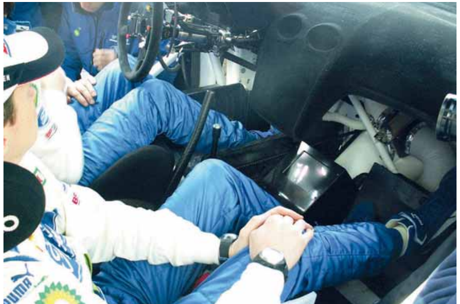
M-Sports designers have situated as much equipment as possible on the floor of the car to lower the centre of gravity, including the crew. Note mechanical and semi automatic shifters
