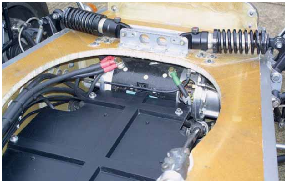
Above: the front motor pack resides ahead of the batteries, and drives out to the front wheels
