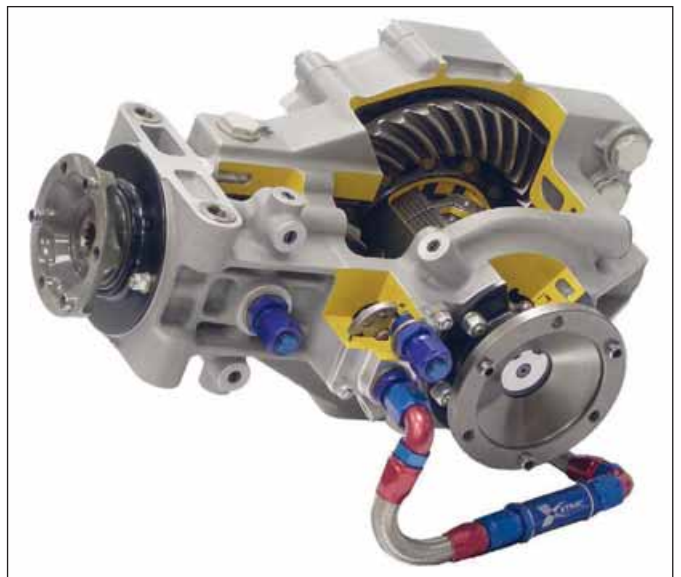
Viscous effect adds control to a plate-type diff in a viscous combined plate unit. Xtrac 247 heavy-duty unit is an adjustable plate diff, also available with viscous
