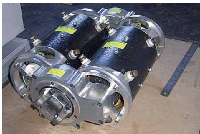
Above: the front motor pack resides ahead of the batteries, and drives out to the front wheels
