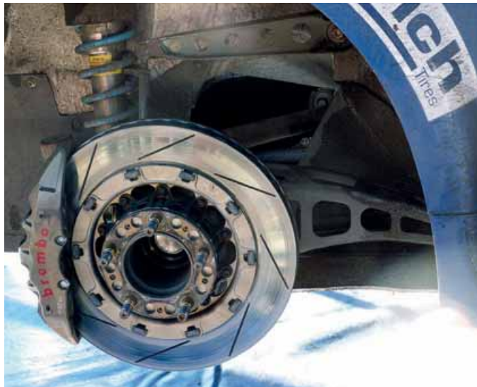
Brembo ventilated discs and eight piston calipers provide stopping power on asphalt and four piston units on gravel. Note Reiger remote reservoir shocks and McPherson strut arrangement
