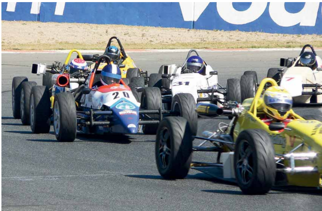
Formula Vee racing has always been close and action packed and British spectators regularly claim that Vees are the most entertaining formula of all to watch. Here, cars in the South African series battle for position. These cars do not use the Beetle's air-cooled engine, instead water-cooled, 1400cc VW units are fitted.
