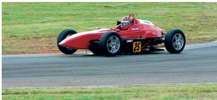
Many Vee manufacturers employ high noses and a splitter to try and create an aerodynamic gain, though little wind tunnel research has been done to justify this. Pictured is a South African-built Lantis chassis
