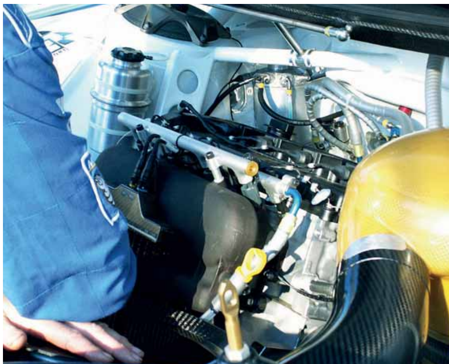
The engine bay was originally designed for the road going Focus ST220's 2.5-litre Volvo five-cylinder unit
