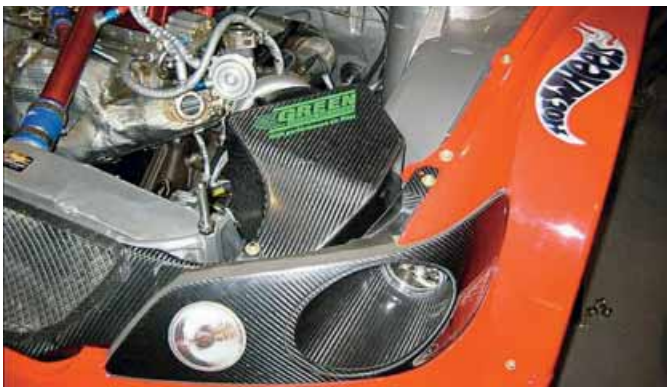
Green filters are currently used on all WRCs, except Citroën. Here a Mitsubishi
