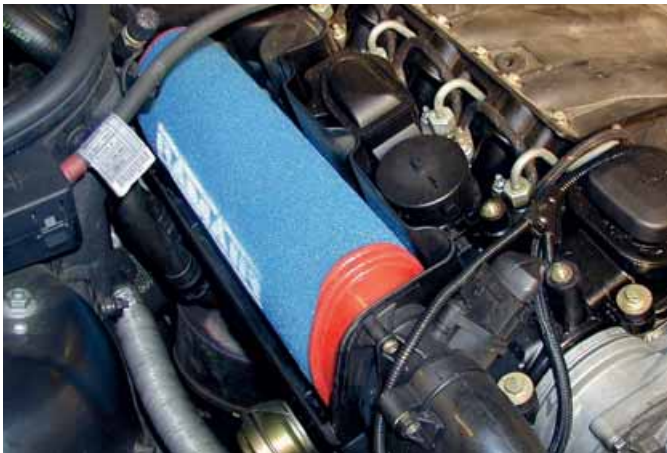
Ramair offers filters with up to five different stages of filtration and with either open or closed cell foam, the latter said to be particularly effective in dirty air
