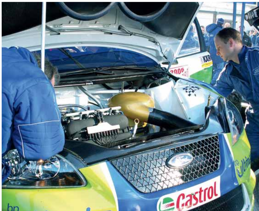
2006 Focus WRC's engine is based on the Mazda Duratec in-line four and is prepared by Pipo in France
