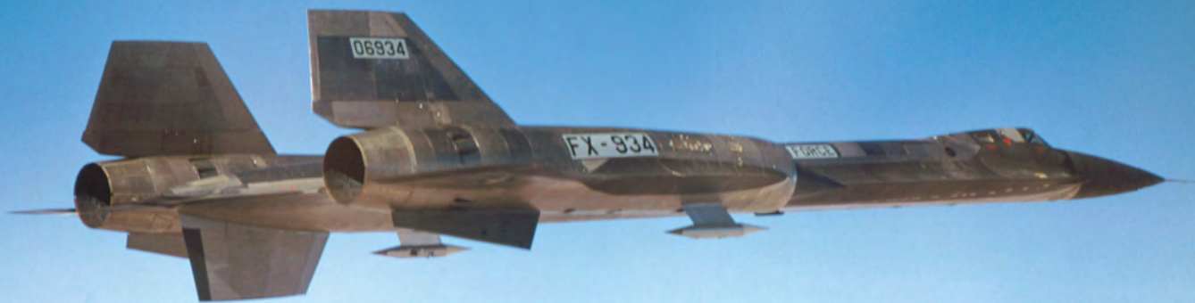
Prototype article 1001, serial 60-6934 with its centreline folding ventral fin extended to improve longitudinal stability. This picture was taken early on in its test flight career, before it was given an overall black colour scheme to reduce the effects of thermodynamic heating encountered at its design cruise speed of Mach 3.2. Lockheed Martin
