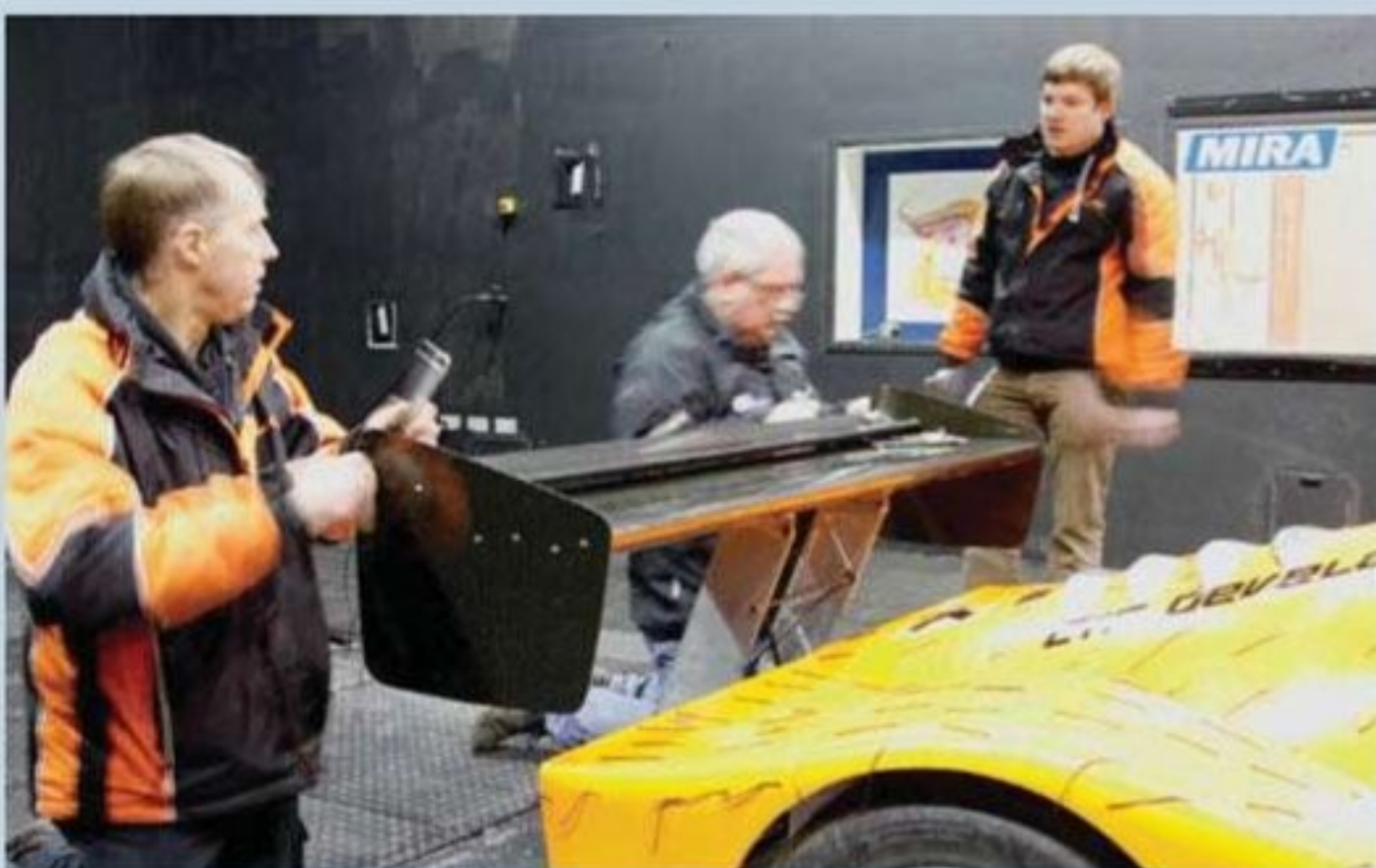
Dropping the rear flap angle shifted yet more balance
