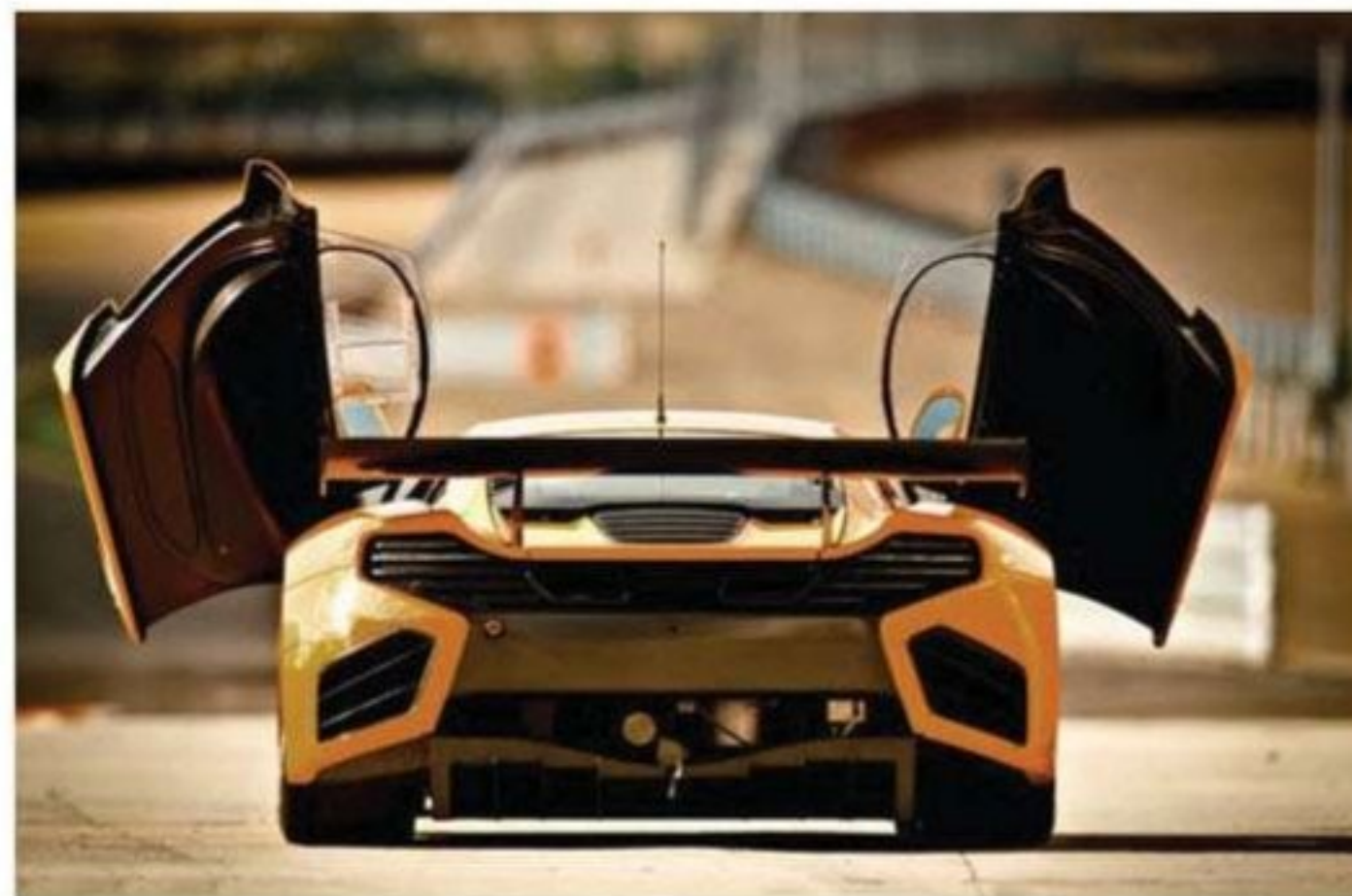
A single plane rear wing is used on the racecar version in place of the road car's automatically-adjusted aerofoil. Ducting has also been revised
