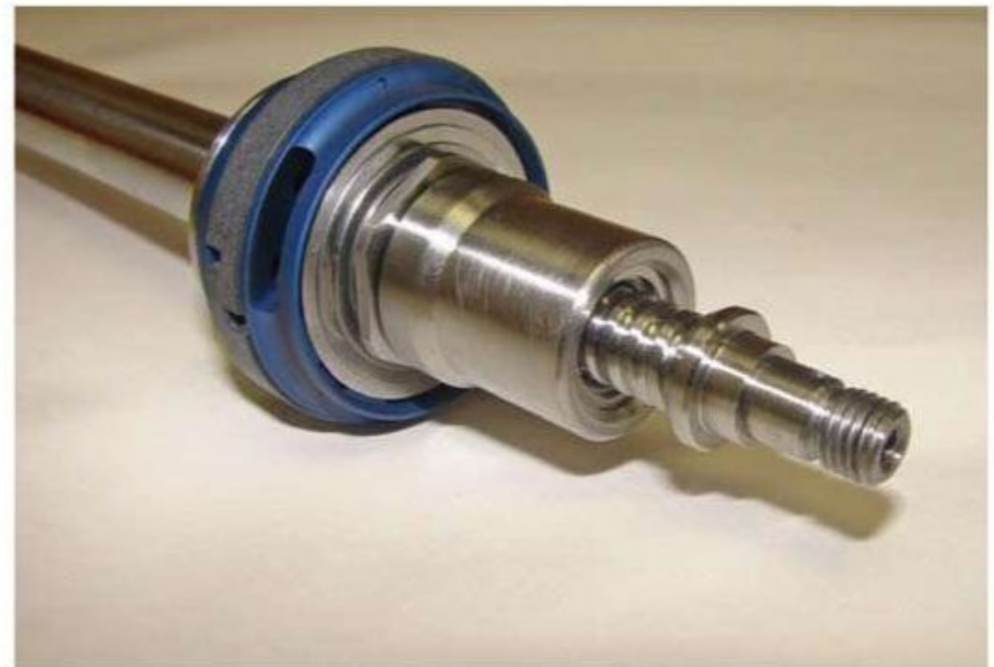
The ball screw and rotating weight arrangement in close up is revealing in respect of the order of mass involved
