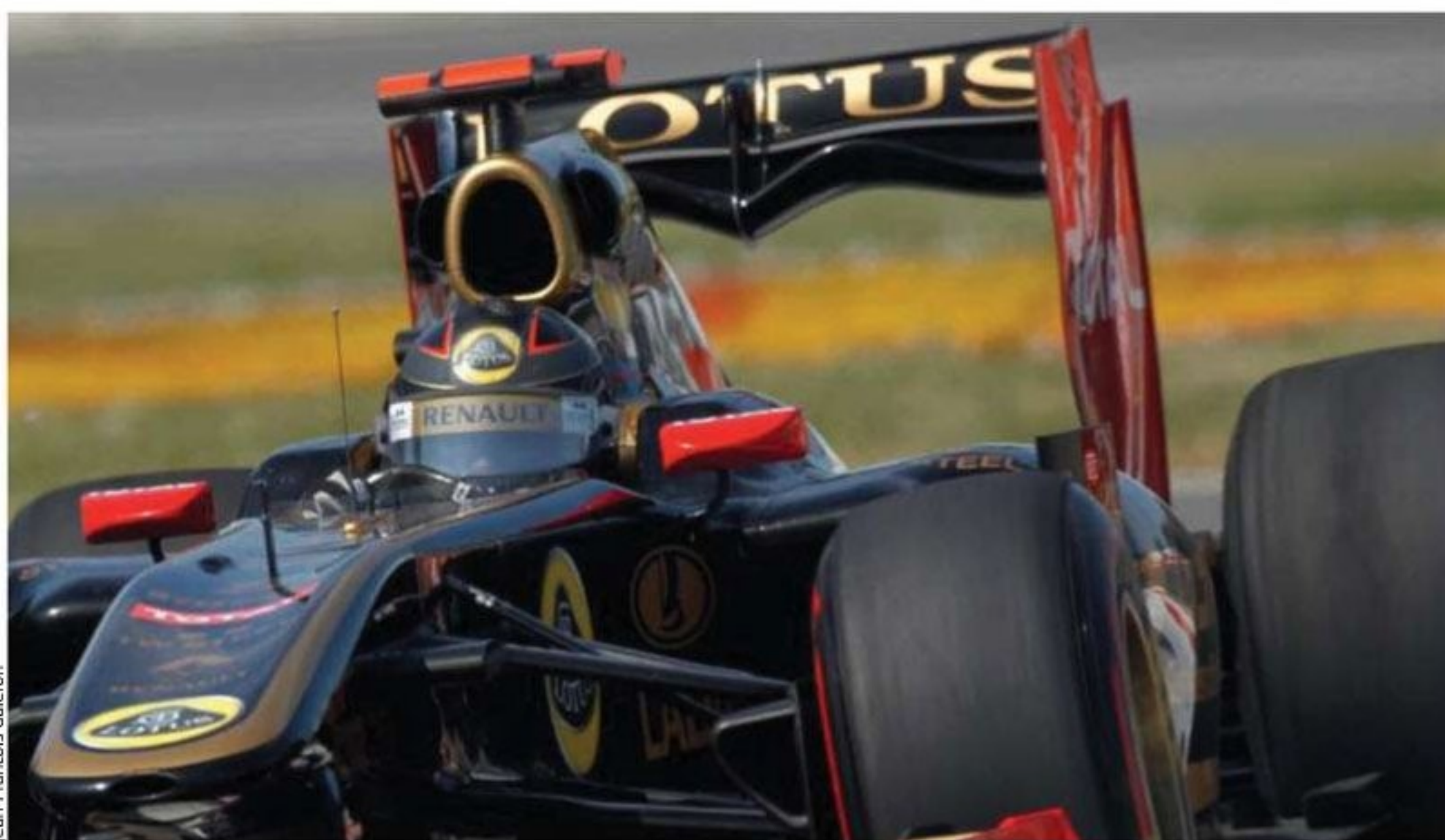
In Montreal the car was tested with this ultra swoopy rear wing in an attempt to reduce drag. It is identical in concept to a similar wing trialled, but not raced, on the R30 of 2010. This is one of the very few carry-over items
