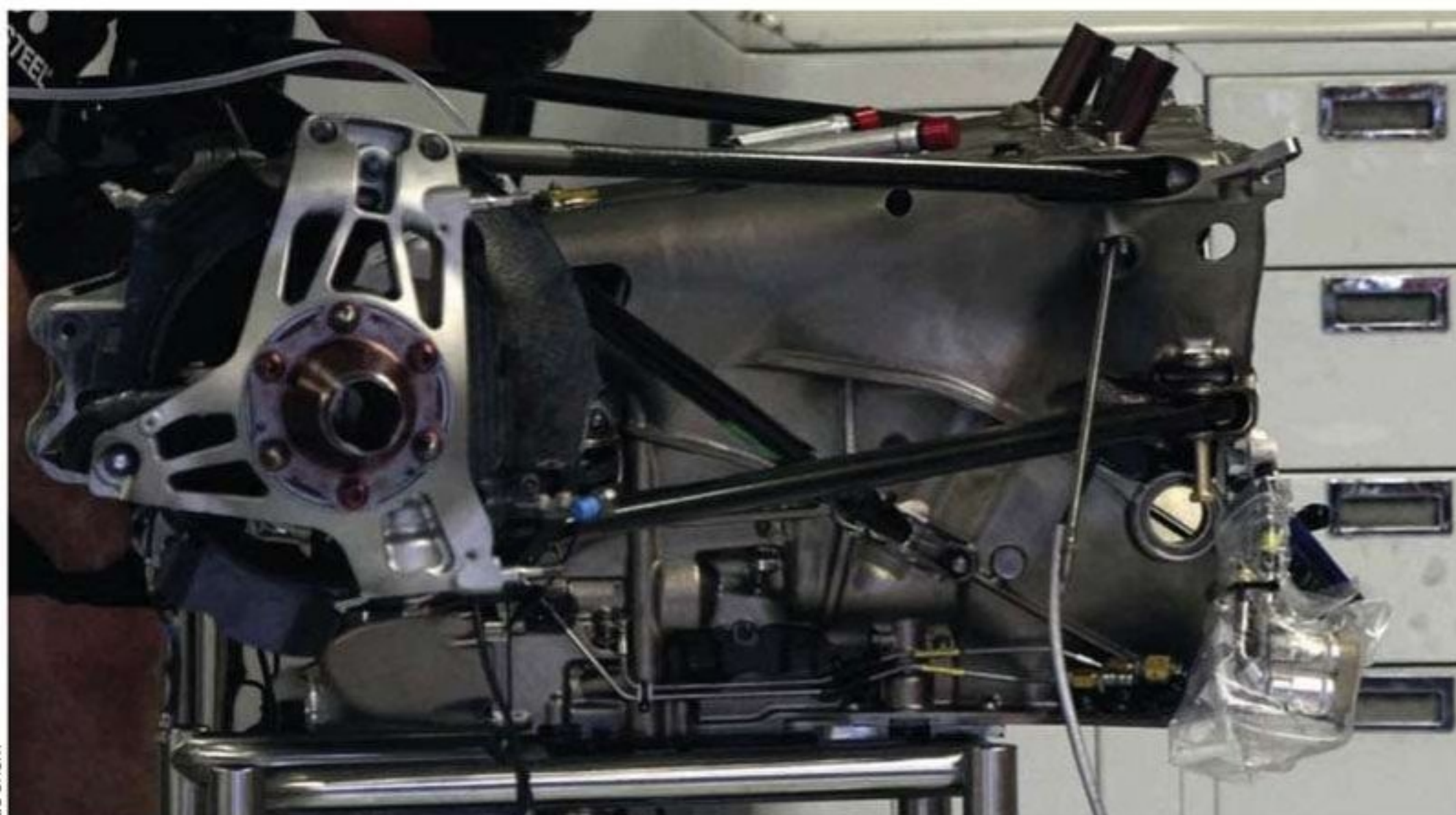
For the R31, LRGP adopted a pull rod rear suspension layout, although James Allison claims that in aerodynamic terms there is not much to choose between this concept and a more conventional push rod set up
