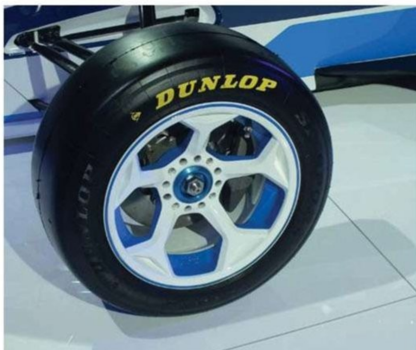
Garish Rimstock wheels look more like aftermarket road car alloys but are a further spec part designed to keep costs down. Wheel tethers are also used
