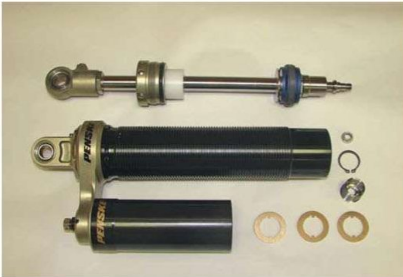
Penske Racing Shocks hybrid damper / inerter disassembled. Look top right for the interesting new bit...
