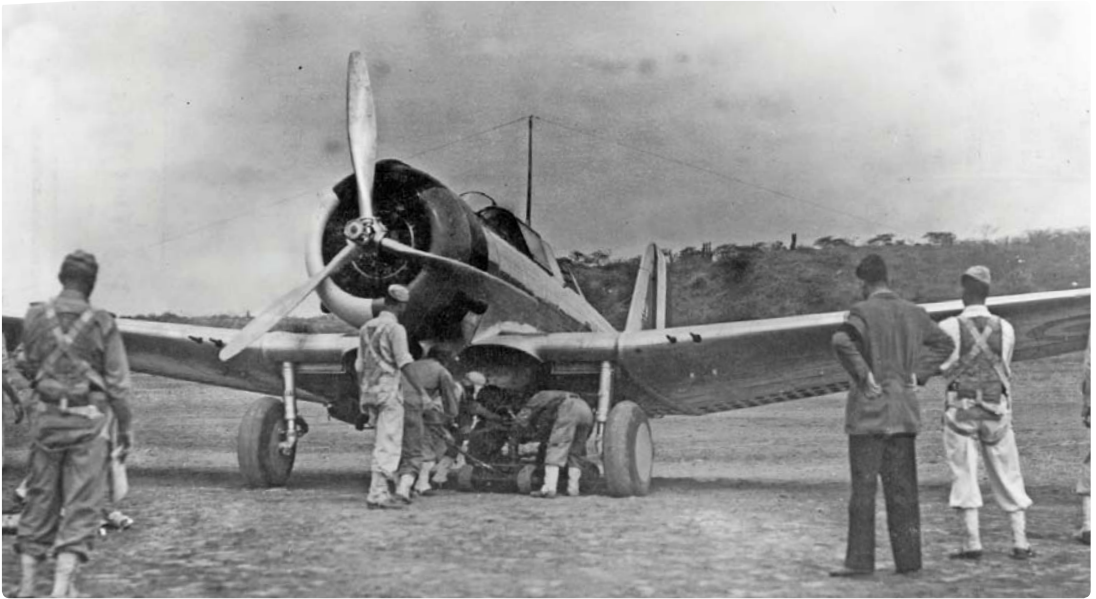
ABOVE The CAP's 8As were used extensively during the conflict with Ecuador, often as bombers; here an 8A-3P is rearmed with fragmentation bombs before another bombing sortie from Tumbes forward airfield on the Peru-Ecuador border, in late July 1941. The 8A was also fitted with a pair of Browning 0.3in machine-guns in each wing.
