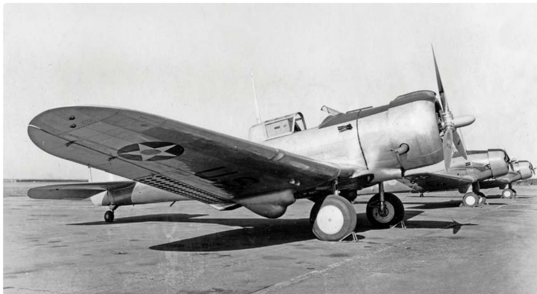
ABOVE Fitted with a 1,200 h.p. Wright GR-1820 Cyclone engine and machine-gun gondolas under the wings, the 8A-5 was the most powerful and heavily armed variant of the Northrop/Douglas series of attack aircraft. Norway's 8A-5s became A-33-DEs in USAAF service, an example of which is seen here at Kelly Field, where they were stored.
