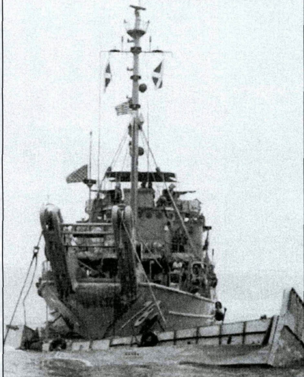
The last class of ANs built in WWII were the steel-hulled Cohoes -class in 1944/1945. They were 168-ft LOA and were rated at 560-tons with 1000-shp diesels. ANs carried wartime crews of from 48 to 60 men, depending on their gunnery requirements. Here, class leader Cohoes (ANL-78) is seen lifting a sunken 50-ft LCM. They carried hull numbers AN-78 to 92.
