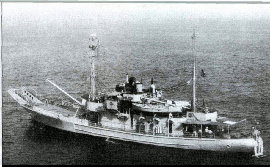
A good side view of USS Butternut showing the variety of deck gear that was their stock and trade. Their forward boom was rated at 12-tons lifting capacity. Originally designated YNs, they were reclassified ANs in December 1942.
