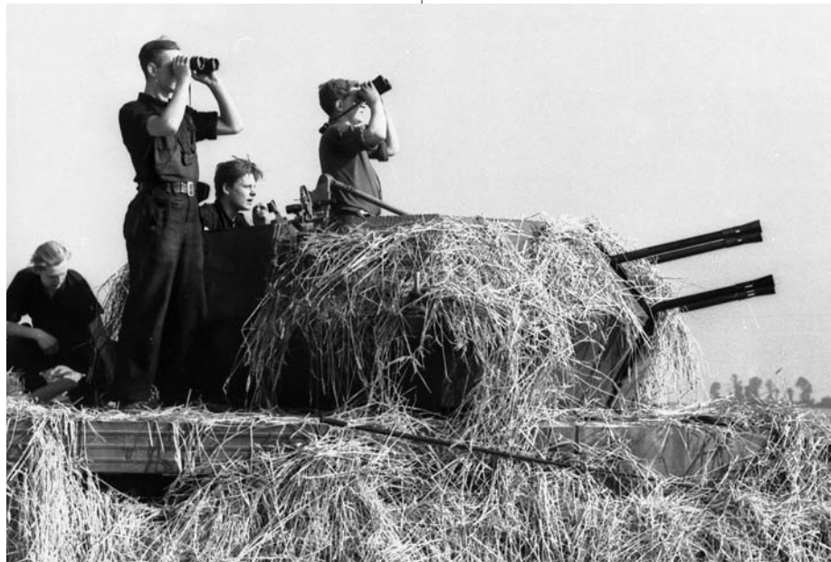
Germans man a camouflaged Flakpanzer IV Wirbelwind ("Whirlwind"), a self-propelled anti-aircraft gun outfitted with a 2cm Flakvierling 38 auto cannon, at the air base in St. Malo, summer 1944.
