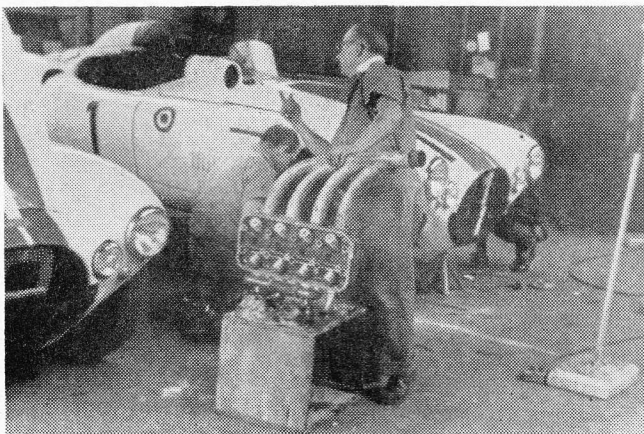
5½-LITRES: A pre-race scene in the Cunningham workshop, showing one of the V8 Chrysler engines.
