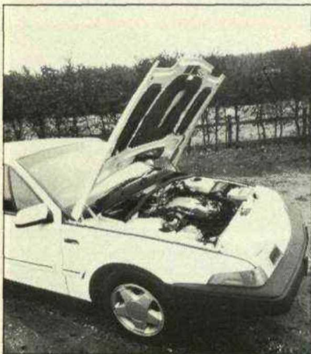
Headlamp pods are switched so that they cannot be raised while the short bonnet is up.
