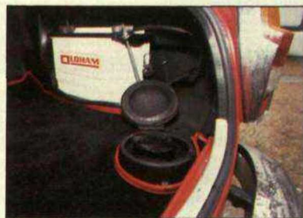
Fuel filler is concealed inside boot with flip-top and screw caps to prevent fumes.
