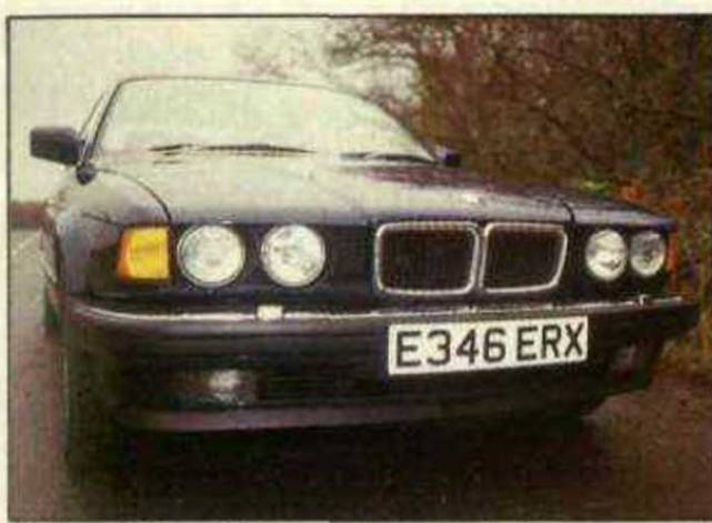
Ellipsoid headlamps have superb throw on main and very sharp cut-off on dip.
