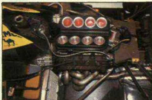
Cosworth's 3½-litre DFR V8 will be used by Benetton in preference to turbo power.
