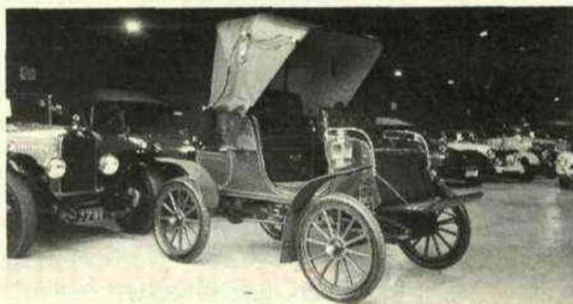
1903 Stevens Duryea. Twin cylinder, 4 seat Brighton runner in magnificent condition, v.c.c. dated.
