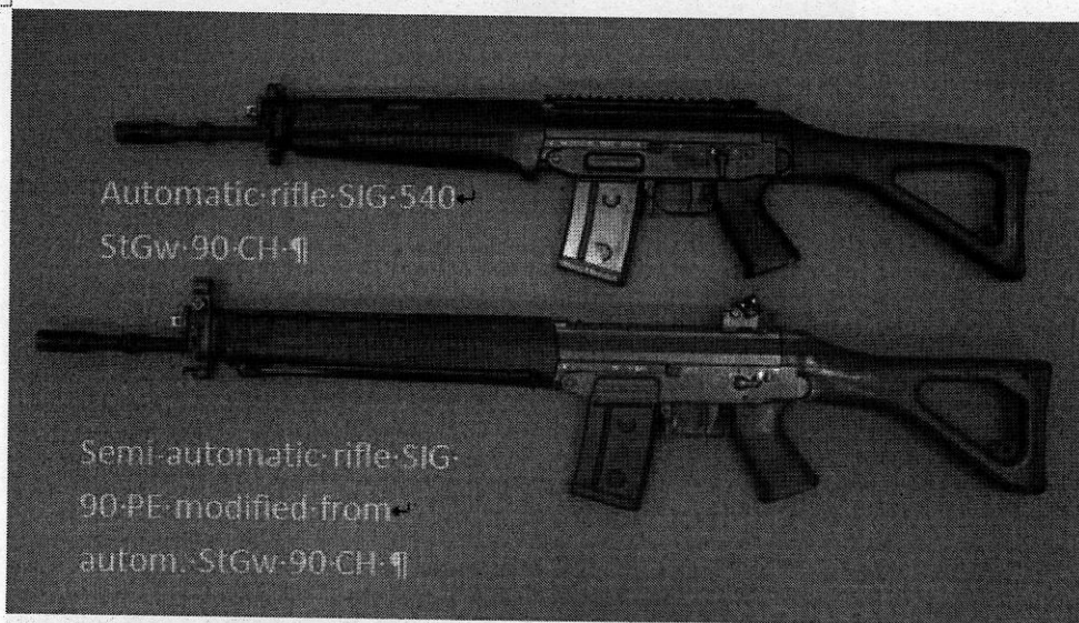
Pic. 6: Semi-automatic rifle SIG-90-PE, modified from full-automatic rifle SIG-540/StGw-90, cal. 5.56mm x 45.
