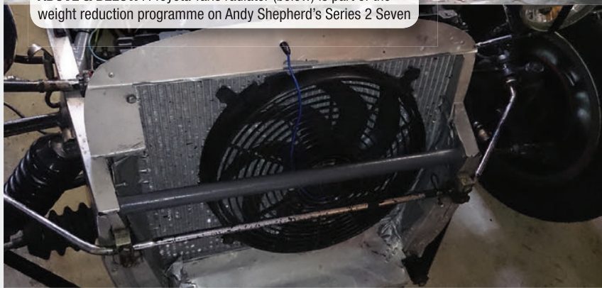
ABOVE & BELOW A Toyota Yaris radiator (below) is part of the weight reduction programme on Andy Shepherd's Series 2 Seven
