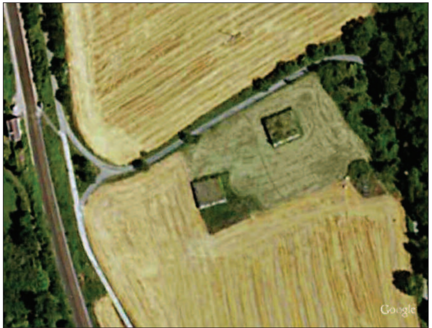
Trees now hide most of the 'W 2' bunkers from aerial observation but the pair of bunkers at Vauxaillon show up clearly. Type 108A ammunition bunkers measured 16.8 by 18 metres, with walls and ceiling three metres thick, and featured two storage rooms, each six by three metres. The road from the bunkers to the tunnel (seen on the left alongside the railway line) is the original German concrete road.
