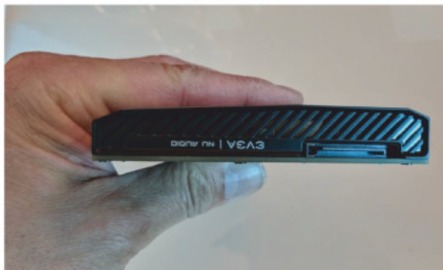
The card is powered by a single SATA connector.
