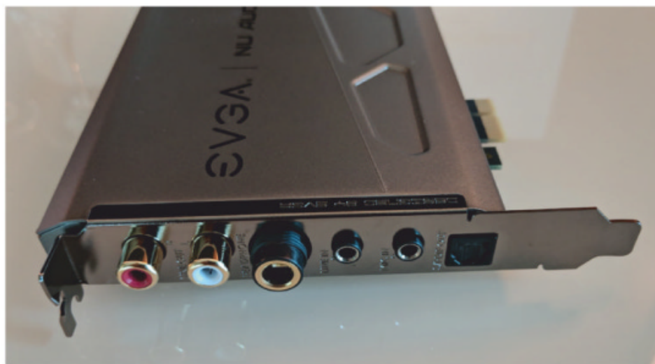
Ports: RCA, quarter-inch, two 3.5mm jacks, plus TOSLINK.
