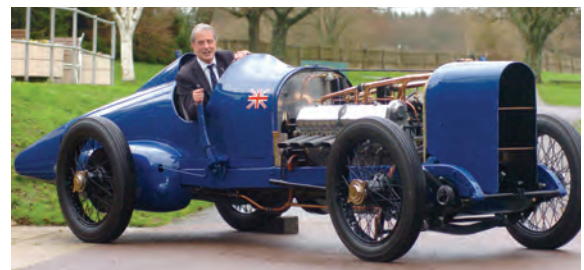
ABOVE Sir Malcolm Campbell's grandson, Don Wales, in the record-breaking 350 hp Sunbeam. The modified aero engine, an 18.322-litre V12 Manitou Arab, was rebuilt with Formhalls bearings in 2008
