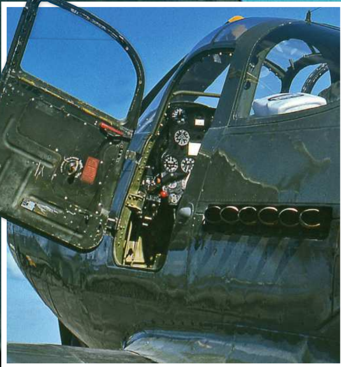
The unusual cabin-style cockpit of the Airacobra, with car-style doors
