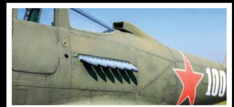
The position of the engine led to unorthodox placement for the supercharger air intake and the exhausts
