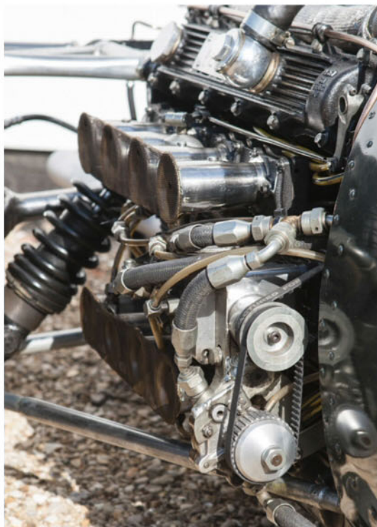
The complex H16 needed an array of pulleys, cams and gears to get it to function correctly and all this just added weight to the unit
