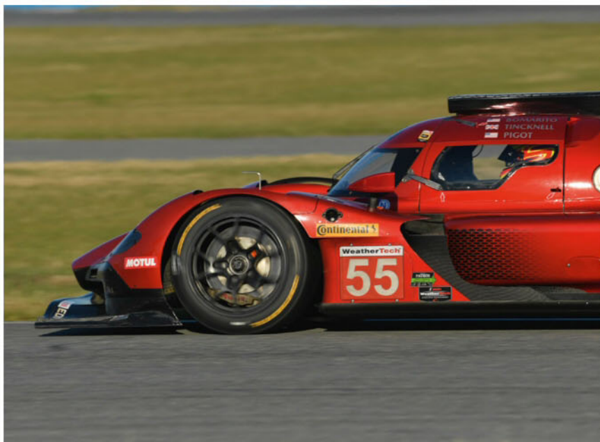
The front end of the car has seen very little development over last year's version. This is partly because major changes to the suspension here would have meant knock-on changes to the tub, entailing another crash test
