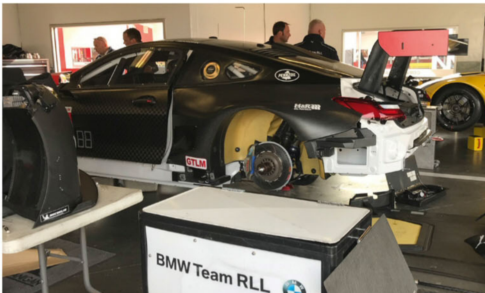
Suspension is conventional double wishbone set-up with 4-way adjustable shocks front and rear. Car body is composite
