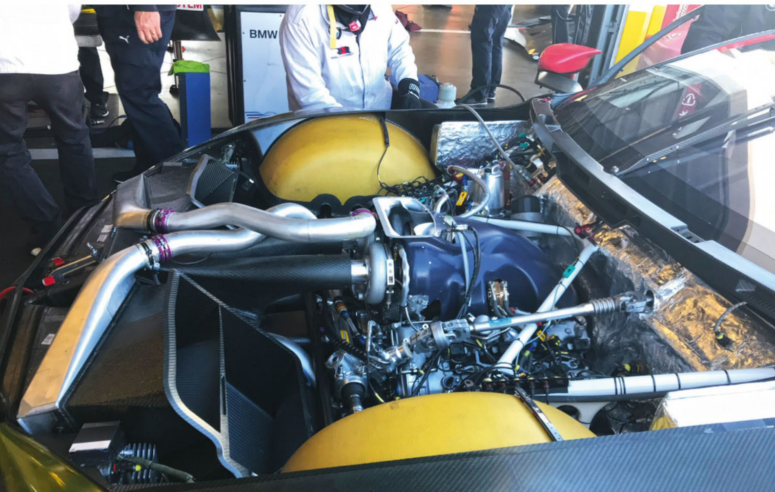
The engine is based on the 4.4-litre unit that saw service in the M6 GTLM car last season, but capacity has been cut to 4 litres while BMW has also adopted a twin-turbo layout
