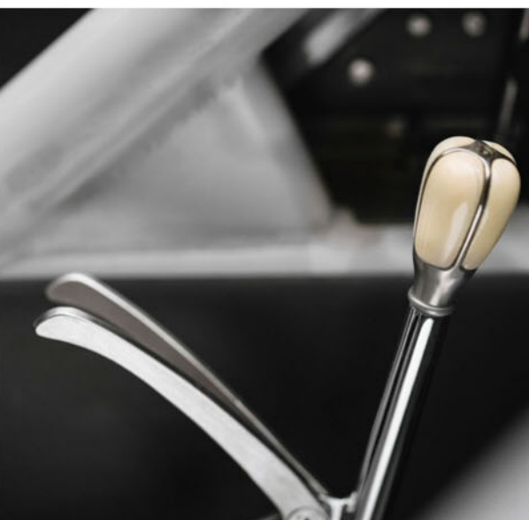
Many of the parts on this record car are pleasingly low-tech, such as this hand-operated lever for the wheel brakes. The brake system features Wilwood discs and pads that last for just a few seconds
