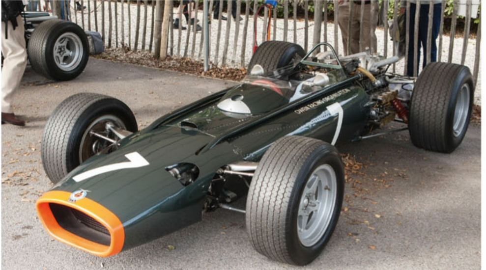
The first Formula 1 car to pack the H16 was BRM's 1966 entry, the P83. Note the routing of the water pipes outside the car
