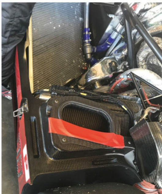
Radiators are blanked off for the cold temperatures at Daytona. Ironically, overheating was a big problem for the car last season
