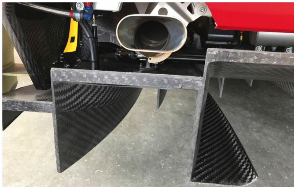
Ferrari kit also includes a reworked diffuser and newly shaped exhaust pipes; the latter to maintain the gap between the two
