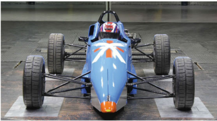
The early 2017 narrow sidepod configuration. Frontal area was reduced by three per cent
