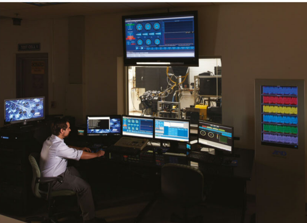
Combustion Analysis Software is used on the test bench to tune the engine, for calibration, and for defining the knock limits
