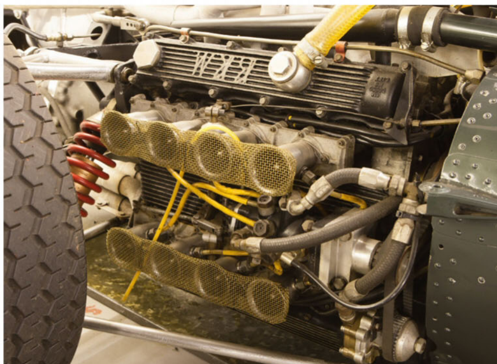
One of the H16's unsung legacies is that it was the first engine to be used as a fully stressed member; before the DFV in '67
