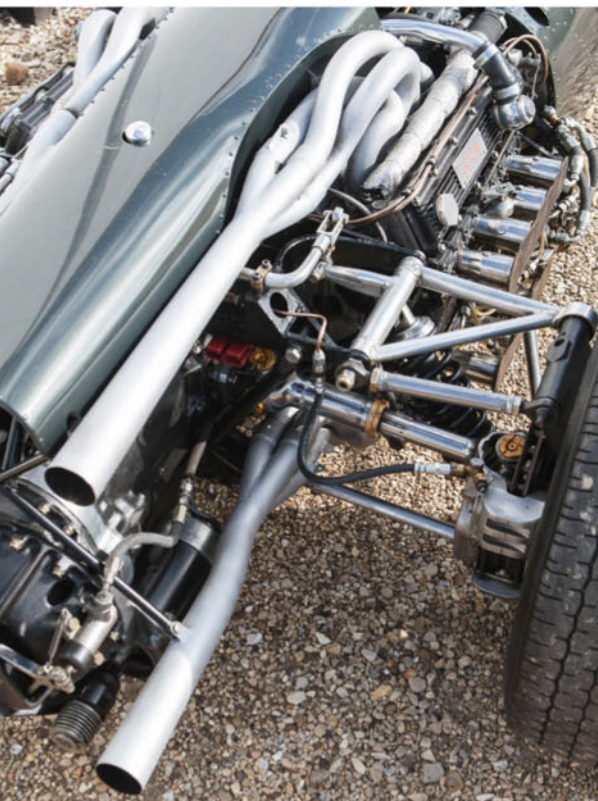
Early 3-litre F1 cars were noted for their elaborate exhaust layouts and the P115 was no exception with its under-and-over approach
