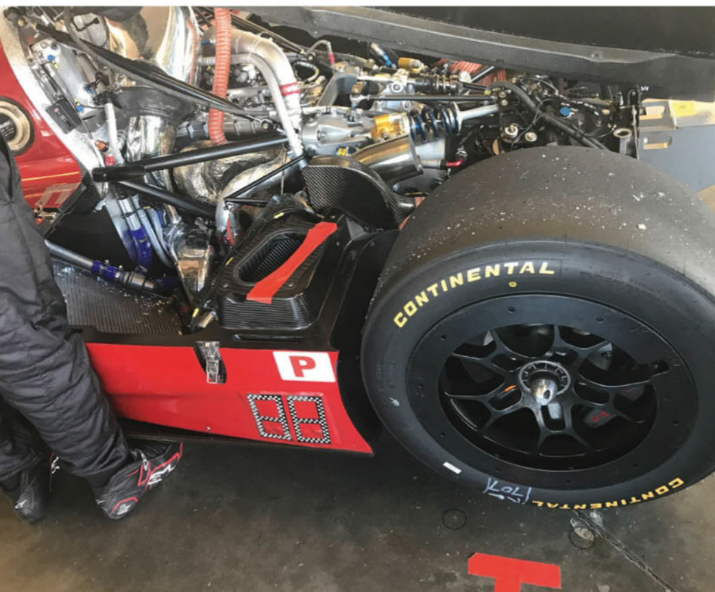
Much of the work has been focussed on cooling. The original car had the radiators stood up in the sidepods but these have now been made bigger and placed at an angle, while there's also been an effort to improve the airflow going through them
