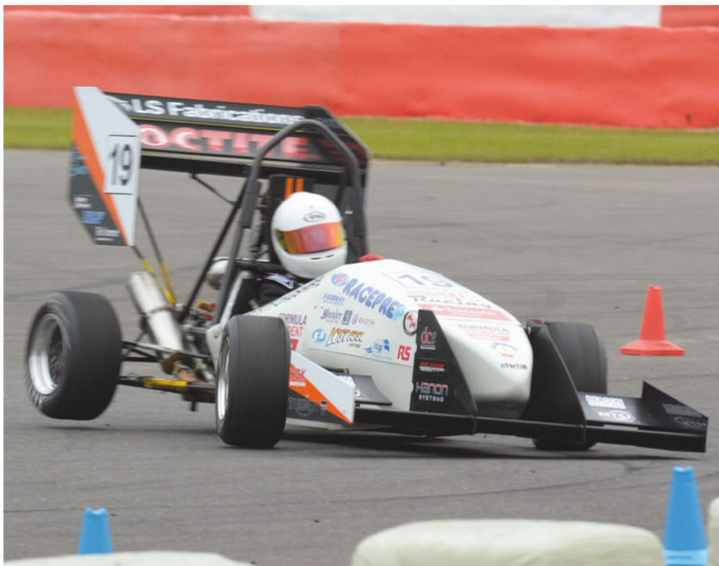
The three main goals you need to keep in mind during your Formula Student project's concept phase are keeping the car weight to a minimum, with the lowest possible centre of gravity and minimal yaw inertia
