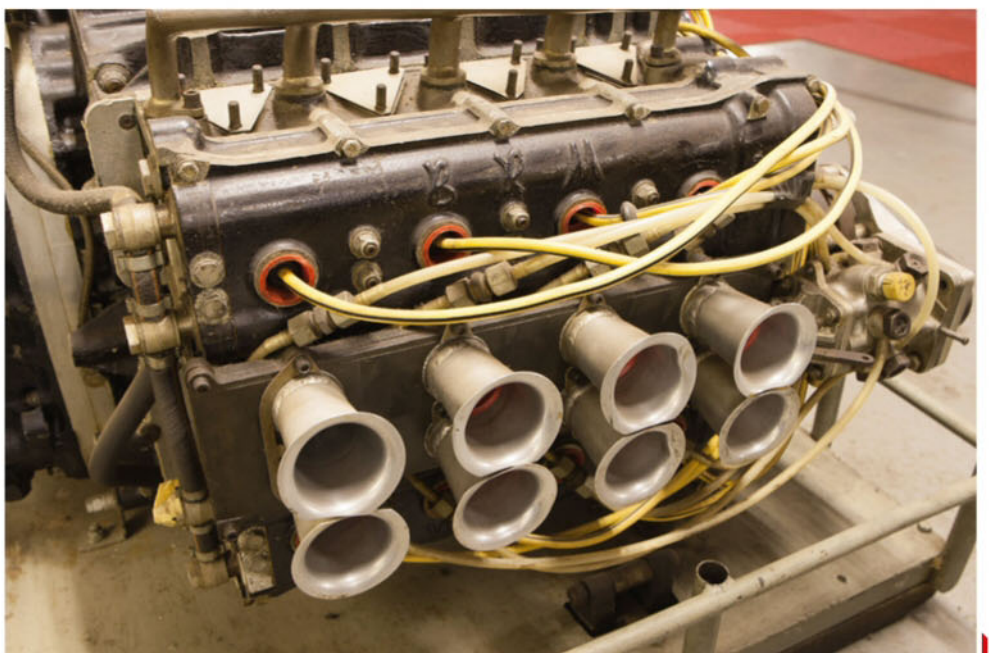
BRM's old V8 engine had inlet ports between the camshafts. This allowed the H16's intake trumpets to stick out of the sides
