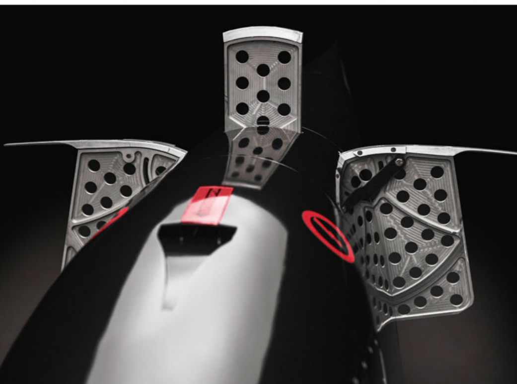
Airbrakes deployed. Most of the retardation actually comes from parachutes fired out from the rear of the car. There were problems with these at early tests due to the disturbed salt that was thrown up behind the record car chewing up the chutes
