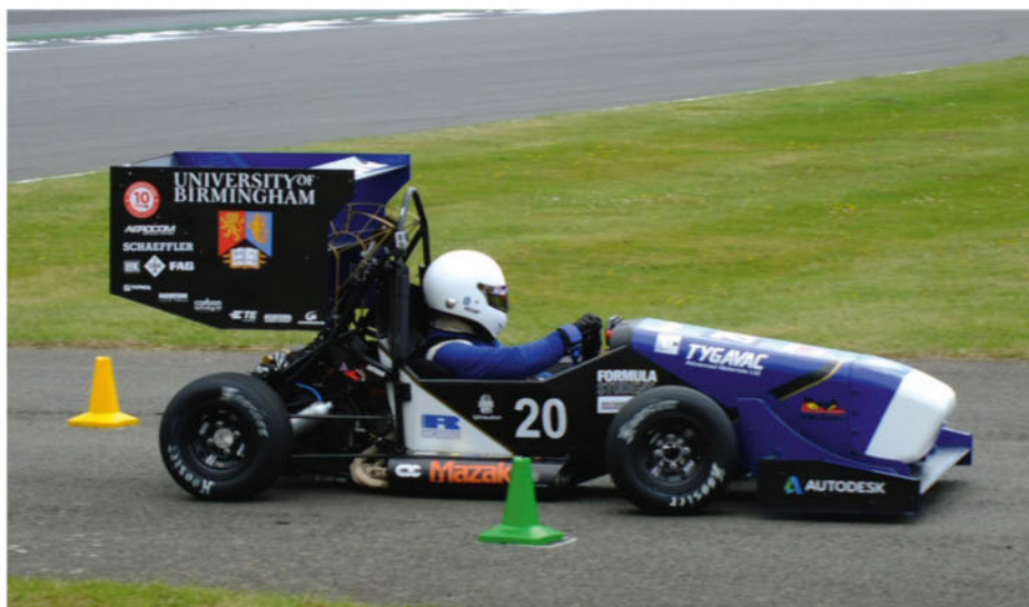
A common error with Formula Student teams is not simulating or measuring steering torque, making the car hard to drive on the handling tests. This needs to be no more than 5Nm; road cars are around 3Nm
