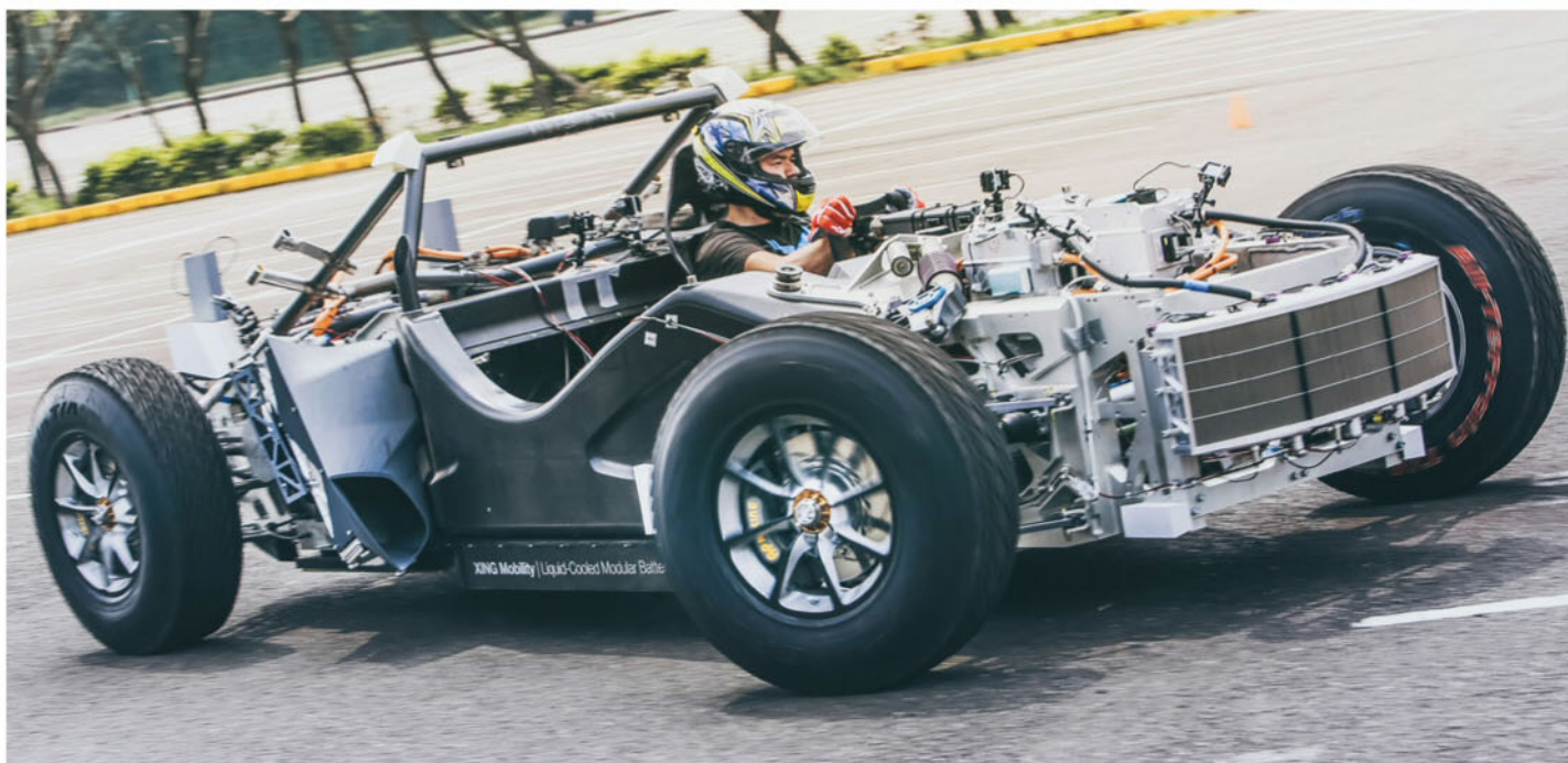
Naked Miss R in testing. It has a projected performance of 0-100kmh in 1.8s, 0-200kmh in 5.1s, with a max speed of over 270kmh. Battery pack can produce one megawatt of power
