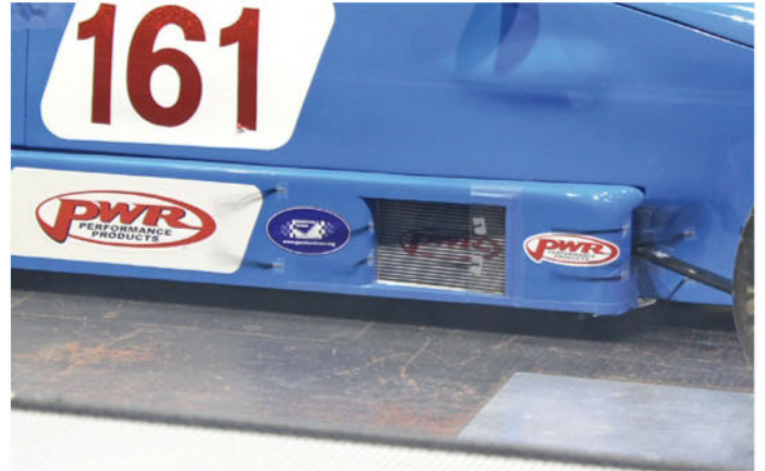
Satisfactory flow into and out of the radiators is revealed here with the use of wool tufts, although the flow ahead of the lower inlet did seem to prefer to go under the car
