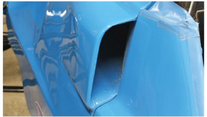
The Swift's original scoop duct to feed the engine inlet was an obvious drag generator
