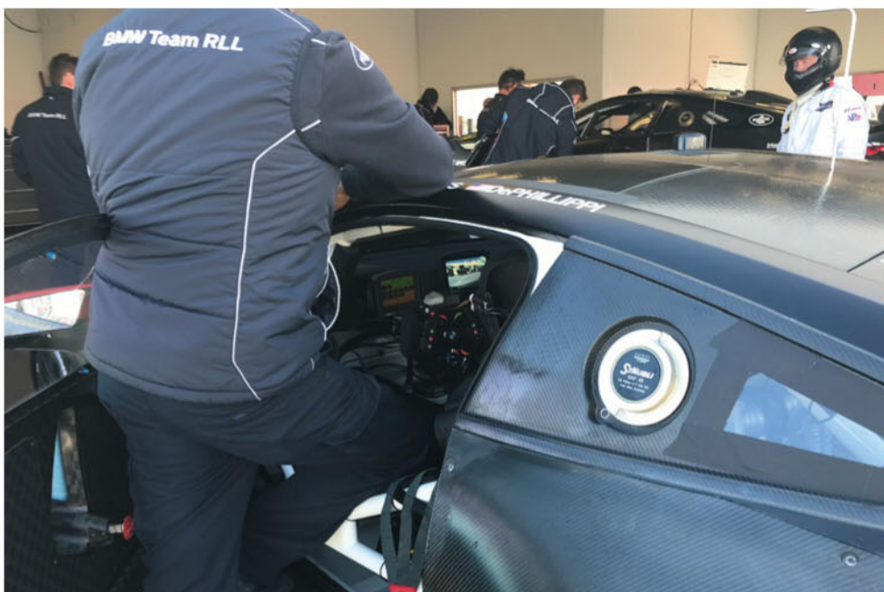
In the cabin the seat is fixed, with the pedals adjustable, while it has also been moved a little closer to the centre of the car
