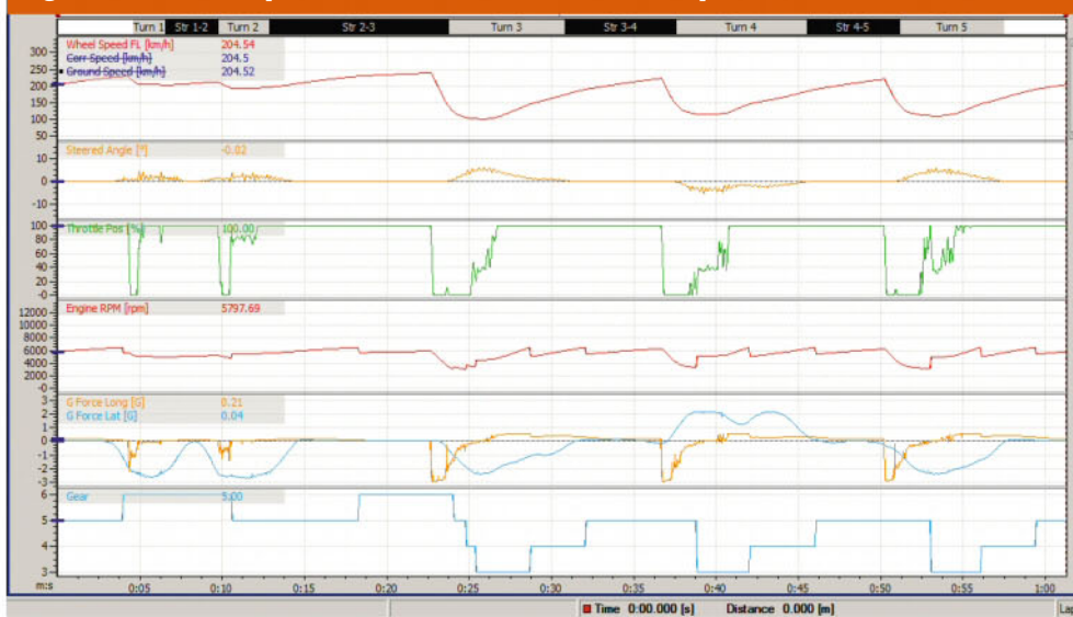
Figure 4: Plot of speed, throttle and RPM for a lap with a conventional car
