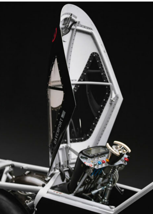
The dash tilts up to allow the driver easier access to the cockpit. Canadian drag racer Les Davenport took over the driving duties after car builder Marlo Treit crashed a previous record racer
