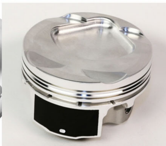
Above and right: Up to 20 per cent of the energy that an engine produces is lost to friction, with as much as half of that due to the piston skirts and rings contacting the cylinder wall. This can be significantly reduced with the dynamic Perfect Skirt coating
