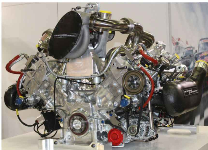
The turbo is mounted in the centre of the vee. New compressor and turbine could be developed after Le Mans
