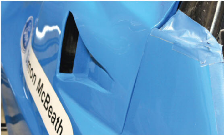
The mid-2017 upgrade featured this NACA duct engine inlet, which was sized to match the rpm and speed regime encountered. This reduced the car's drag by a further 0.6 per cent
