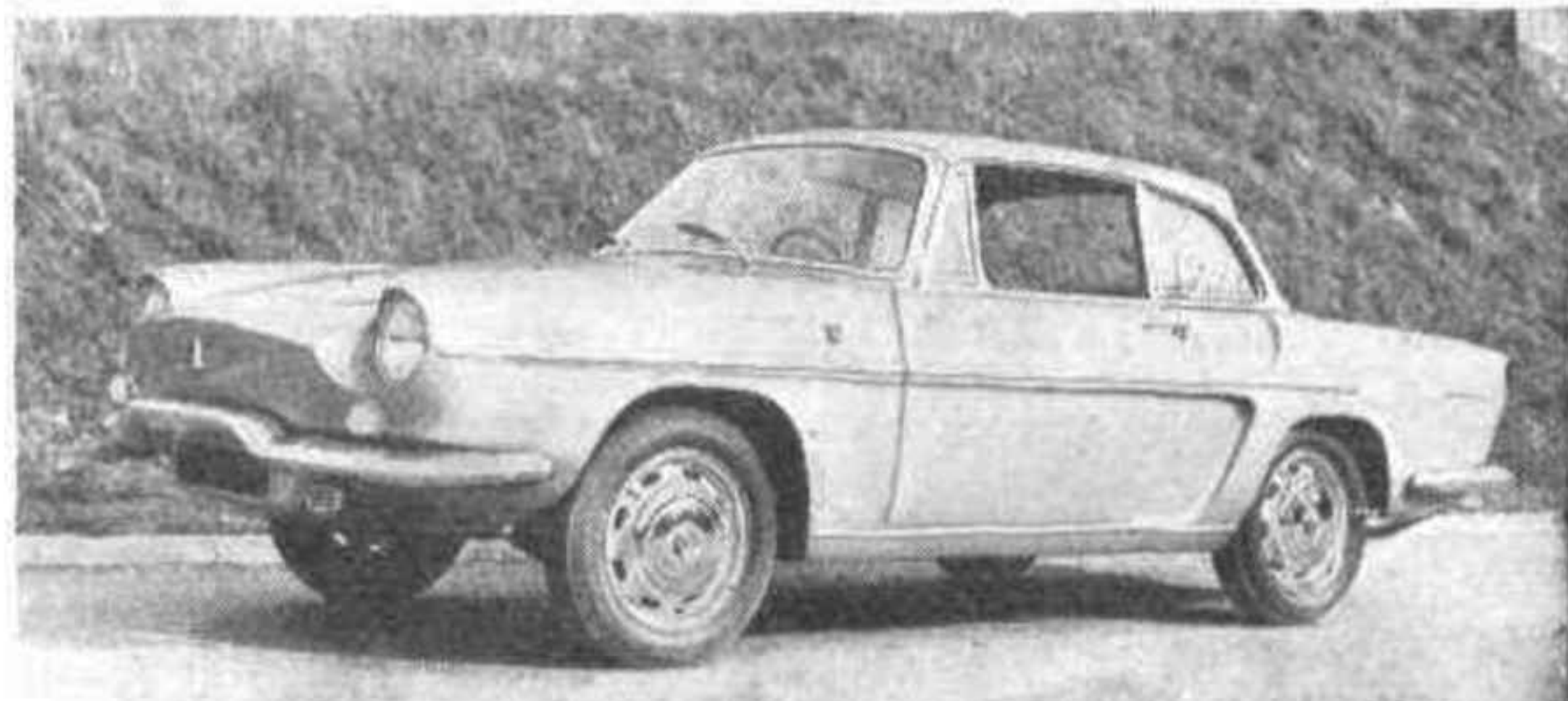
The new 956-c.c. Renault Floride coupé, recognisable by the changed shape of the roof, elimination of air intakes ahead of the rear wheels, and slotted wheel discs.
