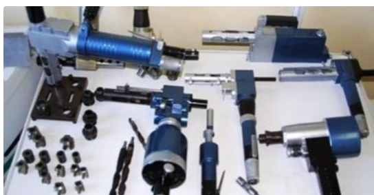
UkrRIAT's pneumatic tools for airframe assembly (Image courtesy of UkrRIAT)
