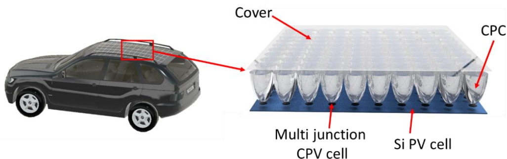
Figure: Design concept of a solar concentrator photovoltaic for vehicle application based on compund parabolic concentrator (CPC)
