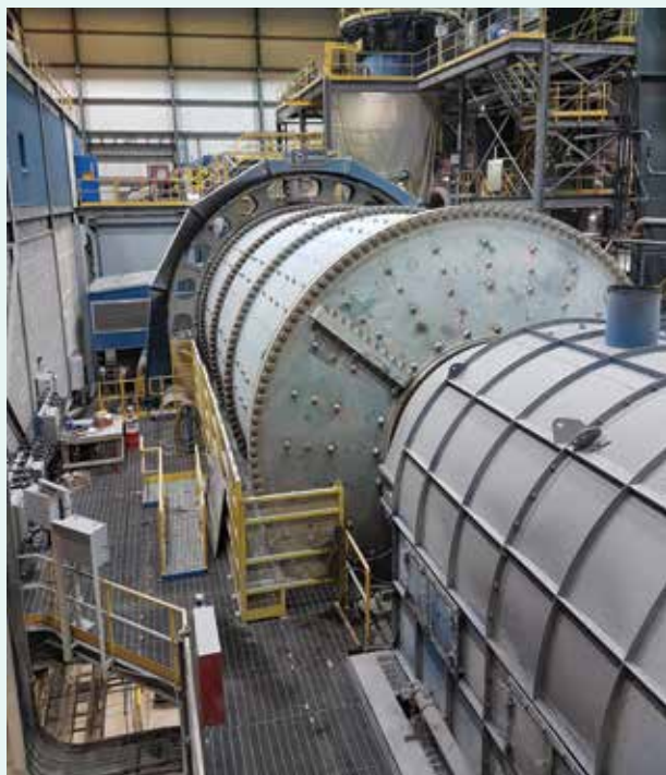
A semi- autogenous grinding (SAG) mill at LSG's ore-processing mill, one of the most-energy intensive equipment at that site.
