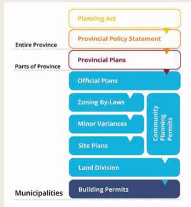
Figure 4.19. A schematic showing the land use planning framework in Ontario, from provincial (top) to local (bottom).
