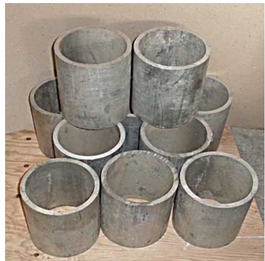
Bearing housings ready for machining
