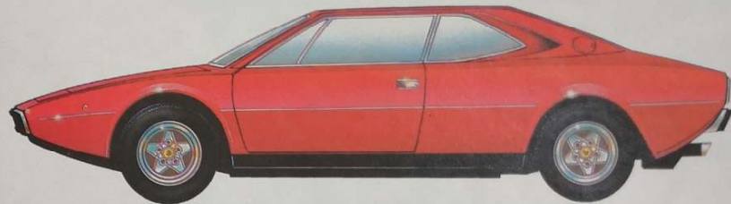
Ferrari 308 GT4 2+2 coupé. Coachwork by Bertone. Transverse mounted 90° 2926 cc four overhead camshaft V8 engine producing 255 bhp at 7,600 rpm.
