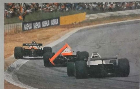
11. ... because the Alfa driver no longer has any rear downforce. His wing is out of position, and Bruno is overtaken by Daly (one lap behind) and Zunino before stopping in the pits.
