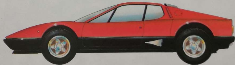
Ferrari BB 512. Coachwork by Pininfarina. Horizontally opposed 12 cylinder four camshaft 4942 cc engine producing 360 bhp at 6,800 rpm. Electronic ignition. Dry sump lubrication.
