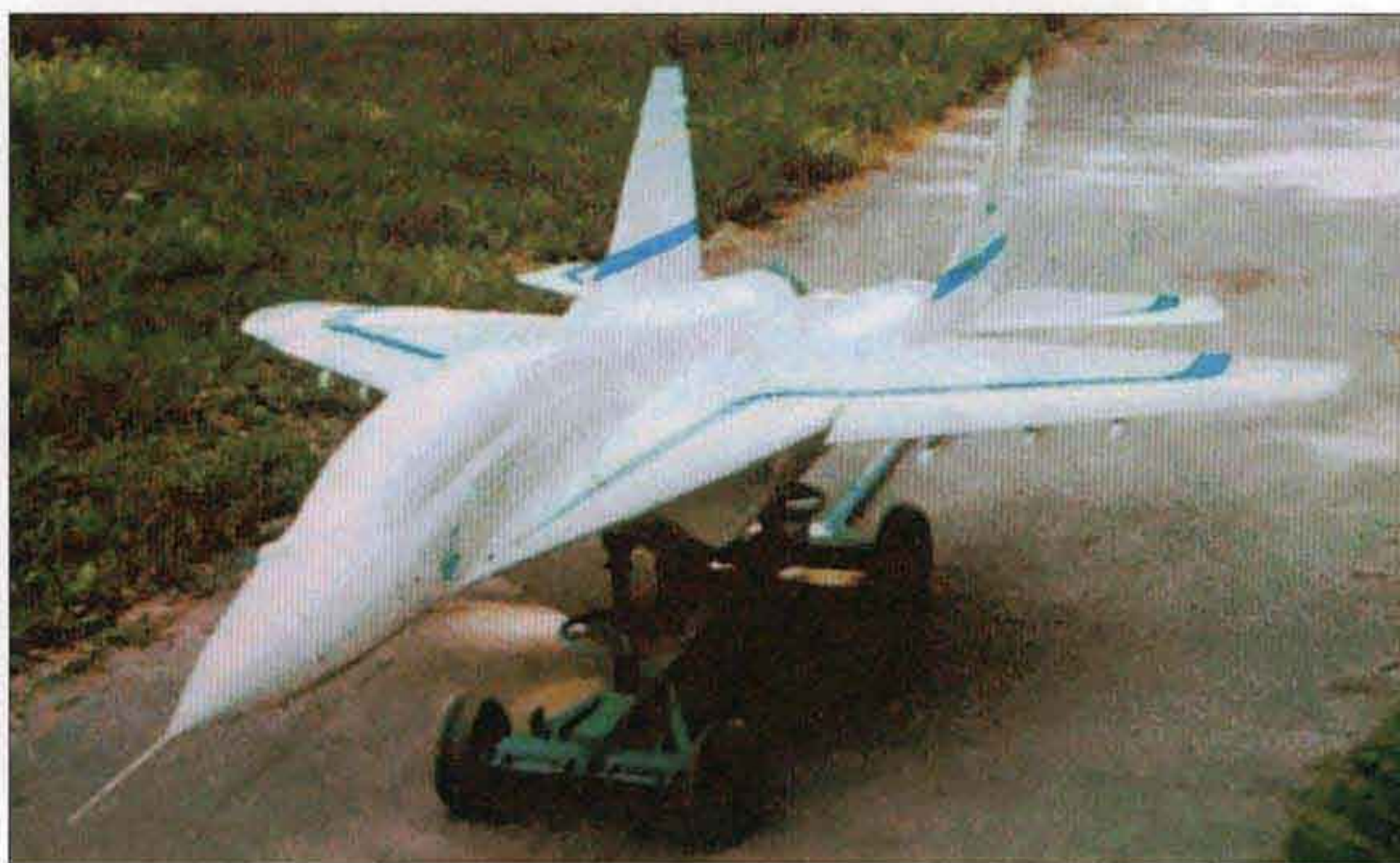
▲ The 1/4th scale gliding model built by LII to explore the control characteristics of the MiG-29M2. It is catapult-launched and lands on a parachute at the end of the mission.
