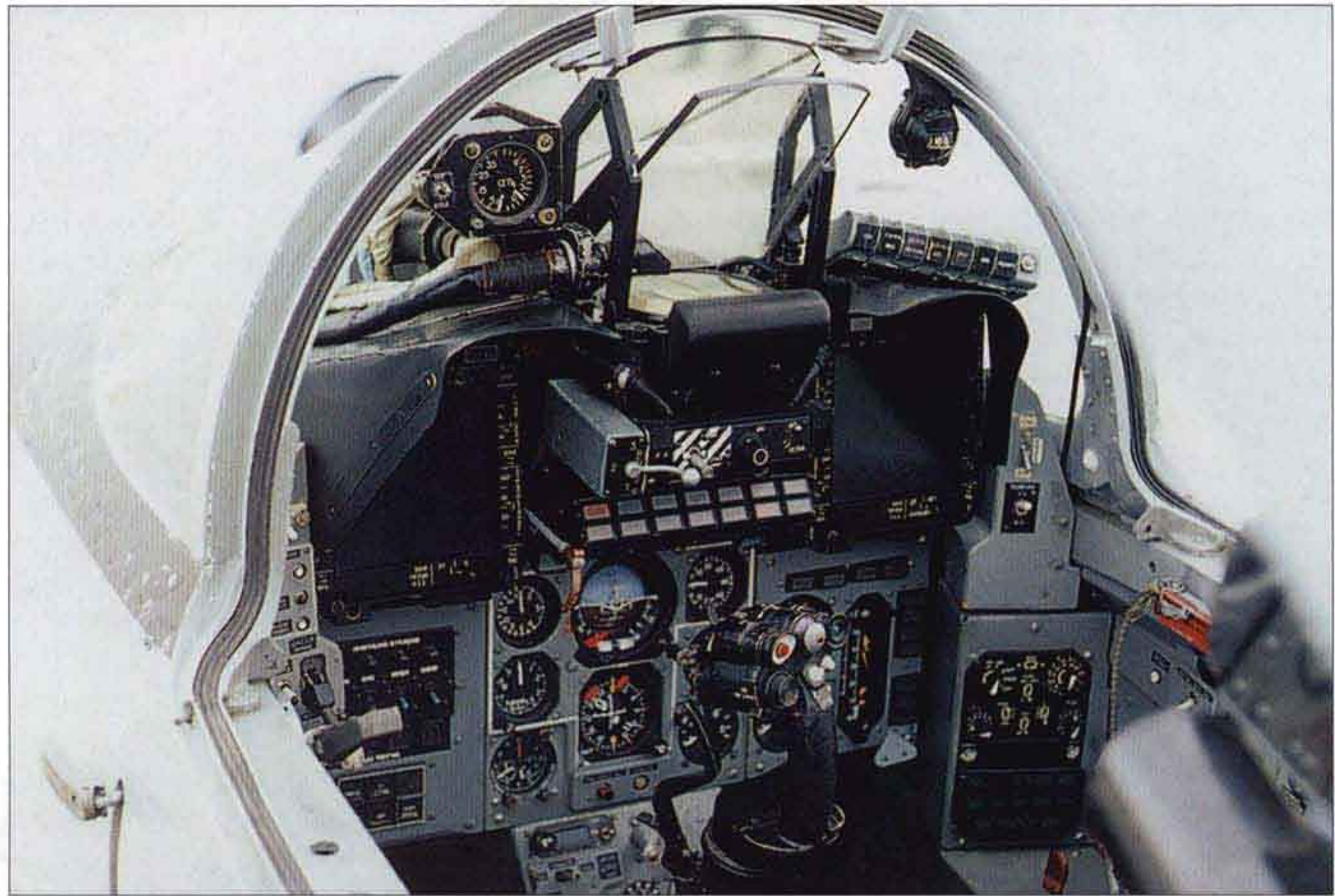
► The cockpit of MiG-29M '155 Blue'. Note the new HUD.
