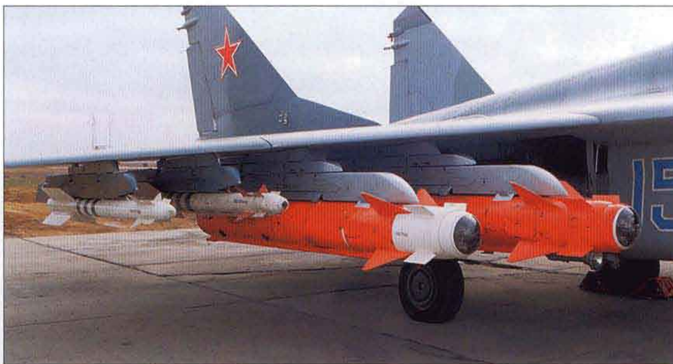
▲ Close-up of the finless Kh-29T AGMs and dummy R-73s under the starboard wing of '155 Blue'.
