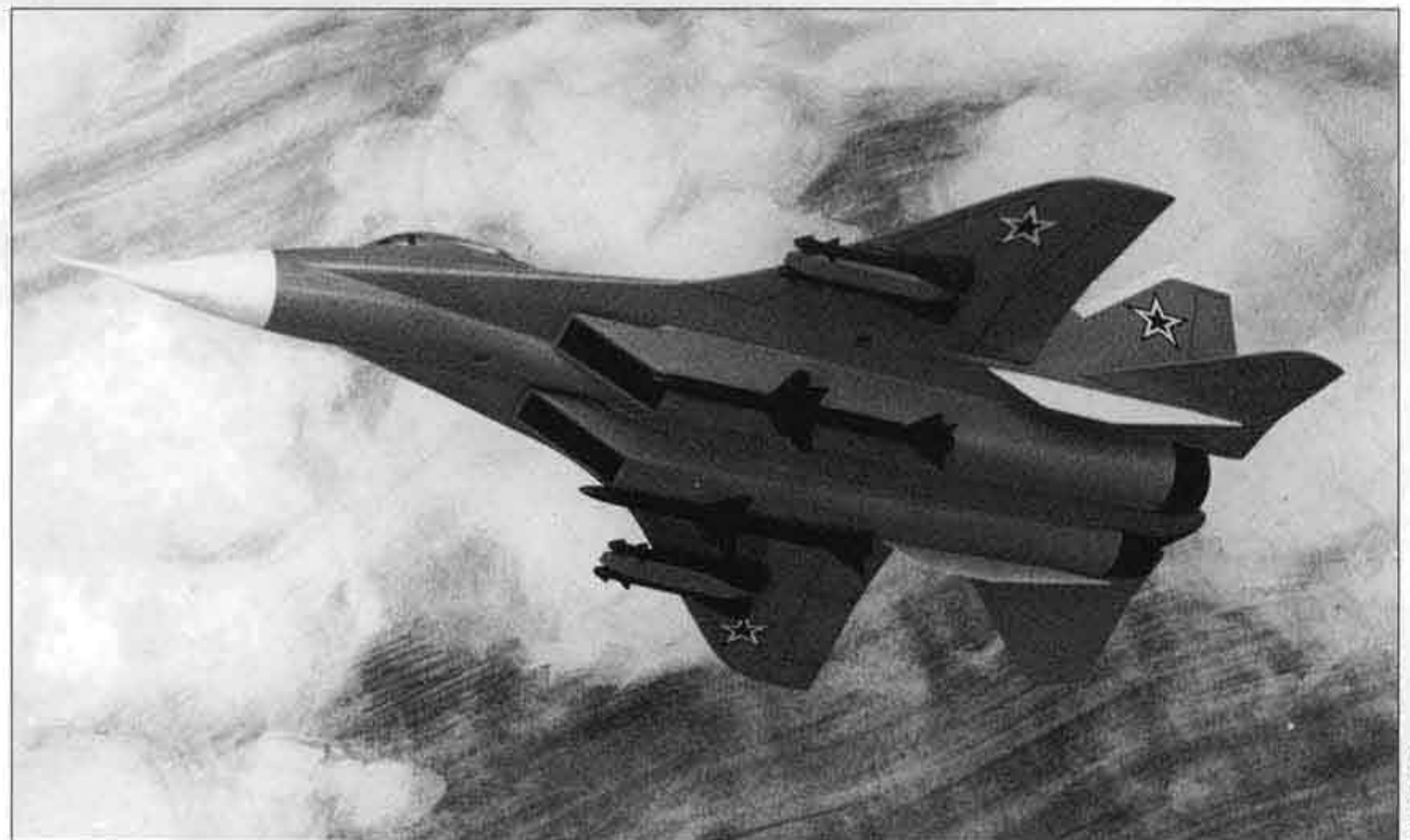
An artist's impressions of the MiG-29 ( izdeliye 9.11 ) project. The aircraft is extremely similar to the real thing but looks more stubby and has an ogival wing leading edge; the ventral strakes are longer and positioned far from the engine nacelles, and the medium-range AAMs are still positioned on the air intake trunks. Note the auxiliary air intakes in the LERXes.
