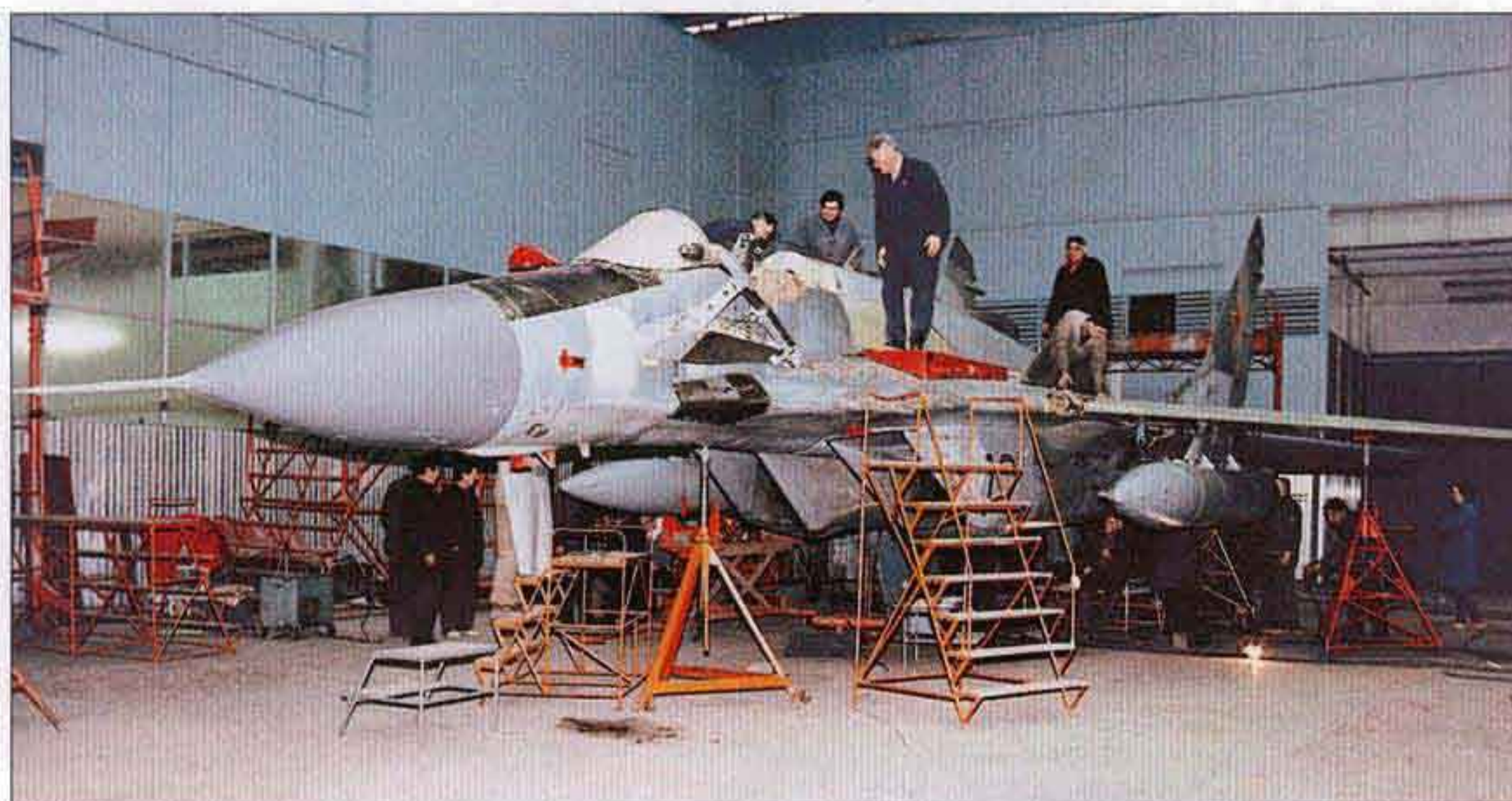
▲ MiG-29 Fulcrum-A '12 Blue' (c/n 2960520165) in the process of conversion to a MiG-29SMT at ANPK MiG's experimental shop in Moscow. Note the IFR probe.
