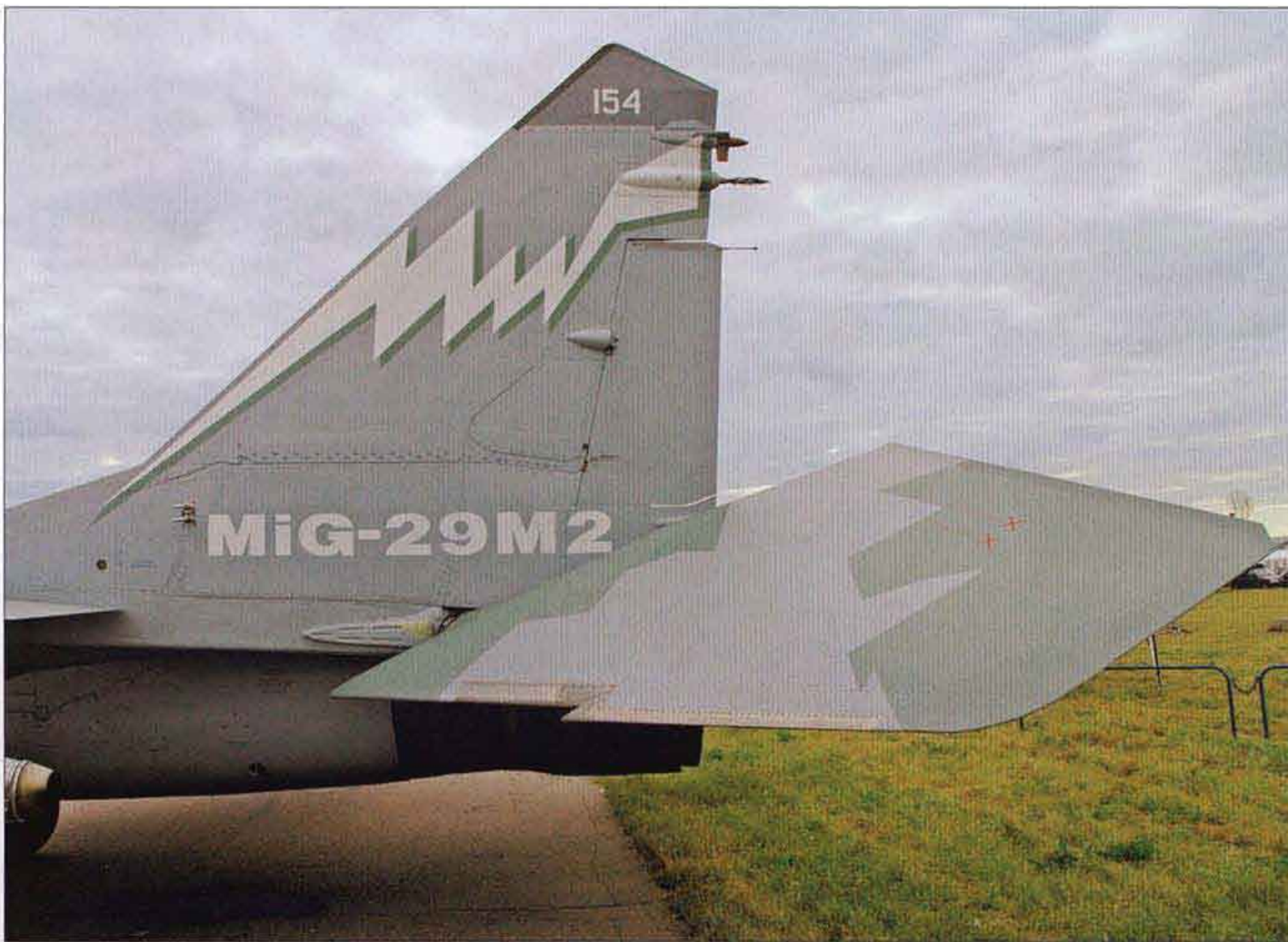
◀ The stabilators of the MiG-29M and its derivatives feature a leading-edge dogtooth energising the airflow at high angles of attack.
