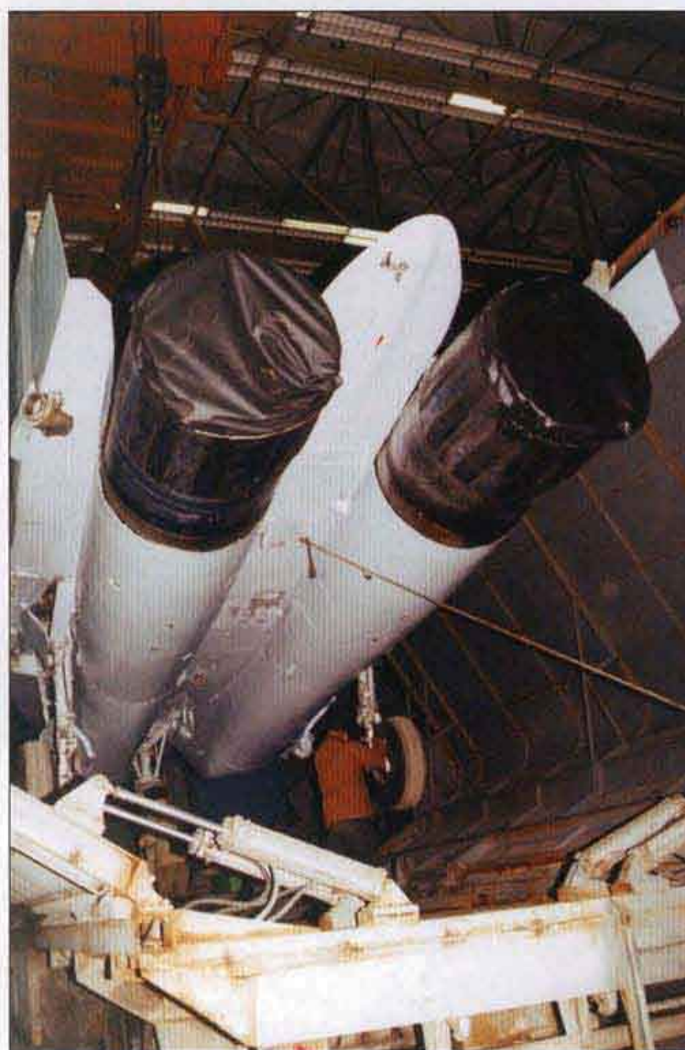
▲ MiG-29 Fulcrum-A '12 Blue' (c/n 2960520165) in the process of conversion to a MiG-29SMT at ANPK MiG's experimental shop in Moscow. Note the IFR probe.
