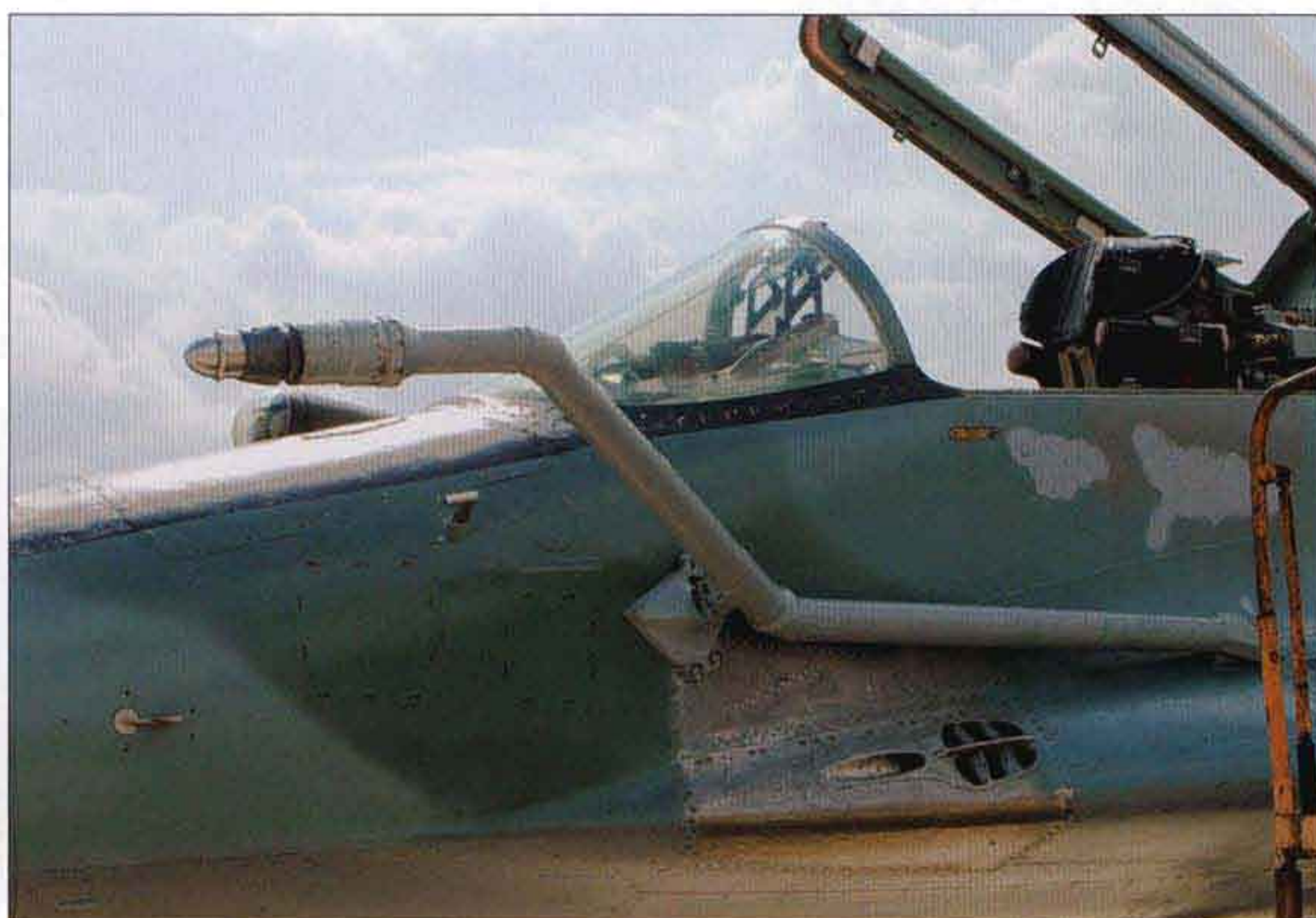
▲ Close-up of the MiG-29BM's IFR probe.
