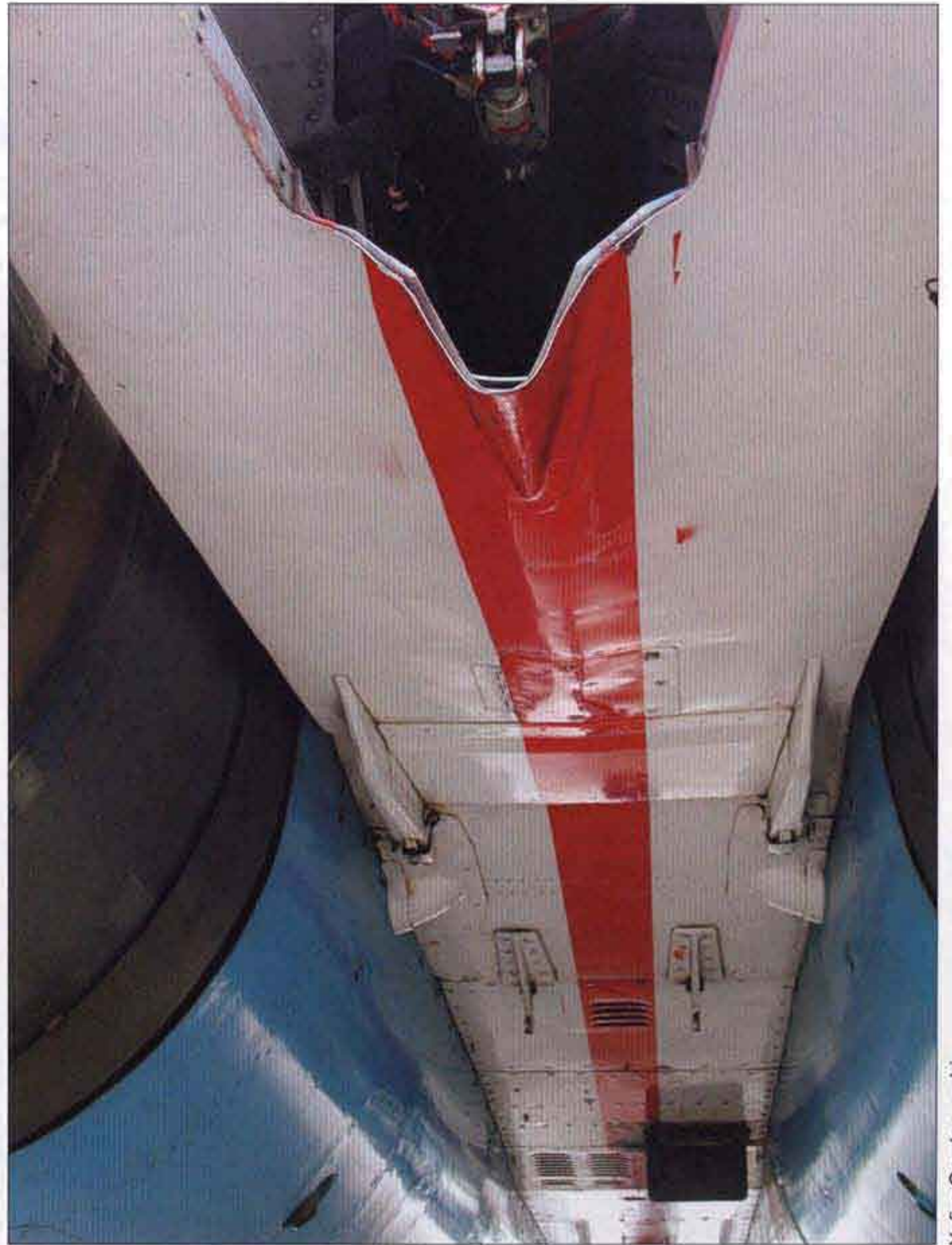
▶ The lower airbrake segment of a Fulcrum-C operated by the Ukrainian Falcons team. Note the APU exhaust door and the drop tank attachment fittings.
