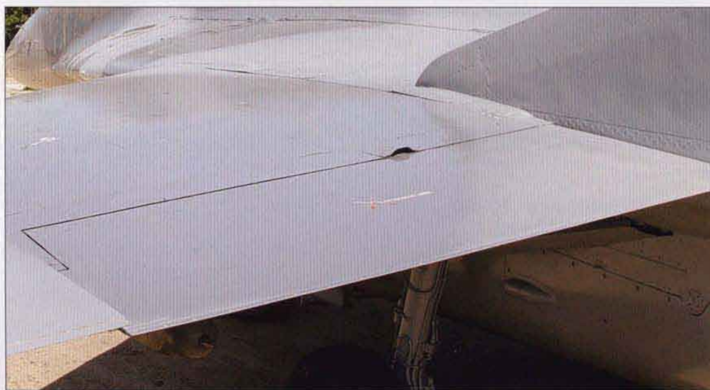
▲ ▲ ▲ ▲ The port leading-edge flaps of Fulcrum-Cs .
