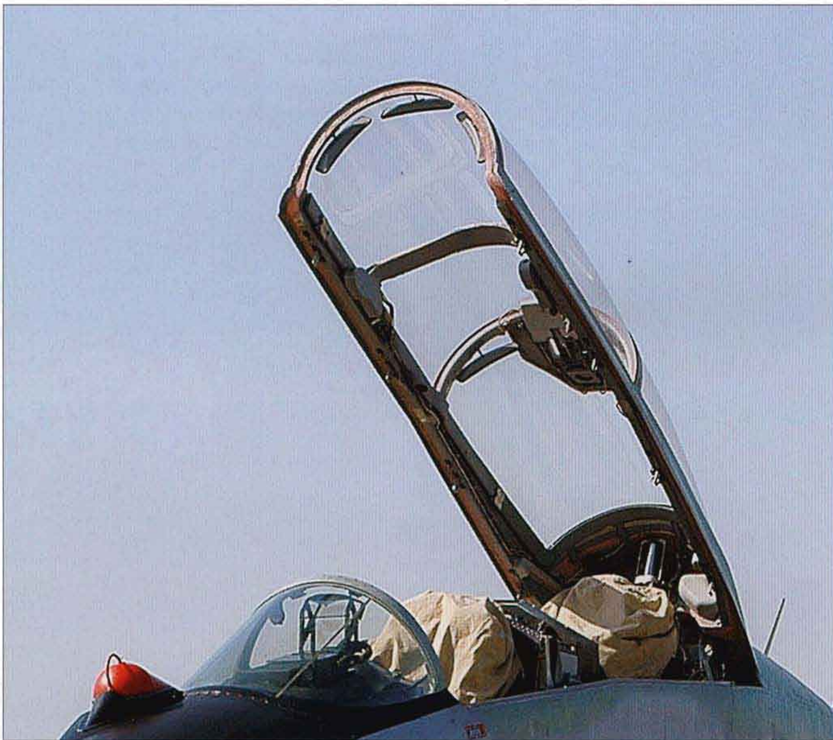
◀ The canopy of a MiG-29UB. Unlike single-seat versions, the canopy actuation pneumatic ram is exposed on the MiG-29UB. Note the folded blind flying hood over the front seat and the forward vision periscope built into the rear half of the transparency.
