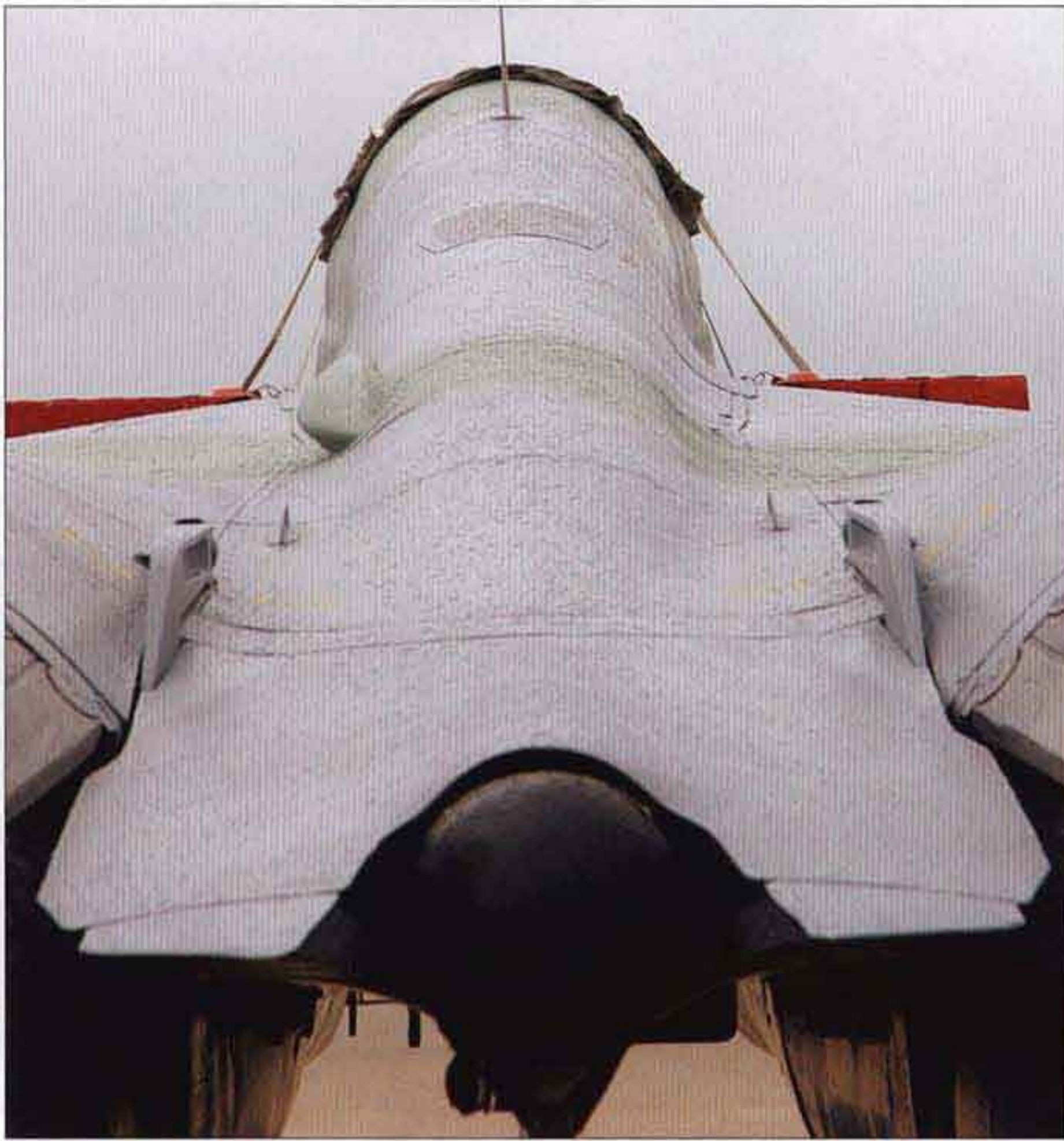
▲ The upper airbrake segment of a MiG-29 Fulcrum-A ; note the hefty external hinges.
