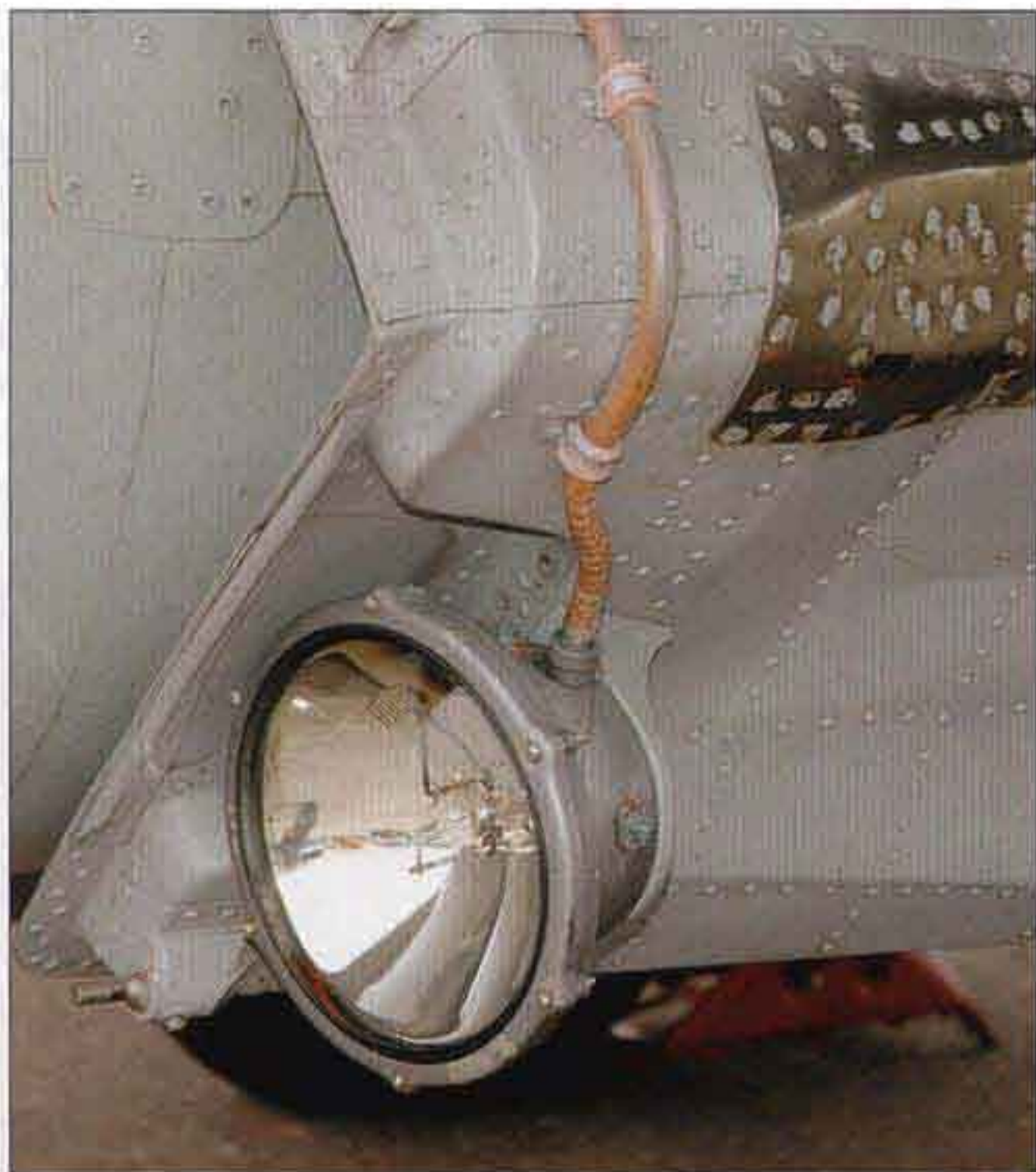
▲ The large mainwheel well doors carry the landing lights.
