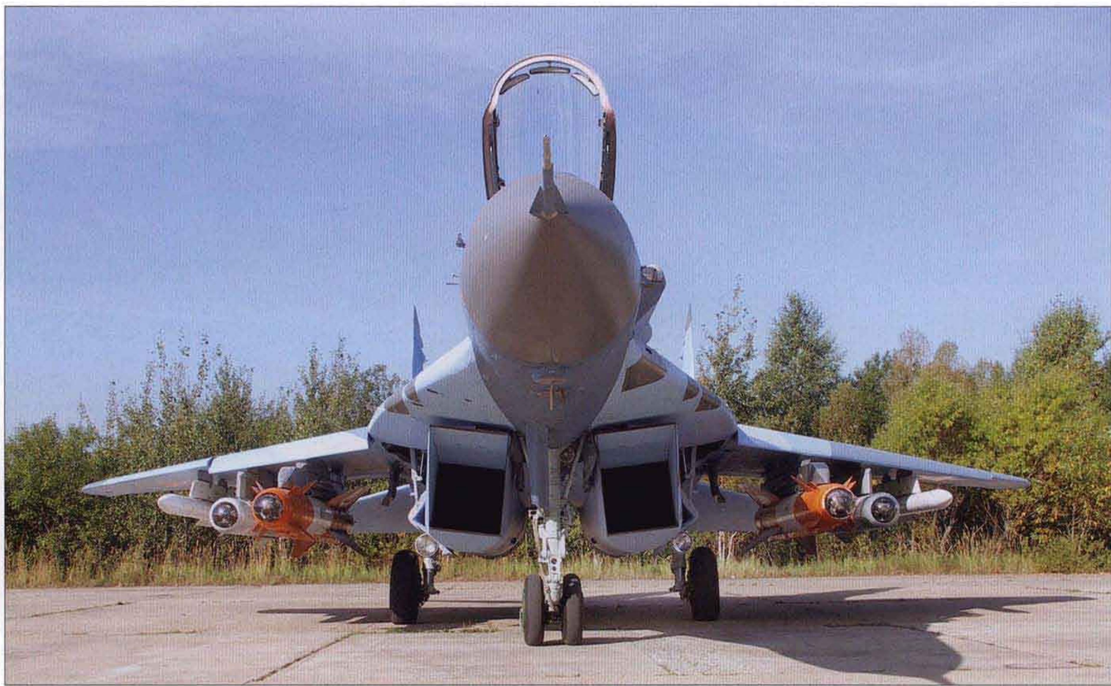
▲ Two views of MiG-29SMT '917 Blue' at RSK MiG's flight test facility. The aircraft is carrying two inert Kh-29T missiles on the inboard pylons, with KAB-500Kr guided bombs further outboard and dummy R-77s on the outermost pylons. ▼
