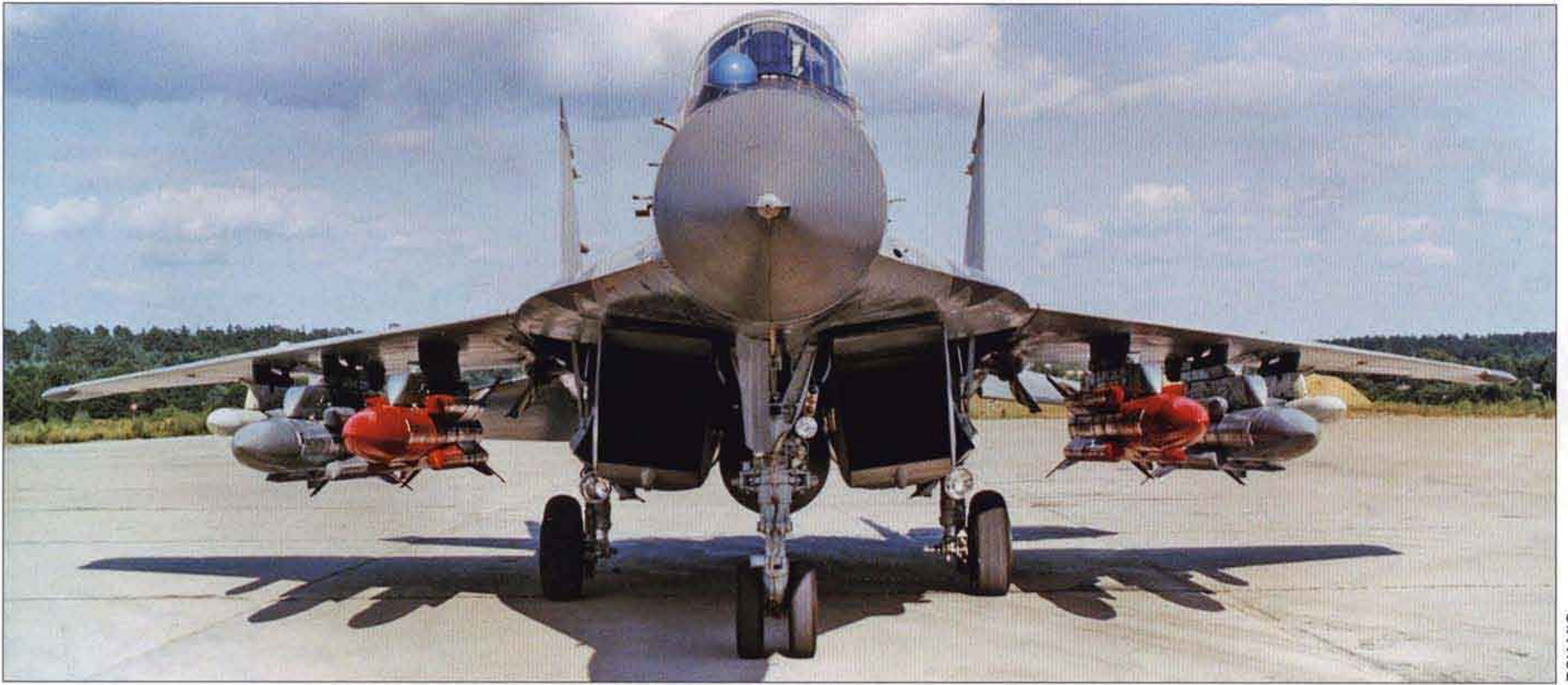
◀▲ The MiG-29K in anti-ship strike configuration with four Kh-31A ASMs on AKU-58 ejector racks under the inner wings. For MTOW reasons the defensive missile armament is limited to two R-77s under the outer wings. Note the drop tank in the upper and lower photos. ▼
