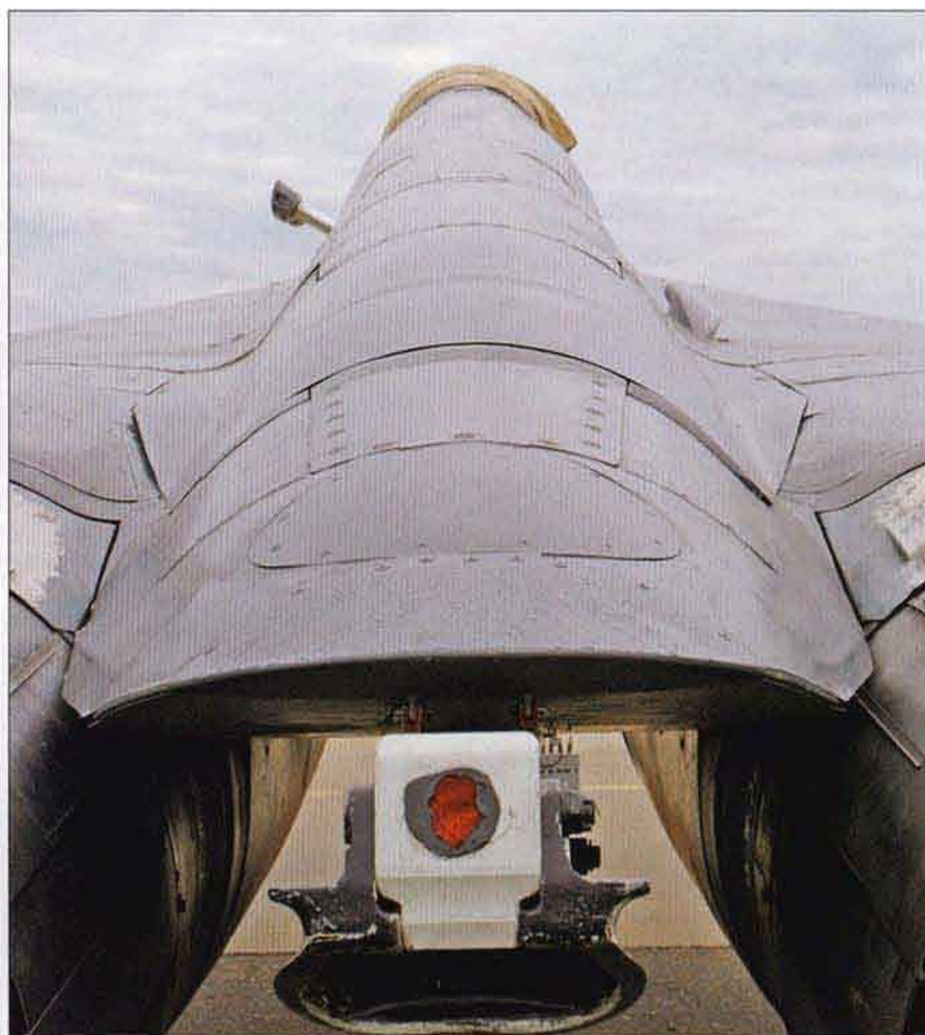
▲ The rear fuselage of a MiG-29K, showing the arrester hook.
