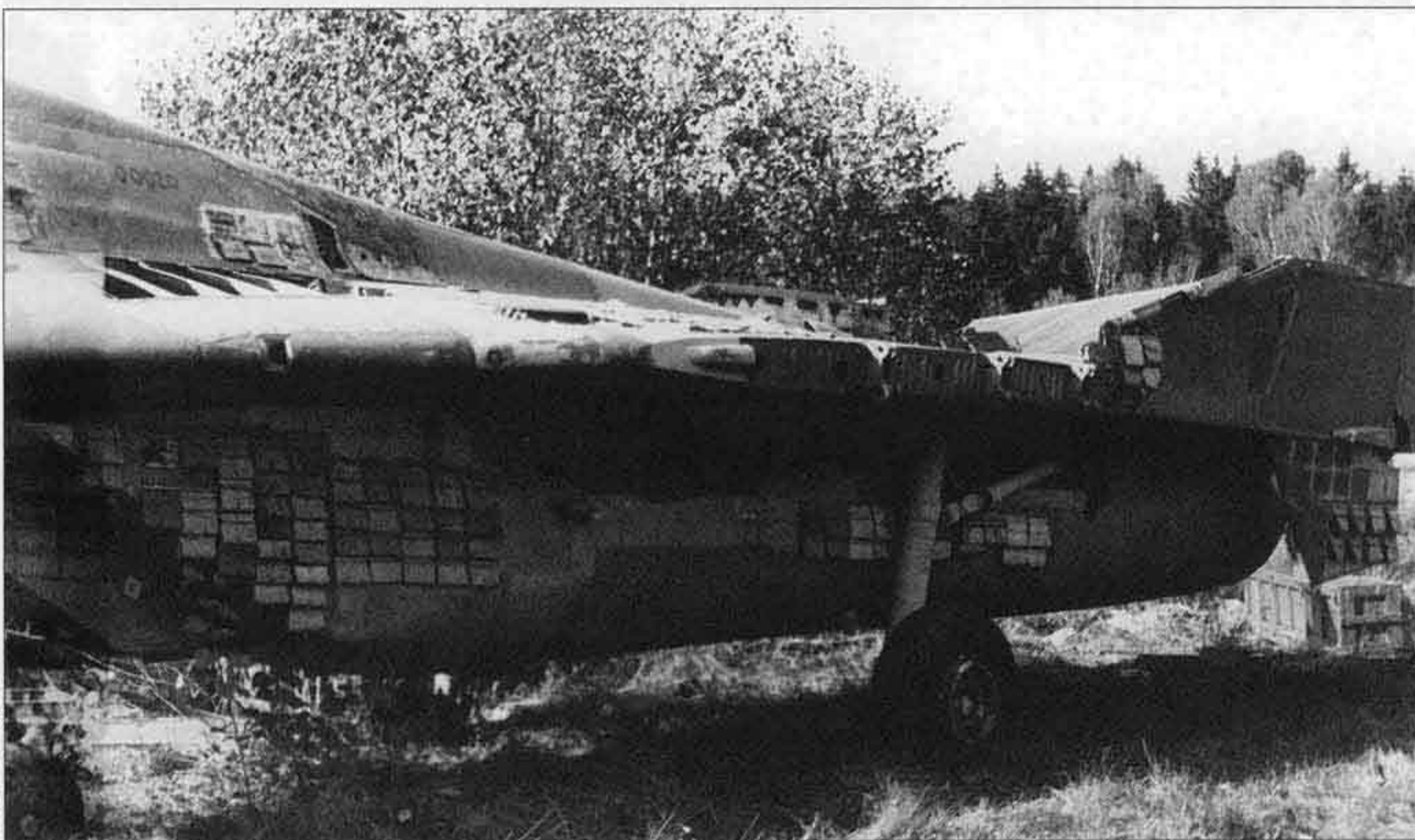
◀ Another view of the static test article. The wing root rib and the three outer wing attachment fittings are visible here. Note the number 00020 hand-painted on the fuselage which may be the aircraft's c/n.
