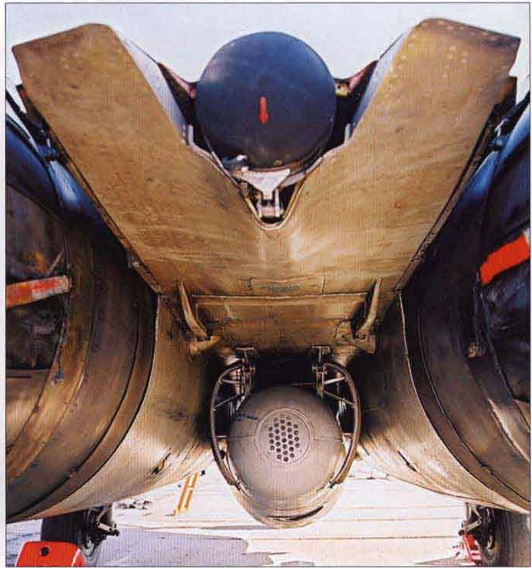
▲ The lower airbrake segment. Note the fixtures holding the rear end of the drop tank in place. The arrow on the brake parachute container points to the cover retention lock.
