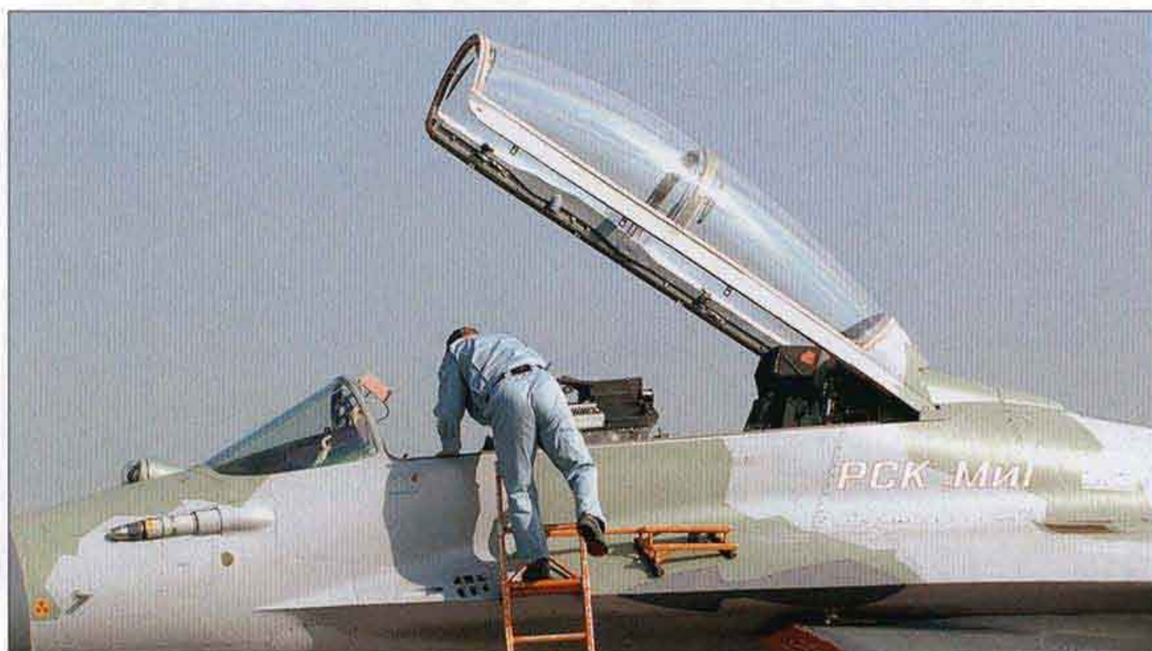
▲ Close-up of the MiG-29M2's forward fuselage, showing the fully retractable IFR probe. Note the custom-made boarding ladder with a side platform enabling the WSO to climb into the rear cockpit without slipping on the LERX.
