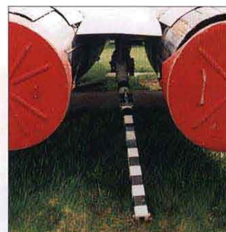
▲ The arrester hook of the MiG-29KVP. Note the absence of the usual airbrake and brake parachute.
