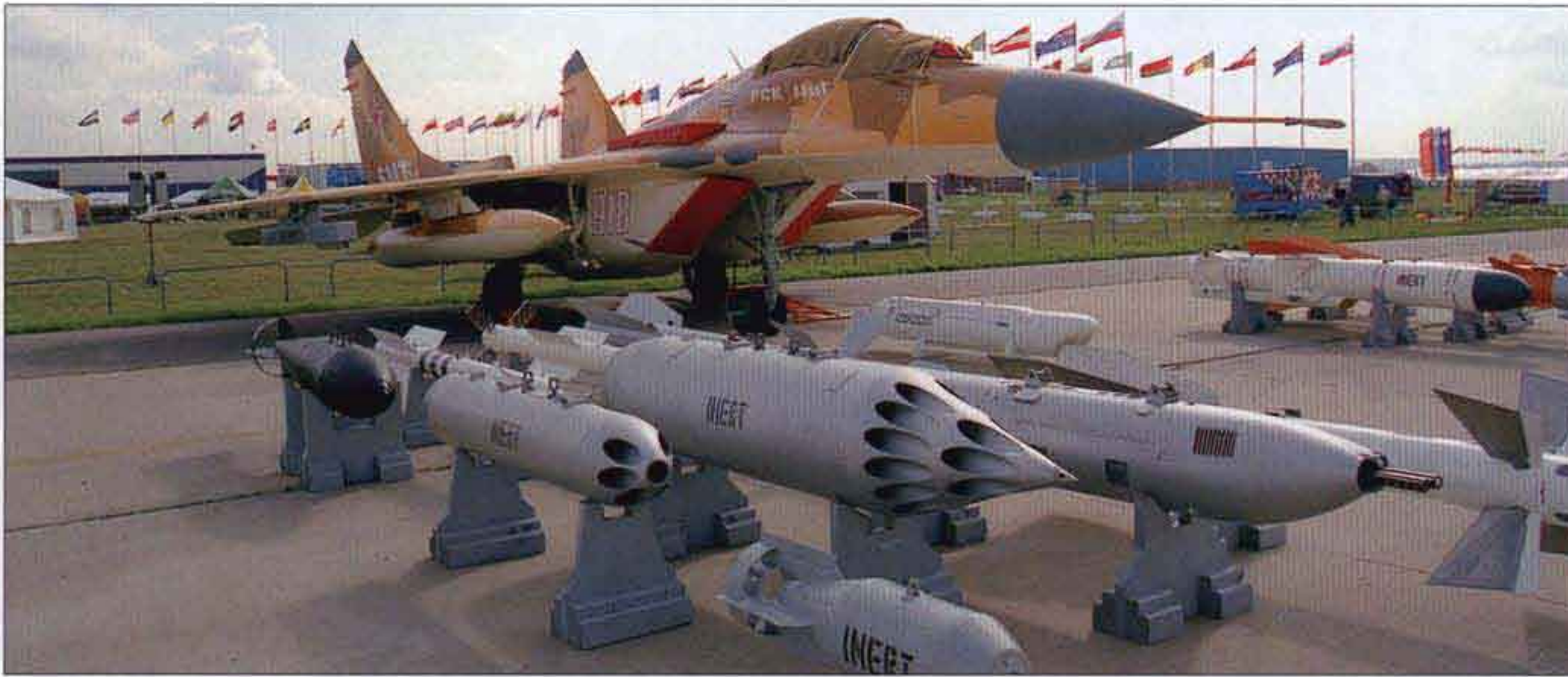
◀ Unguided air-to-ground weapons (an FAB-100M54 HE bomb, B-7L and B-8M1 FFAR pods, a UPK-23-250 cannon pod and an FAB-250M62 low-drag HE bomb) arrayed in front of MiG-29SMT '918 White'. Note also the Sapsan-E laser designator pod in front of the fighter.
