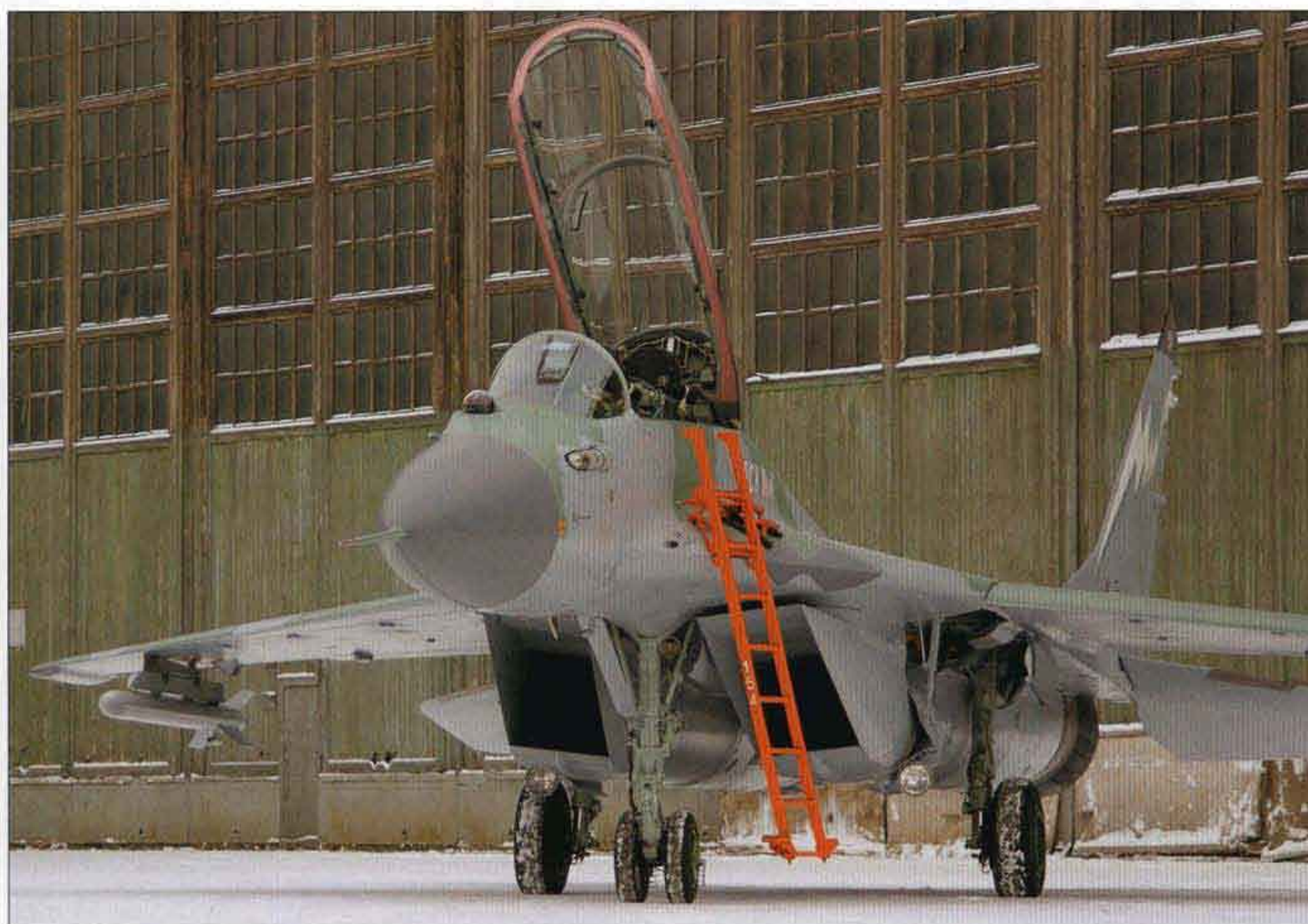
◀ The MiG-29M2 prototype ('154 White') sits in front of the Mikoyan hangar at Zhukovskiy with smoke generator pods (similar to the American 'Smokewinders') on the outermost wing hardpoints.
