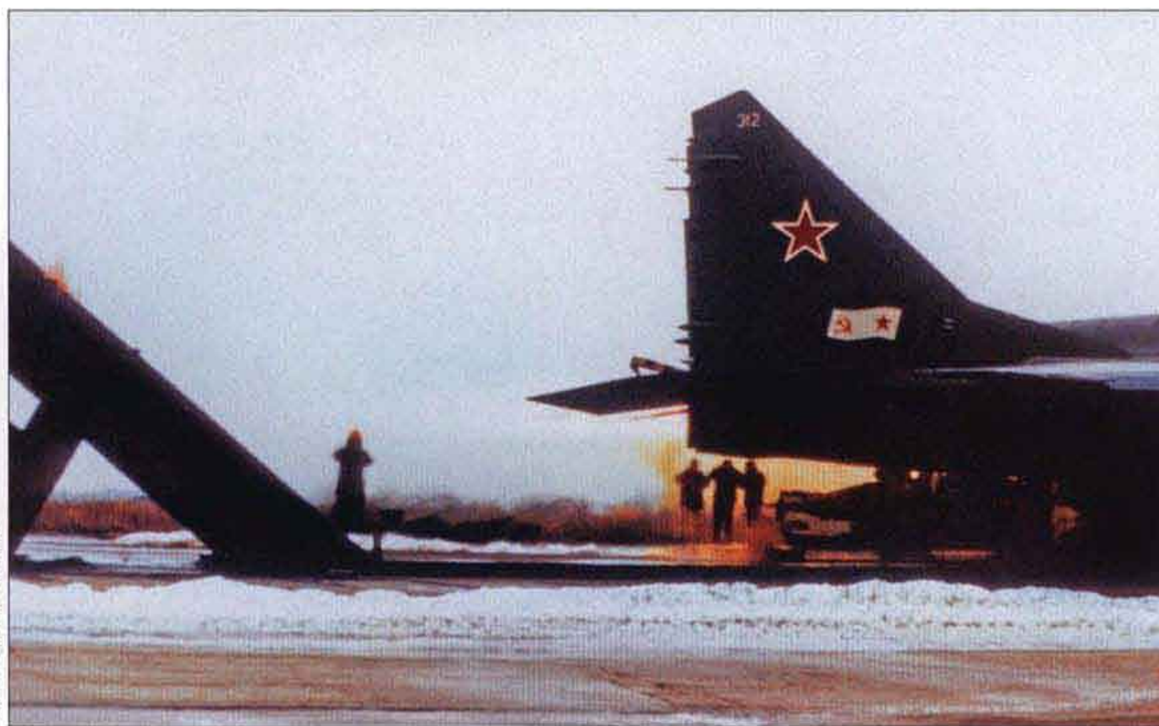
▲ The second prototype MiG-29K ('312 Blue') sits in front of the erected jet blast shield of the Nitka 'unsinkable carrier', the afterburners belching terrific flames.
