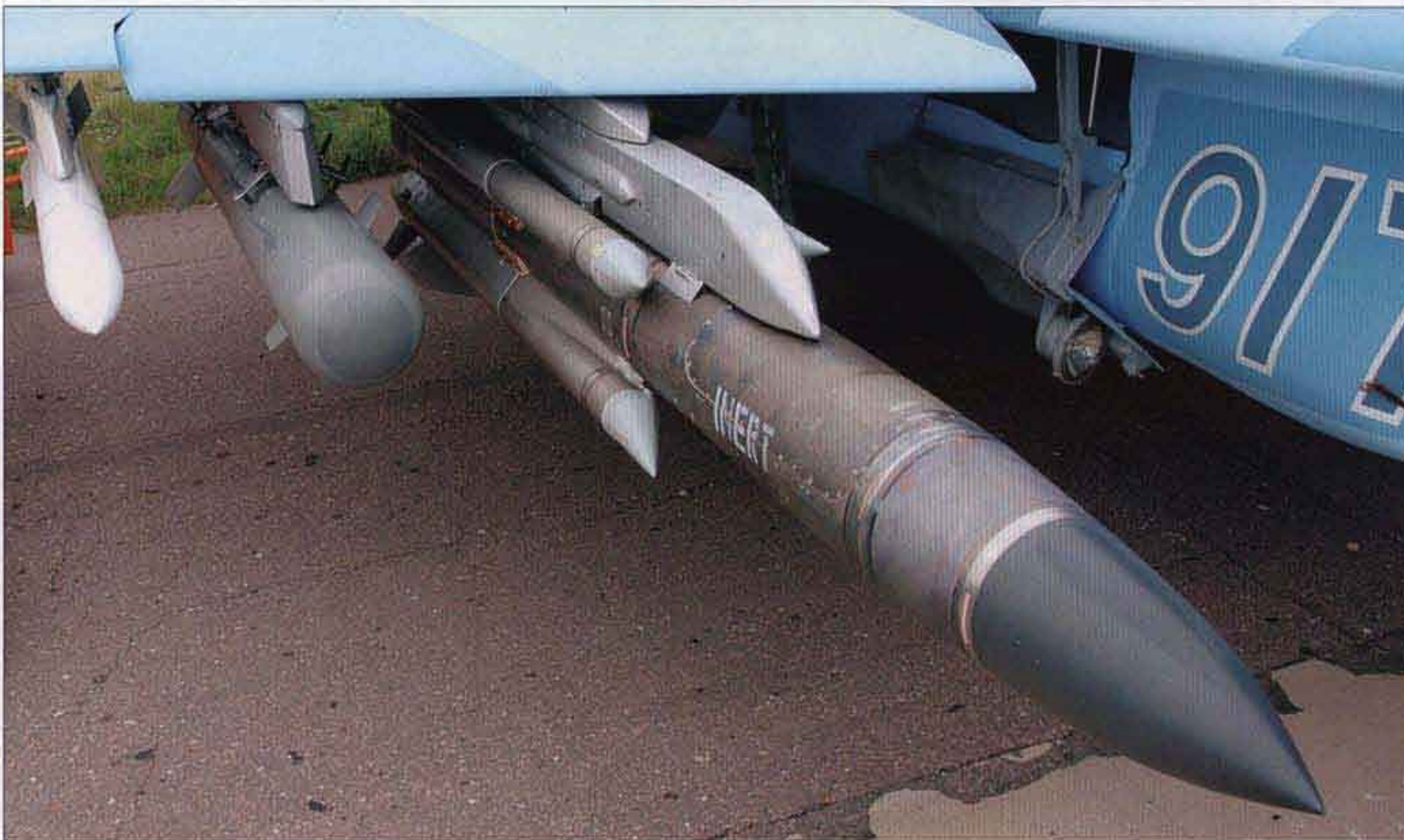
◀ An inert Kh-31P anti-radiation missile under the starboard wing of MiG-29SMT '917 Blue'.
