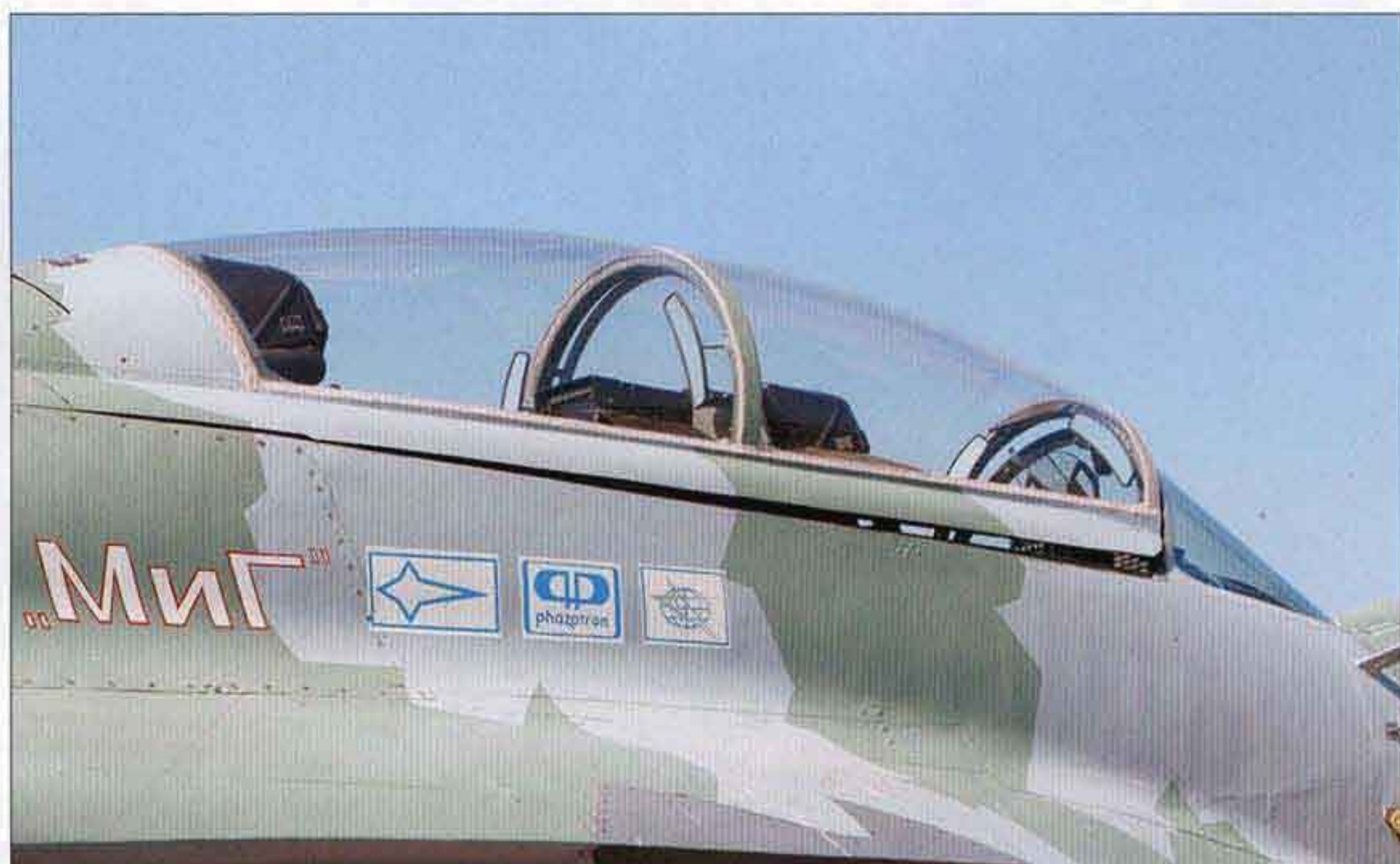
▼ The canopy of the MiG-29M2, while having the same shape as the MiG-29UB's, lacks the trainer's blind flying hood and periscope.
