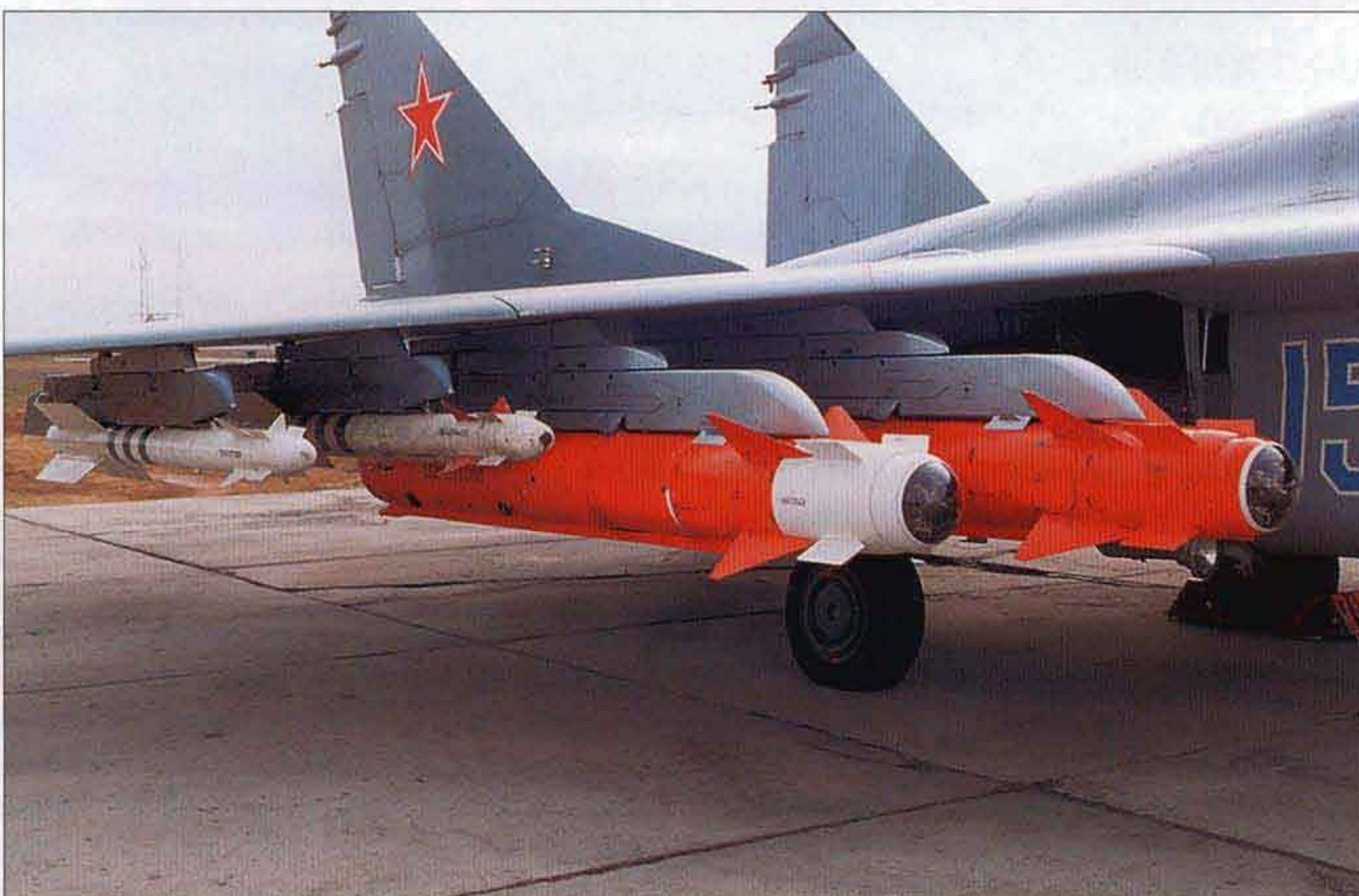
◀ Wingless Kh-29T missiles on the two inboard starboard pylons of MiG-29M '155 Blue'.
