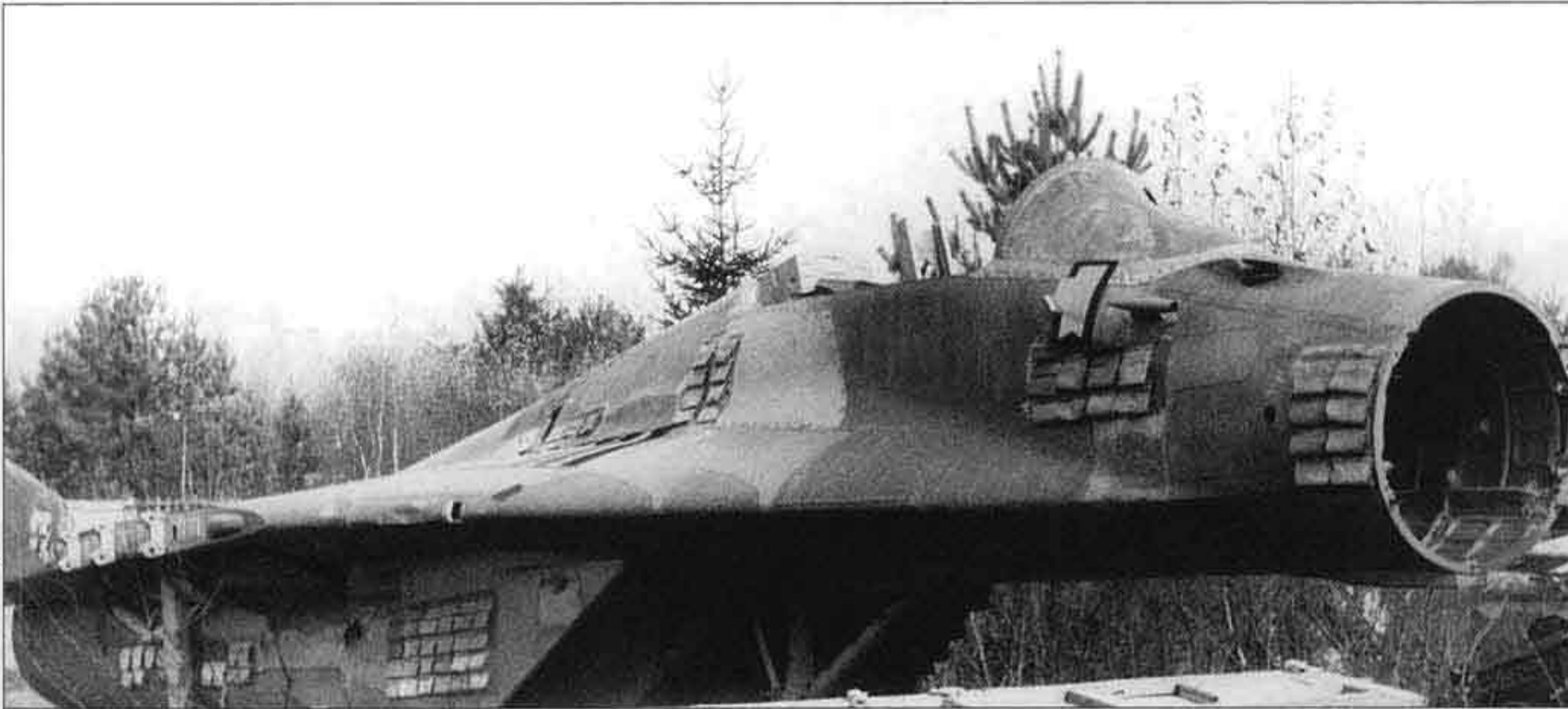
◀ A MiG-29 static test airframe dumped at the OKB's test facility in Zhukovskiy. The numerous rectangular objects on the fuselage sides are attachment points for the load application lines and strain gauges.
