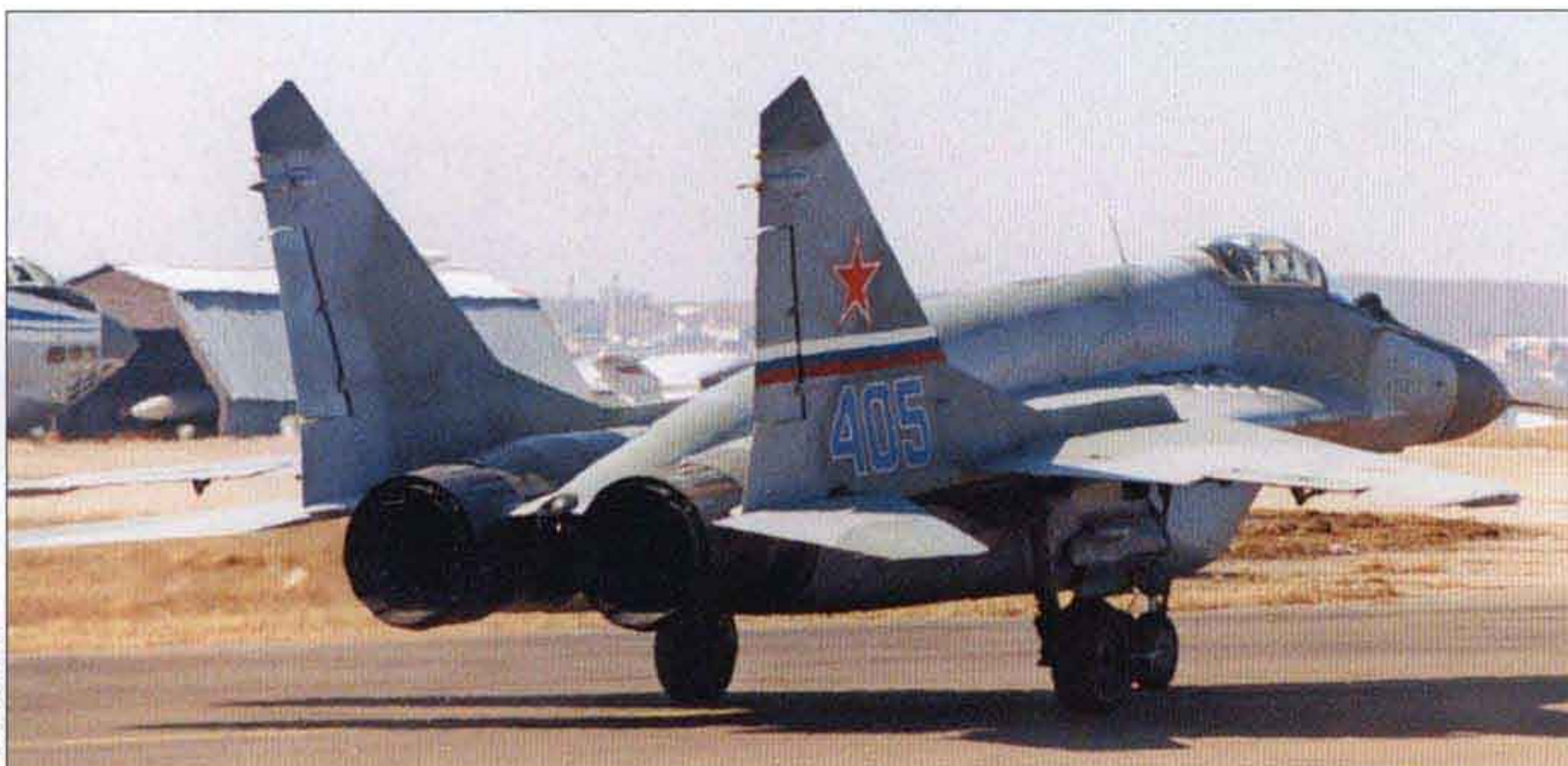
◀ This rear view shows that, despite the new fat spine, '405 Blue' retained the standard brake parachute container.
