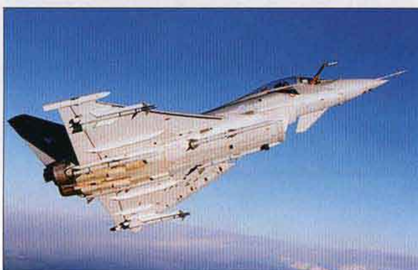
◀ Displaying its 'quadroundel' test markings in addition to the RAF insignia, one of the Eurofighter Typhoon prototypes is seen during a test flight with the IFR probe deployed. The type is in service with the UK, Germany, Italy and Spain.
