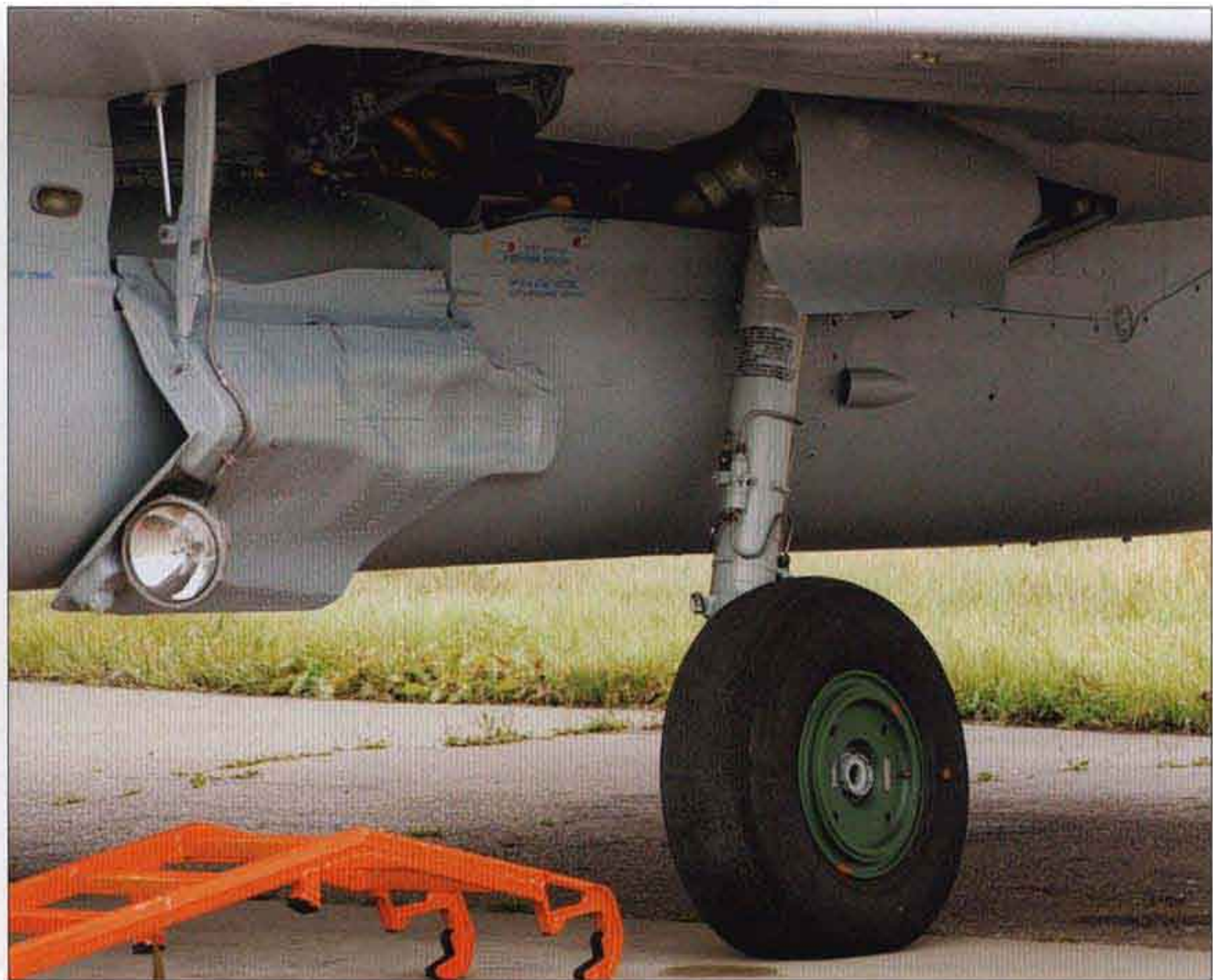
▲ The large mainwheel well doors carry the landing lights.
