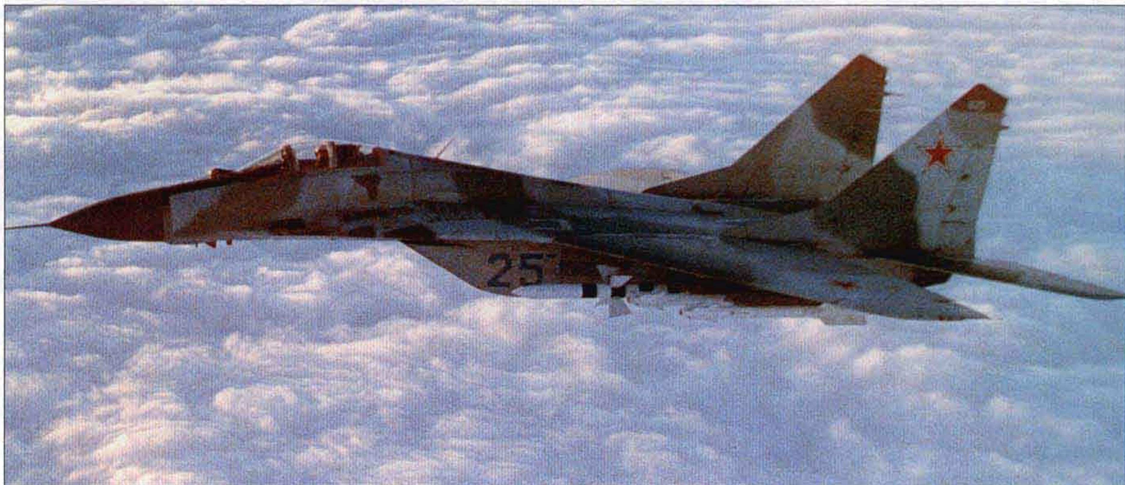
‘25 Blue/925’, the final MiG-29 prototype, in high-altitude flight with a load of dummy AAMs. ▼
