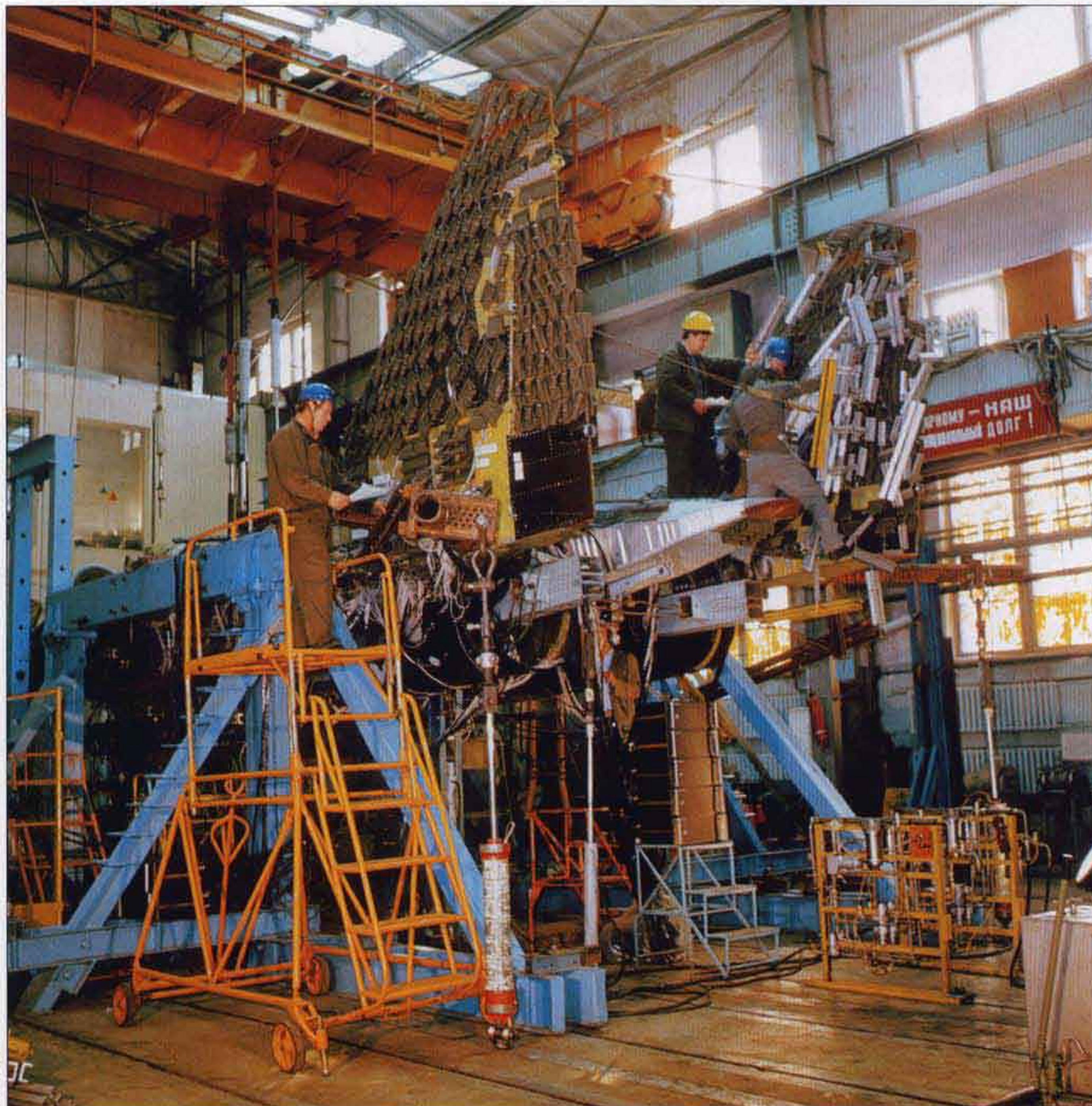
◀ A MiG-29M fuselage in the assembly jig at the Mikoyan OKB's experimental plant. The composite vertical tails have been fitted already.
