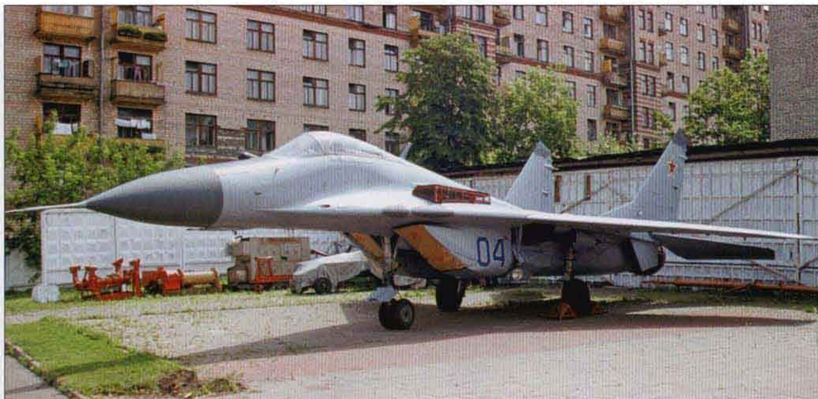
◀ 'Aircraft 904' was briefly displayed at an exhibition near Frunzenskaya tube station in Moscow in the late 1980s; thence it was relegated to the museum at Moscow-Khodynka. Note the angled nose gear door segment attached to the nose gear oleo, a distinctive feature of early-production MiG-29s.
