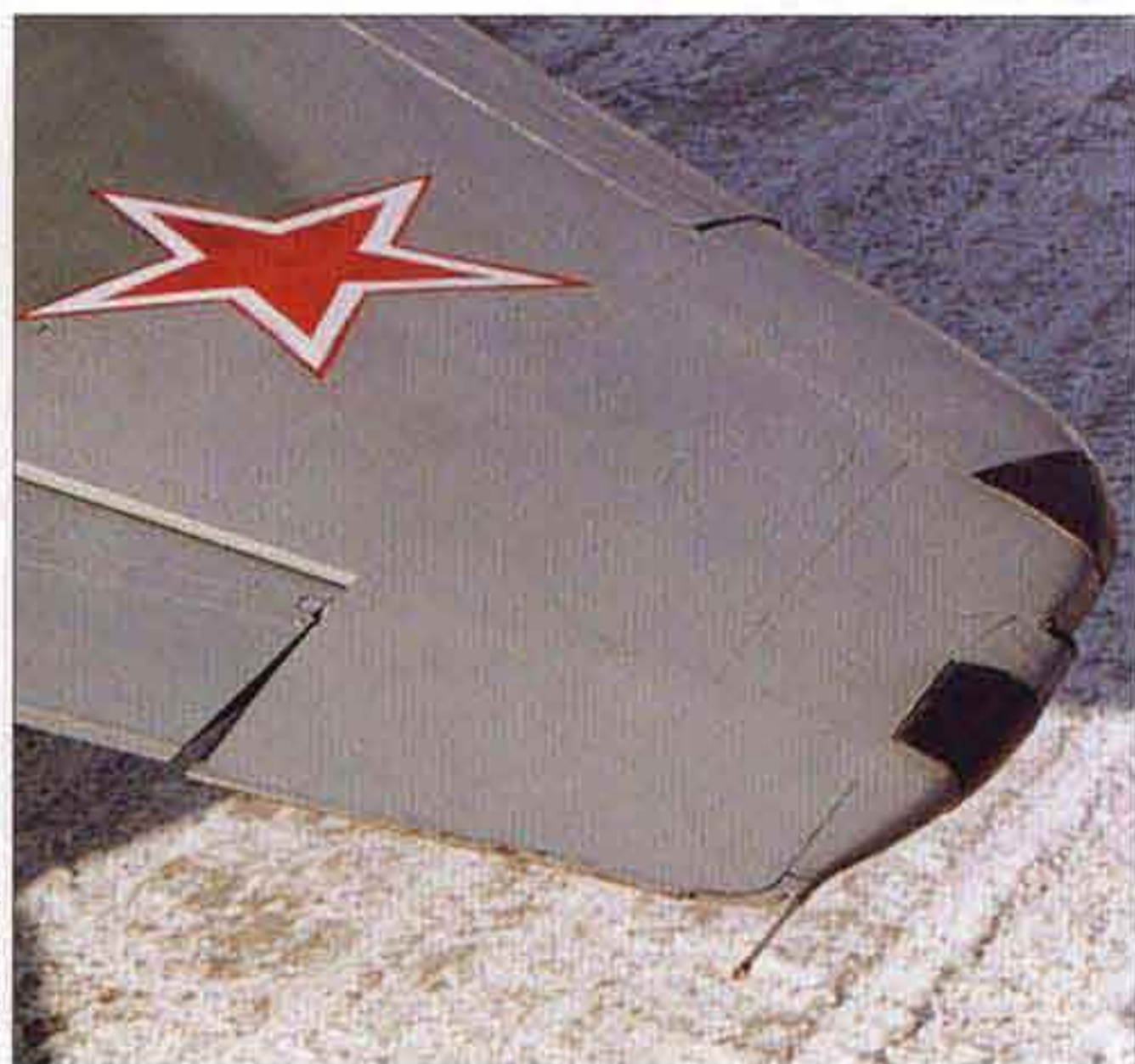
▲ The wingtips of the MiG-29 Fulcrum-C ( izdeliye 9.13 ) incorporate antennas for the Gardeniya-1FU (L-203B) self-protection active jammer and have a slightly different shape as compared to those of the Fulcrum-A and MiG-29UB.
