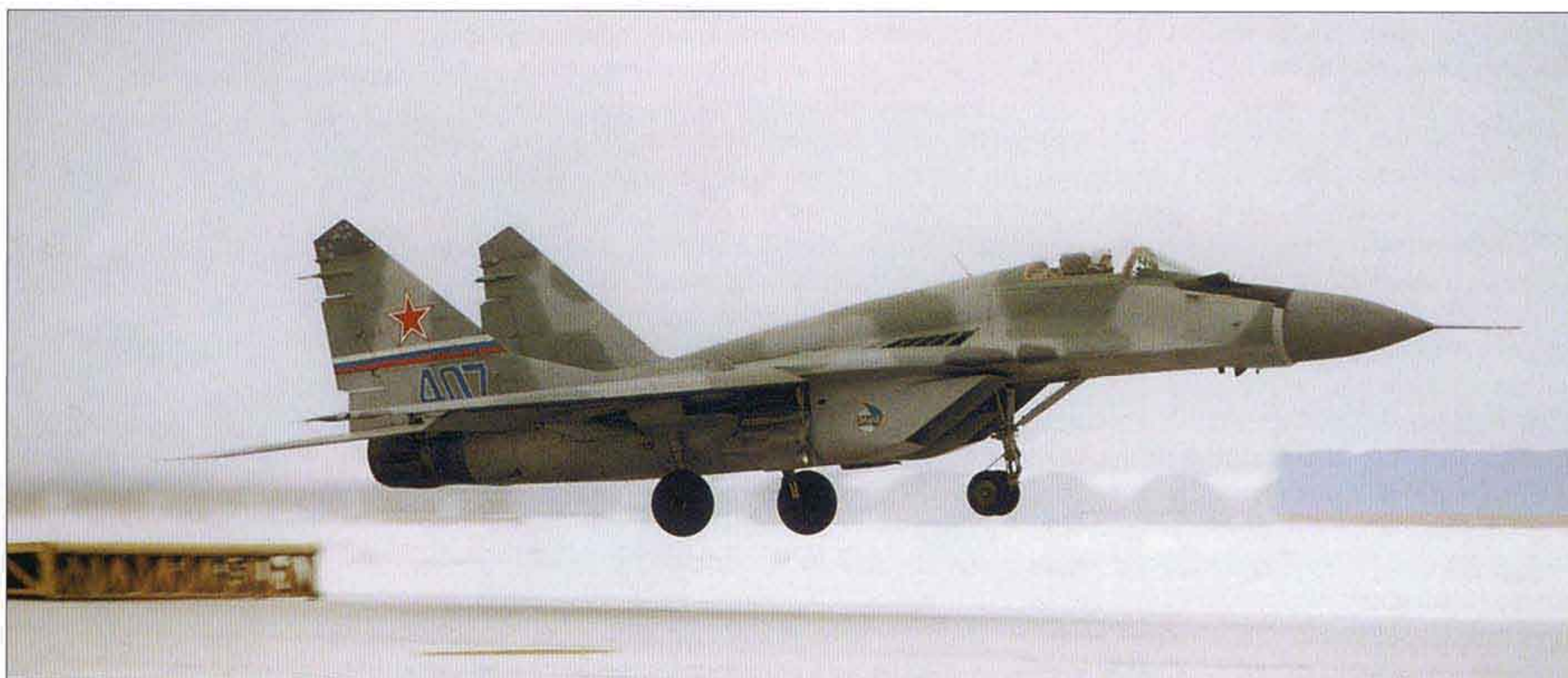
▼ The izdeliye 9.14 development aircraft (‘407 Blue’) takes off from the MT-1 mobile ski jump at Zhukovskiy in December 1997.
