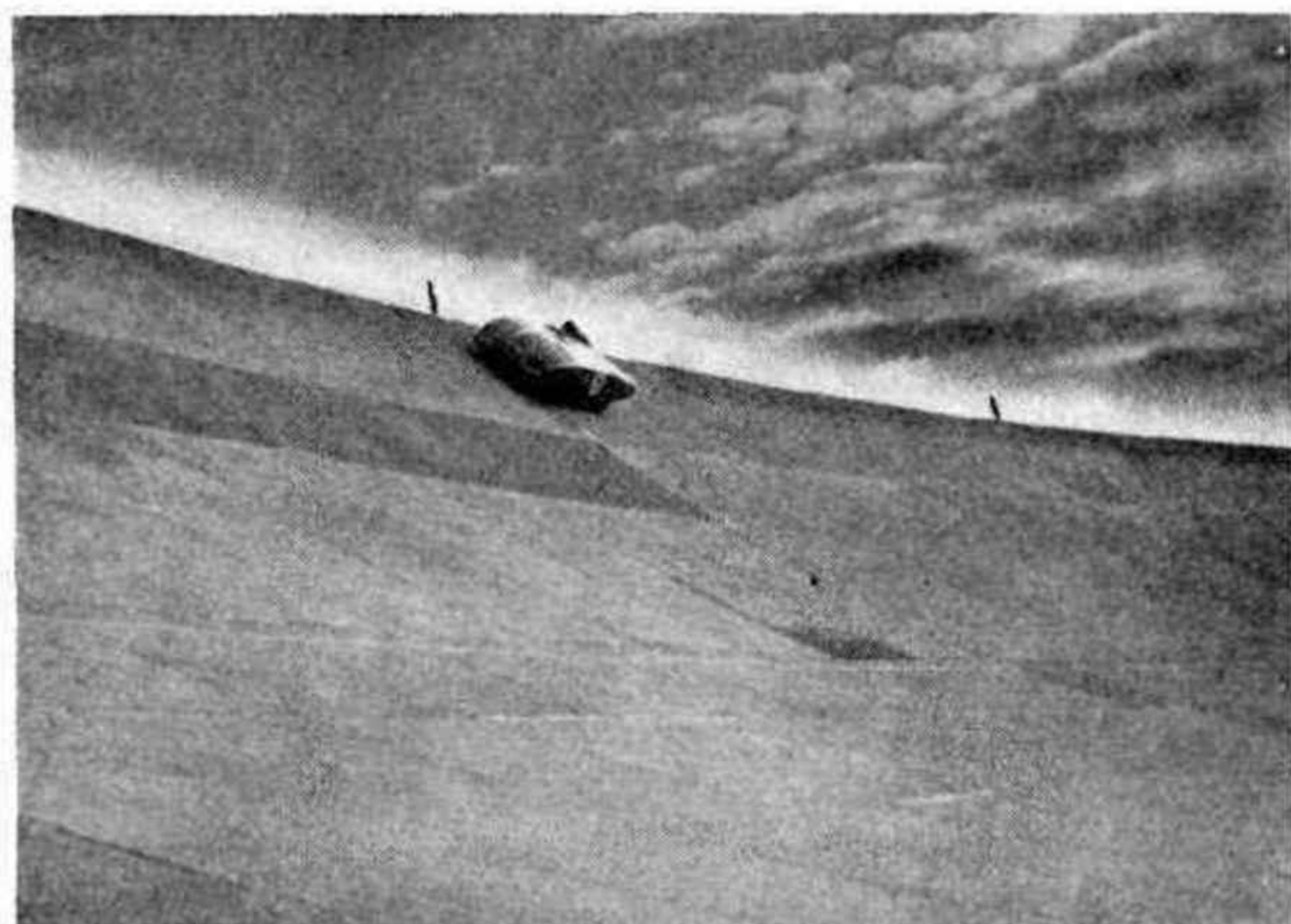
INCENTIVE TO A WIDE-OPEN THROTTLE. —At the top of the banking at Montlhéry last year, Chancel attacks Class H records from 50 km. to 250 miles in a Dyna-Panhard running at 5,700 r.p.m. and said to give 85 b.h.p. from its 610 c.c. flat-twin air-cooled engine—
