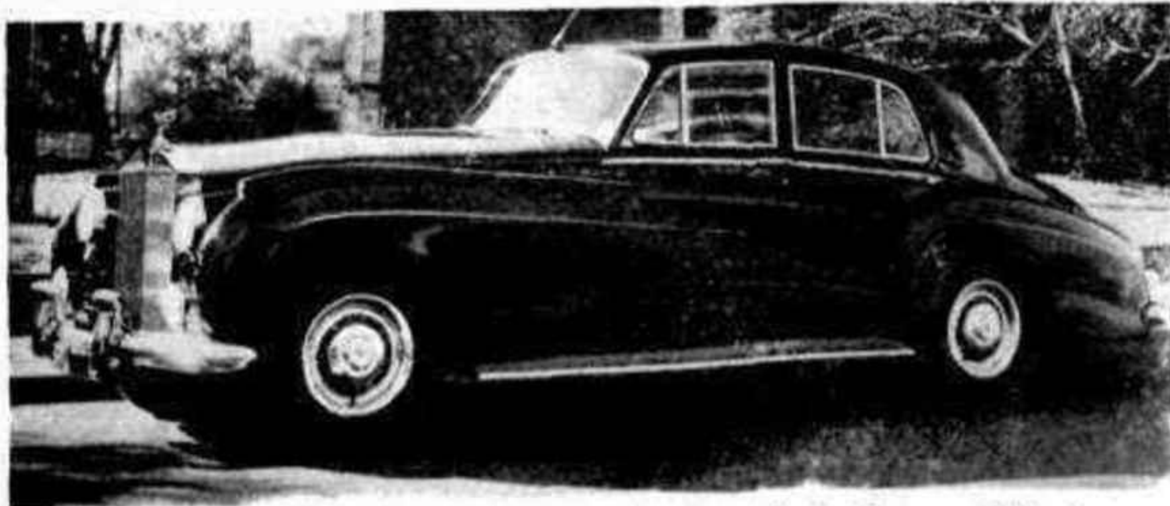
SILVER CLOUD is the type name of the new Rolls-Royce. The forward mounting of the radiator is retained and the engine is now of 4,887 c.c., like that of the new Bentley-S.
