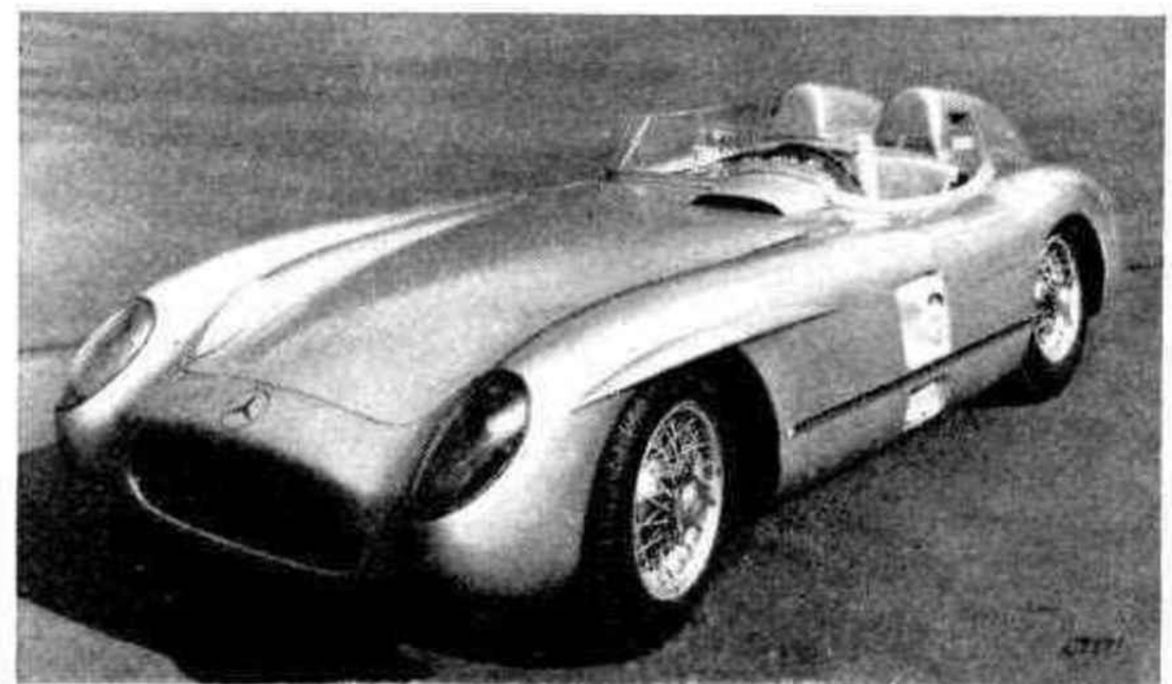
MERCEDES-BENZ 300SLR as it left the factory. Note the Perspex covers over lamps, air-intake on off side of bonnet, cockpit air-scoop in front of screen, dual headrests with fuel-filler in the driver's, under-bonnet outlets in front of door, three-eared hub-caps and negative camber of rear wheels.
