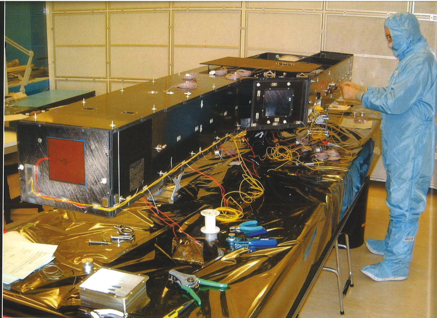
ABOVE AND RIGHT The Solar-B satellite, developed by Japan's Institute of Space and Astronautical Science, uses know-how from McLaren Composites to provide a bench for precision instruments
